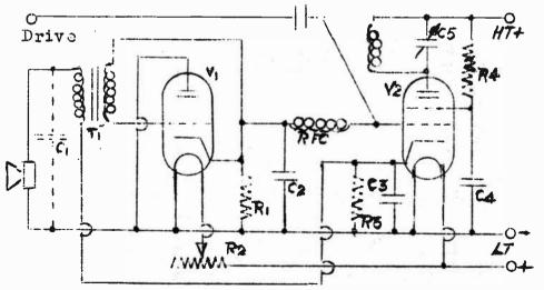
desired. The modulator takes ne current from the power supply. On application of drive to PA. 6J5 will conduct. It replaces PA grid\_ leak and the carbon mike in the modulator. grid circuit varies the 6J5 impedance. Best results were obtained with
