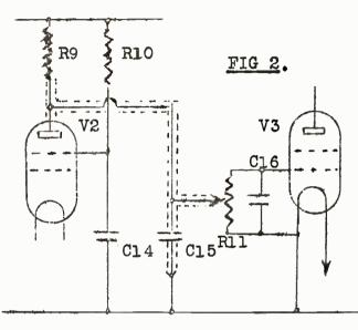
The additional audio unit shown in Fig 2, consists of the following extra components:-<u>R9</u>: .5 meg, <u>R10</u>: 2 meg. <u>R3</u>: 1 meg. <u>C14</u>: 8 uF elect. <u>C15</u>: 1500 pF mica. <u>C16</u>: 50 pF mica. <u>V3</u>: 1LN5.
