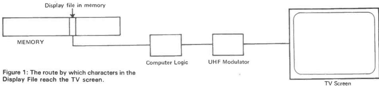
Figure 1: The route by which characters in the Display File reach the TV screen.
