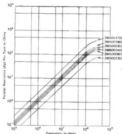
Figure 10: Parallel reactance per turn Vs frequency for Fair-Rite 65 material.
