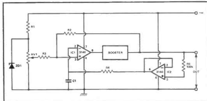
Figure 11: Offset biasing via an op-amp buffer.
