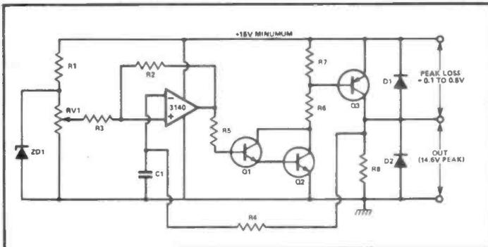
Figure 7: SMVF circuit with high-efficiency power-boosting via a pair of common emitter amplifiers.
