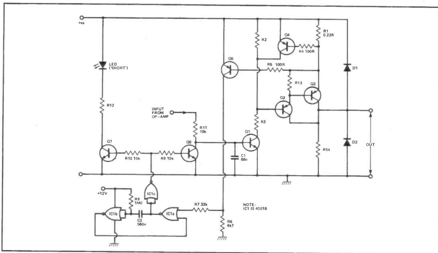
Figure 18: The load current of this circuit limits to 3 Amps peak under normal driving conditions, but falls to about 3mA when a short occurs.
