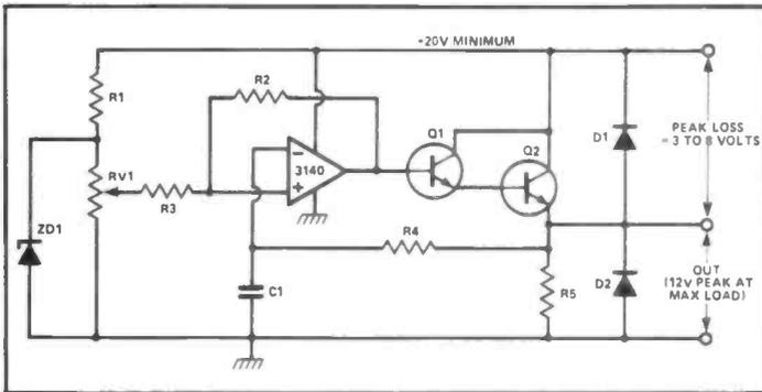
Figure 6: SMVF circuit with power boosting via a Darlington emitter follower.
