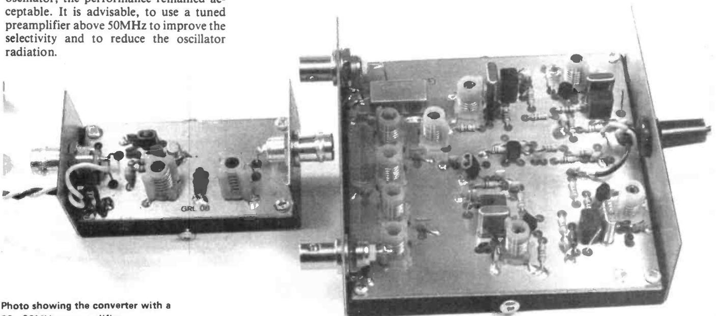
Photo showing the converter with a 28 - 30MHz pre-amplifier.
