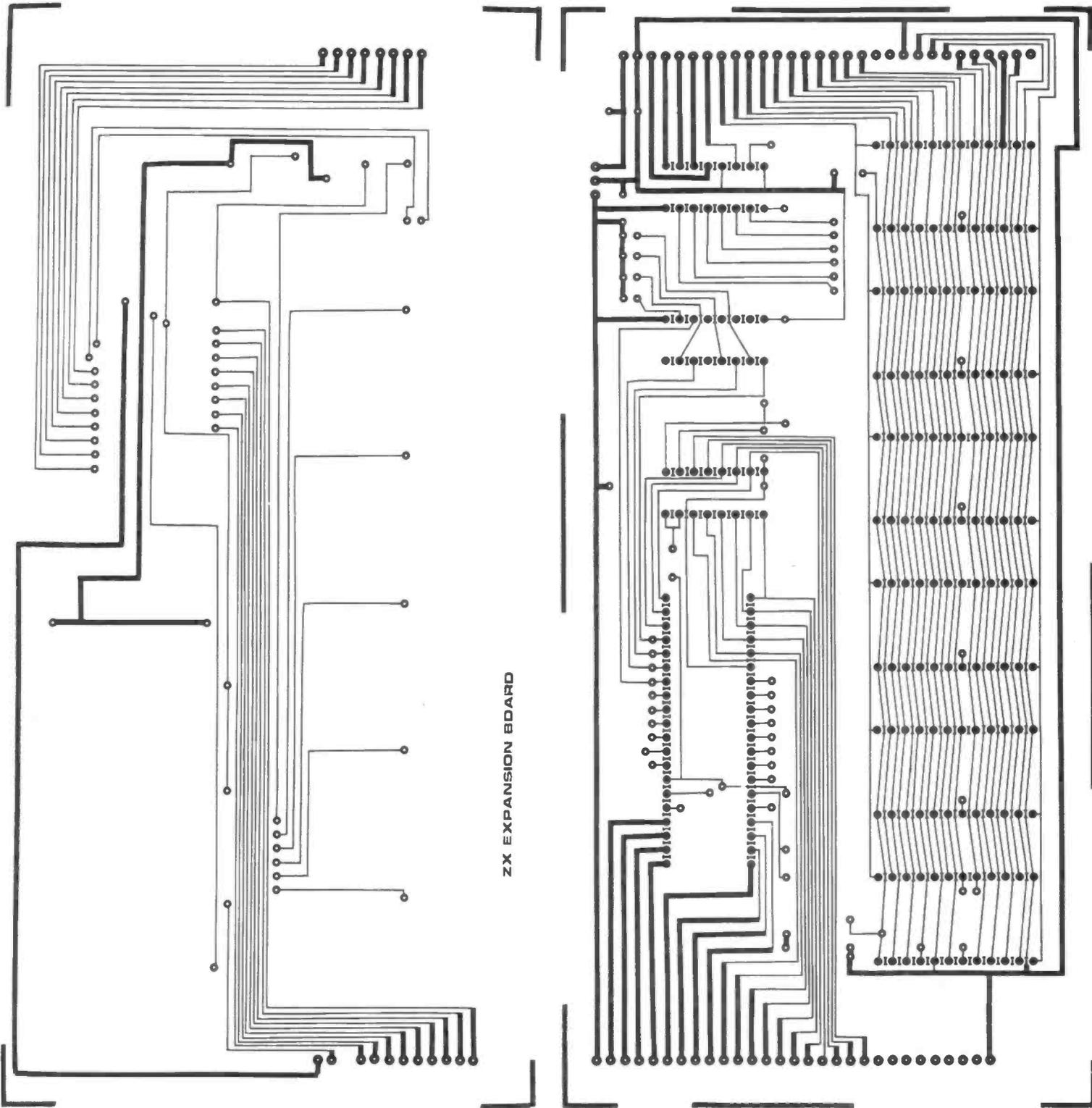
PCB foils of top and bottom track of ZX81 expansion board.
