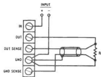
Figure 5: Remote Sensing Connections.
