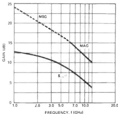
Figure 1a: Typical gain vs. frequency for the NE72089 at  $V_{DS} = 4V$  and  $I_{DS} = 30mA$ .
