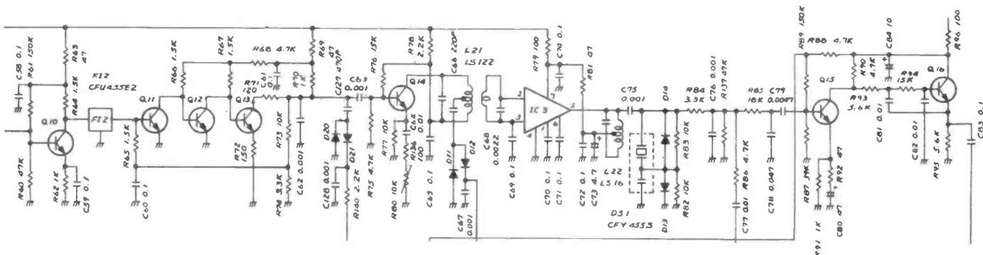
Figure 1: The final IF stages of the IC25 employ a combination of bipolar limiting amplifiers and a ratio detector using a ceramic element and diode arrangement.
