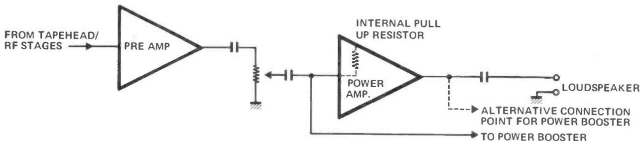
Figure 1. The power booster is turned on by a DC voltage superimposed on its audio input signal. The feed to the 'Booster' should either be taken from the existing amp's output - before DC blocking capacitor, or for better quality sound from the power Amp's input pin. See table 1 for connection details for some popular power amp ICs.
