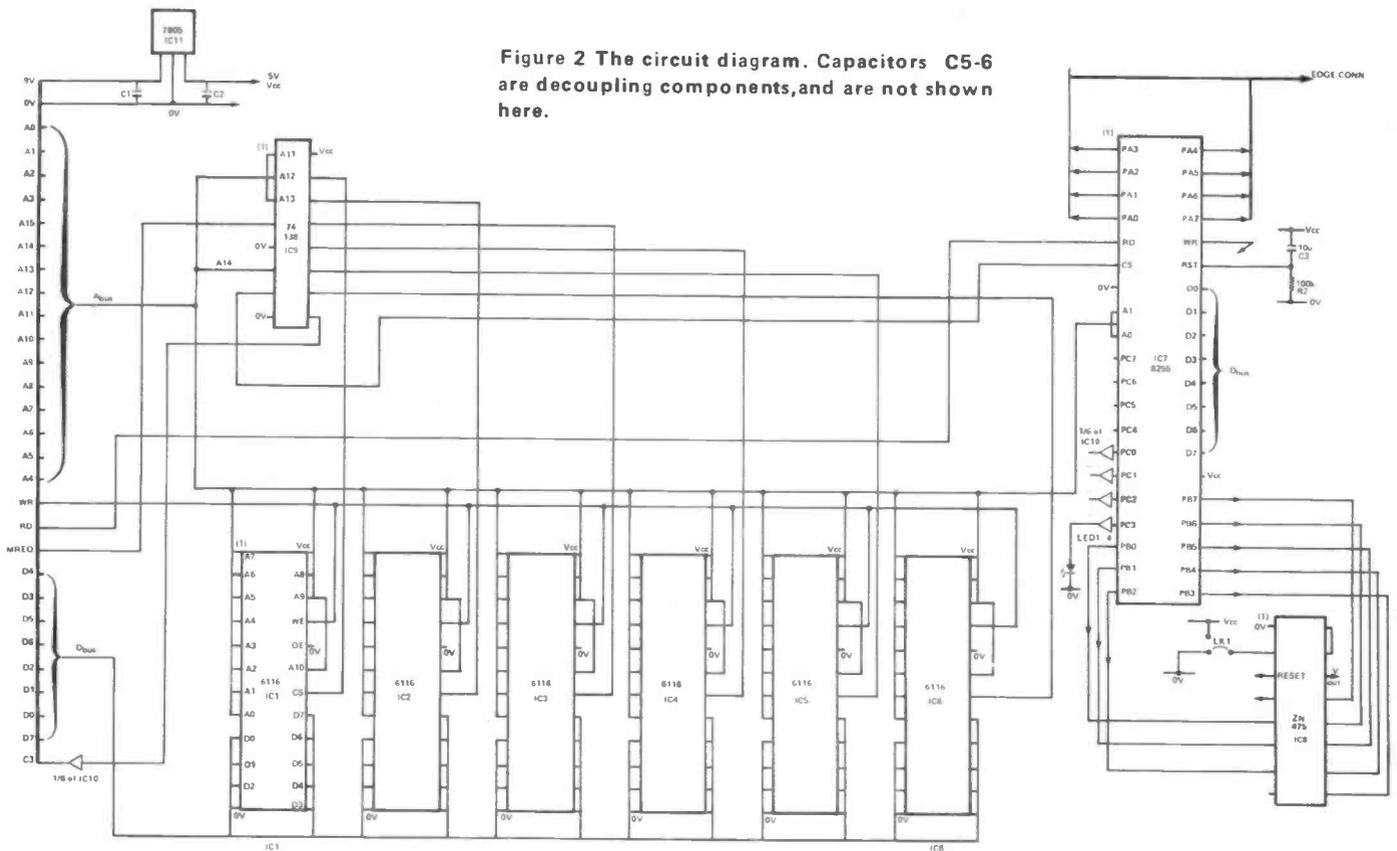
Figure 2 The circuit diagram. Capacitors C5-6 are decoupling components, and are not shown here.
