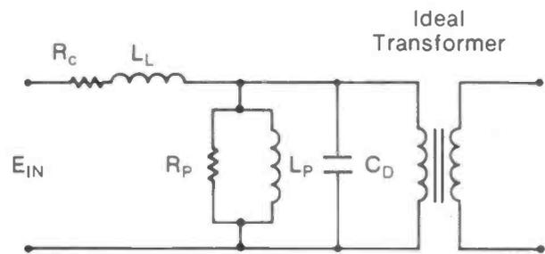
Figure 2: Transformer lumped element equivalent circuit.
