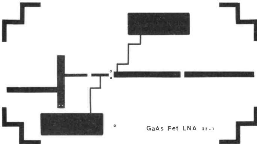
Figure 7: Pre-amplifier PCB Foil Pattern.
