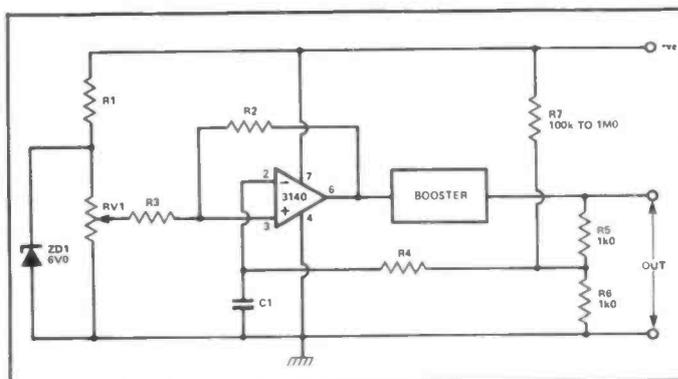
Figure 12: Offset biasing via potential divider.
