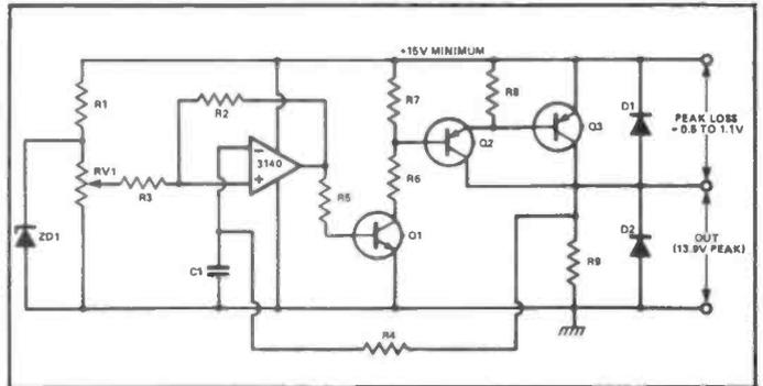
Figure 8: SMVF circuit with slightly less efficient power-boosting via a pair of common emitter amplifiers.
