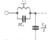
m - derived end sections for use with intermediate pi section
