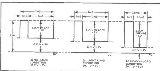
Figure 5: A SMVF-controlled Dc motor has excellent regulation (equal to that of a DC-controlled system) and superb speed control (far better than that of a fixed-frame system).
