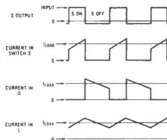
Figure 7: Waveforms associated with a step-down switching regulator design.
