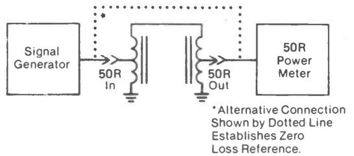
Figure 6: "Back-to-back" transmission loss test set-up.
