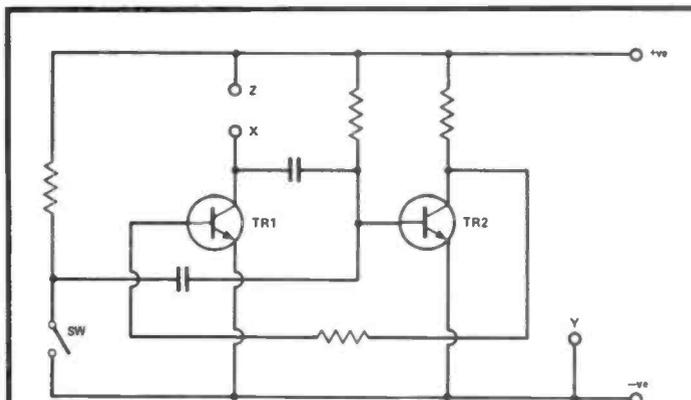
Figure 2: The basic-building block of the speed indicator circuit is a monostable multivibrator.
