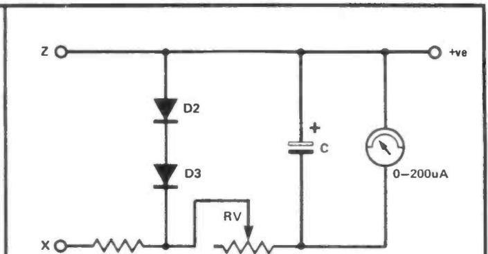
Figure 3: The constant duration pulses from the multivibrator are integrated by this circuit.
