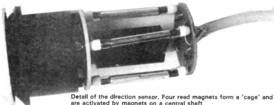
Detail of the direction sensor. Four reed magnets form a 'cage' and are activated by magnets on a central shaft
