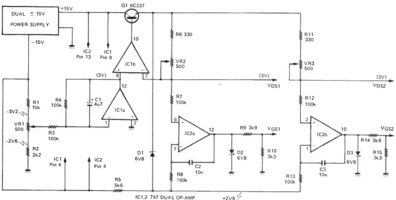
Figure 3: Power Supply Circuit Diagram.
