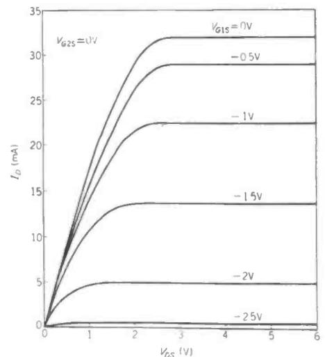
Figure 3: Typical DC characteristics of Ga As Fet.
