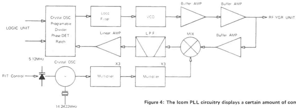
Figure 4: The Icom PLL circuitry displays a certain amount of complexity.
