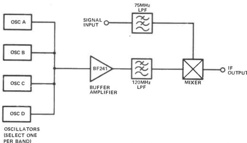
Figure 3: Converter Block Diagram.
