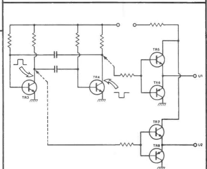
Figure 5: The circuit to produce the AC drive to the direction indicator circuit is an astable multivibrator.
