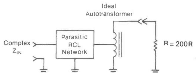
Figure 4: Simplified equivalent circuit of practical 1:4 autotransformer. ►
