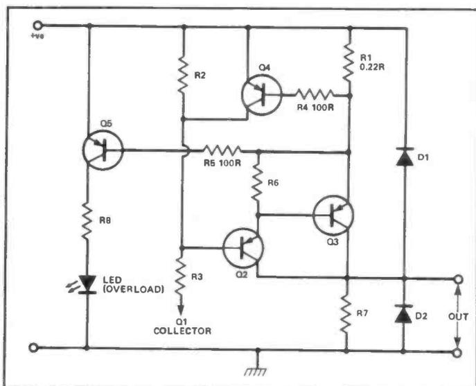
Figure 16: 3 amp output-current limiter with LED Indicator.
