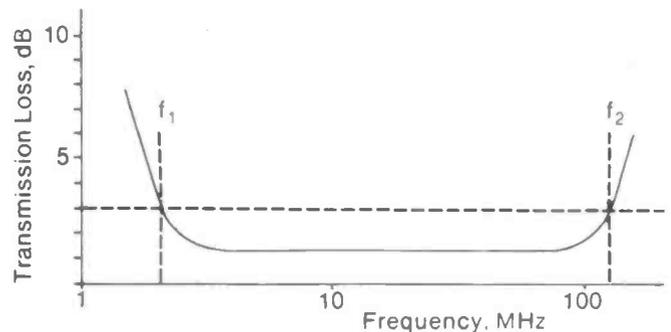
Figure 1: Typical transformer transmission loss vs. frequency.
