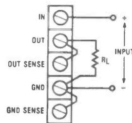
Figure 2: Board Connections for 'Normal Mode' Operation.
