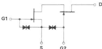
Figure 2: Equivalent circuit of a typical dual gate MESFET (3SK112).
