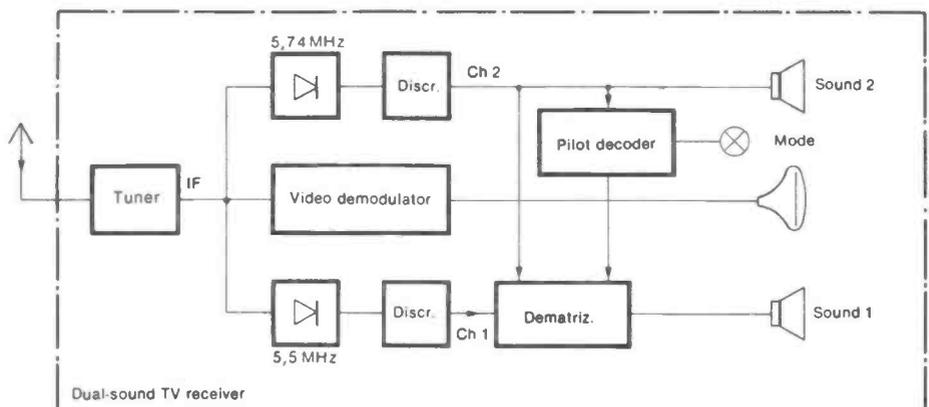
Block diagram of a typical stereo TV receiver using the dual carrier approach adopted in Germany.
