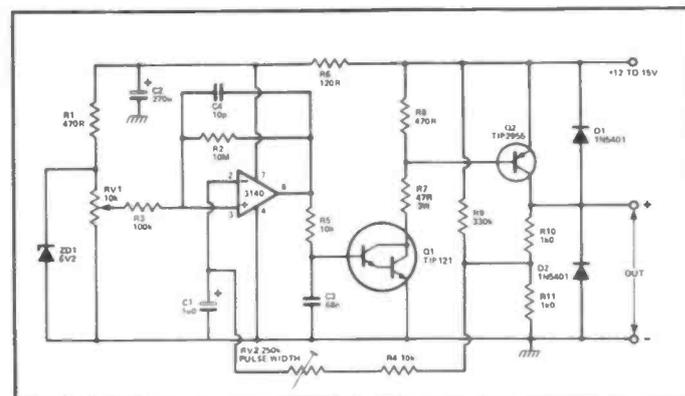
Figure 13: High-efficiency battery-powered SMVF circuit, for use in cars.
