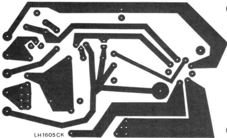
Figure 3: PCB Foil Pattern. Only one side shown, PCB available from R&EW Project Pack Service — See page 58.
