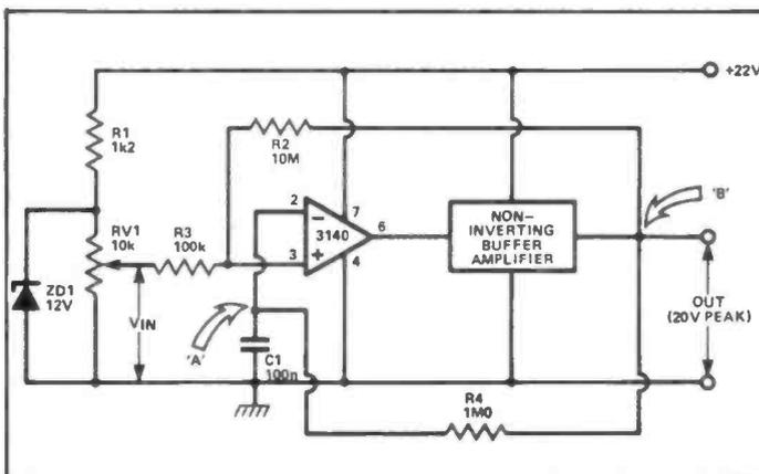
Figure 1: The Switched-Mode Voltage Follower (SMVF) circuit.
