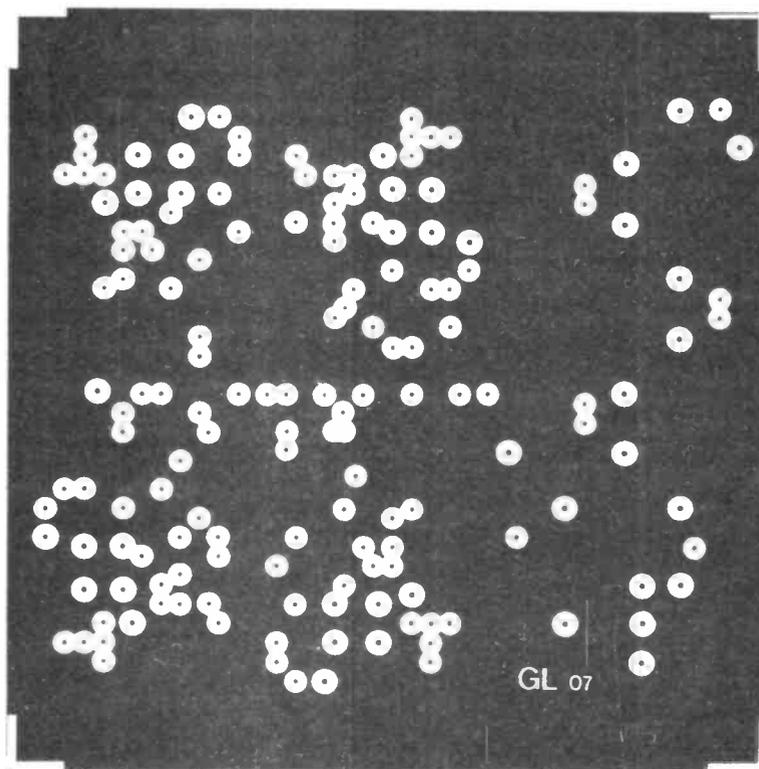
Figure 6: PCB Foil Pattern - Component side.
