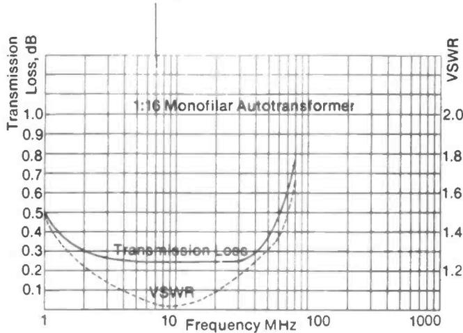
Figure 13: Transmission loss and VSWR.
