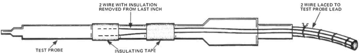
Figure 2: Details of Probe Construction.
