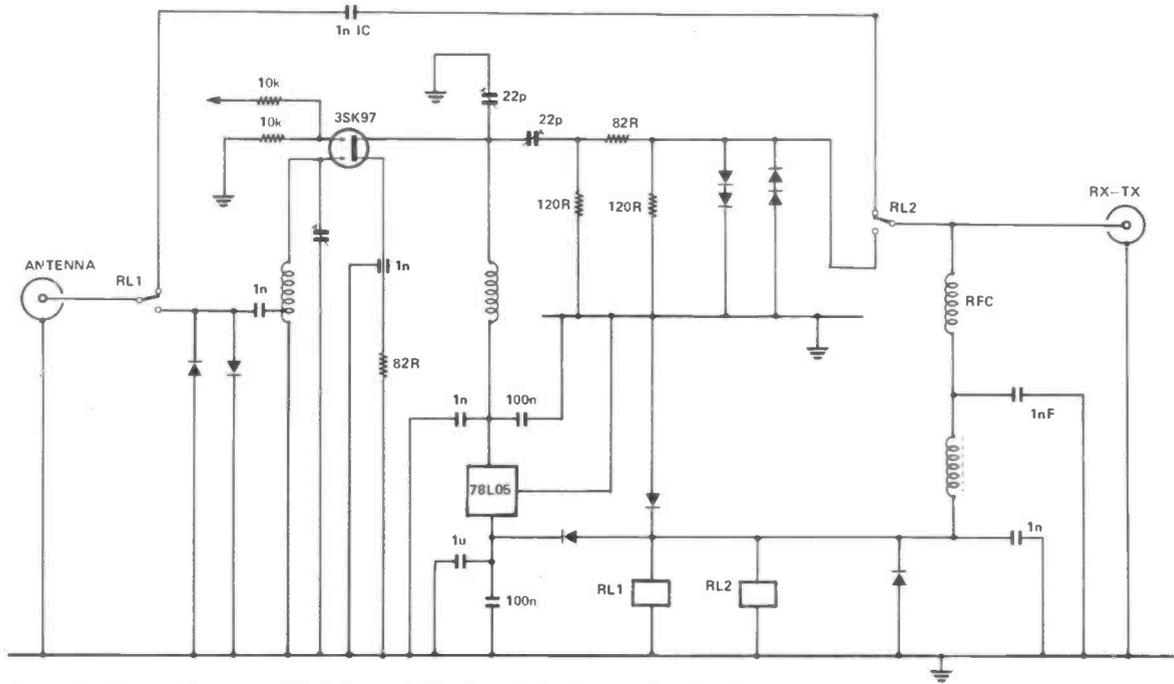
Figure 5: Circuit Diagram of the Masthead Version of the Dressler Pre-Amplifier.
