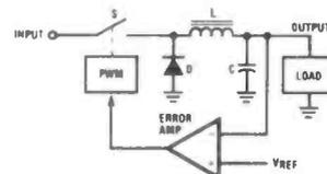
Figure 6: Step-down Switching Regulator Block Diagram.
