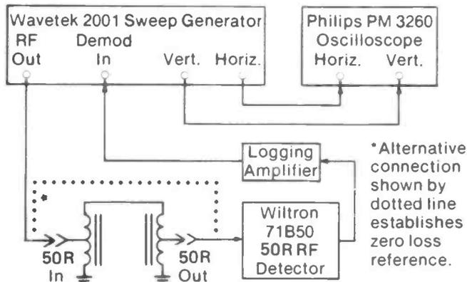
Figure 7: Swept transmission loss test set-up.
