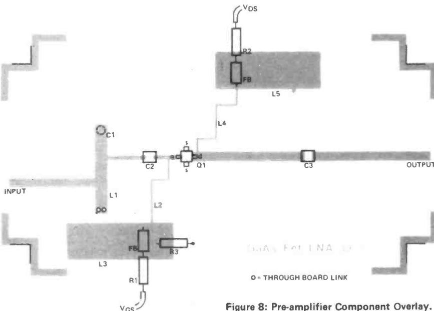
Figure 8: Pre-amplifier Component Overlay.
