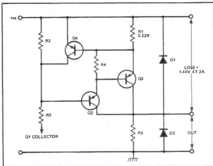
Figure 15: 3 amp output-current limiter.
