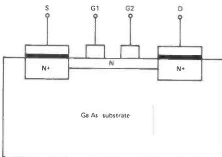
Figure 1: Construction of a Ga As dual gate MESFET.
