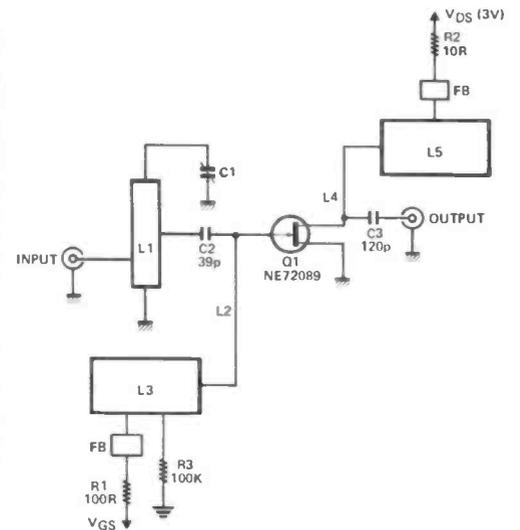
Figure 4: Pre-amplifier Circuit Diagram.
