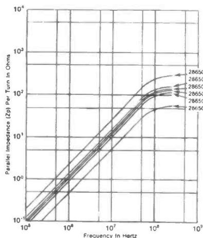
Figure 9: Parallel impedance per turn Vs frequency for Fair-Rite 65 material.
