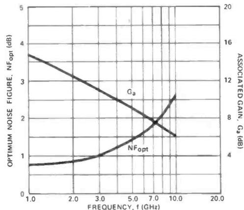
Figure 1b: Typical noise figure and associated gain vs. frequency for the NE72089 at  $V_{DS} = 3V$  and  $I_{DS} = 10mA$ .
