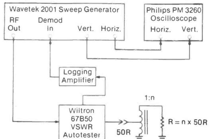
Figure 8: Swept VSWR test set-up.
