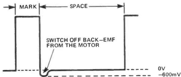
Figure 9: The negative back-EMF of a motor prevents the SMVF circuit from turning fully off when its input is reduced to zero.
