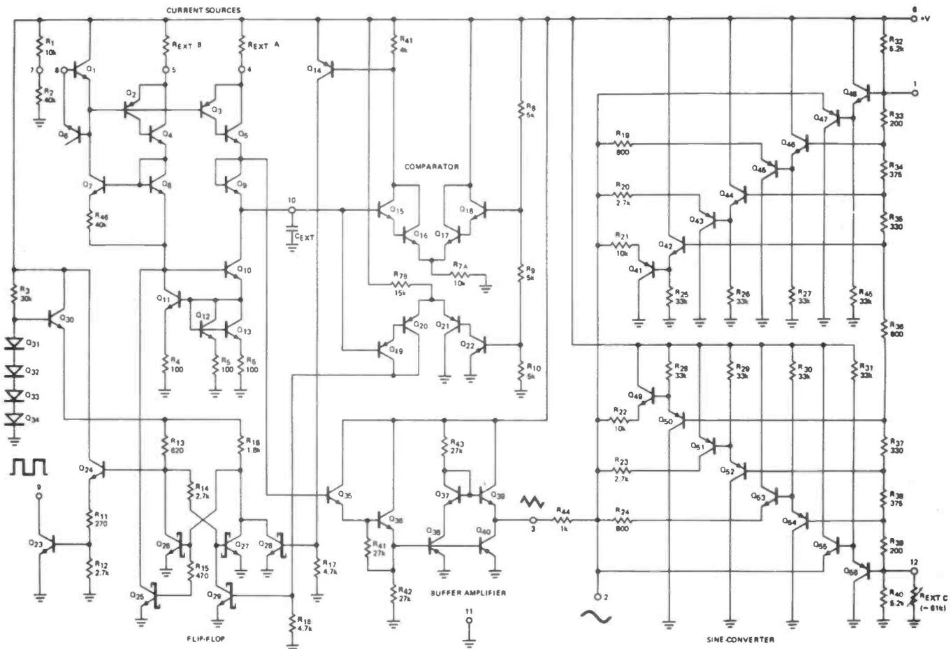
Figure 2 Internal schematic of the 8038, the IC that generates the basic waveforms of the 2001.
