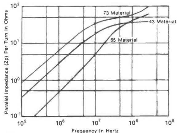
Figure 16 Parallel impedance per turn for a Balun Core in three materials.
