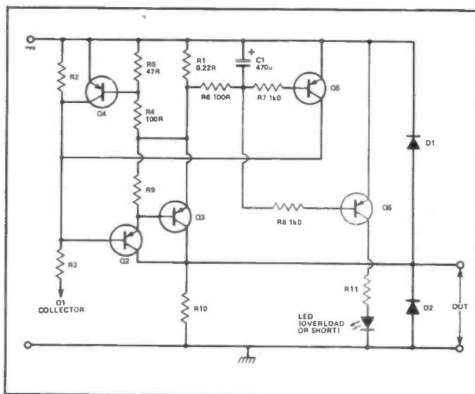
Figure 17: Circuit limits current to 3 amps MEAN but can supply brief transients of 9 Amps. LED indicator is optional.
