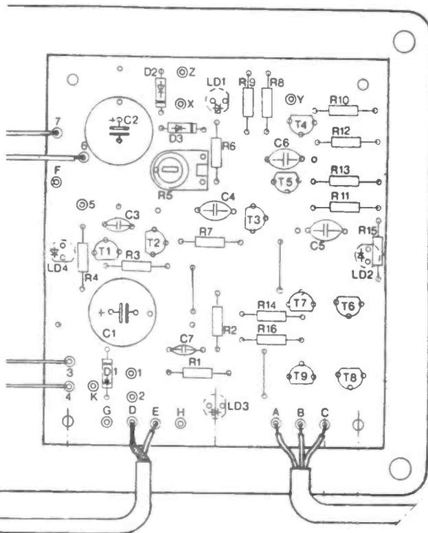
Figure 6: The overlay of the Windspeed and Direction Indicator's PCB.
