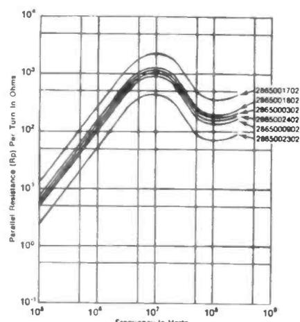
Figure 11: Parallel resistance per turn Vs frequency for Fair-Rite 65 material.
