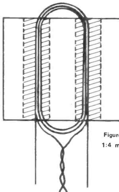
Figure 12: Cutaway drawing of 1:4 monofilar autotransformer.
