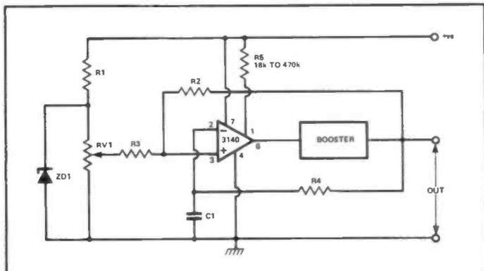
Figure 10: Offset biasing via pin 1 of the op-amp.
