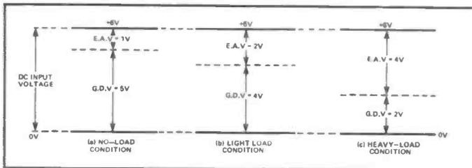
Figure 3: A voltage-controlled DC motor has excellent regulation, because its speed-dependent 'Generated Dynamo Voltage' (GDV) decreases as the load increases and thus causes the Effective Applied Voltage (EAV) to increase. Its low-speed control is, however, very poor.
