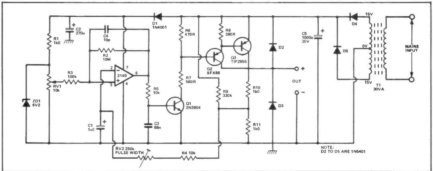
Figure 14: High-efficiency mains-powered version of the SMVF circuit.
