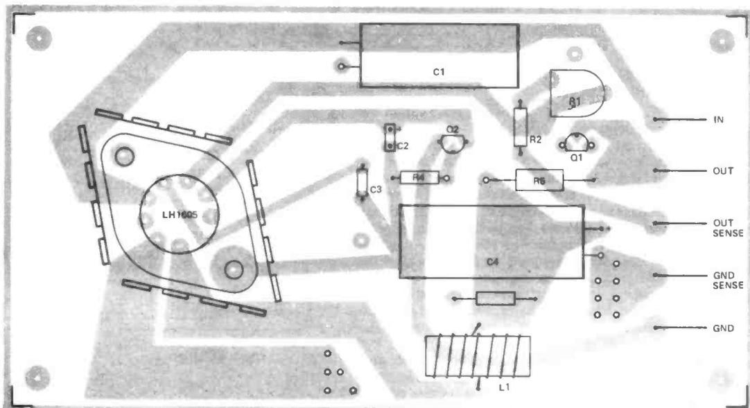
Figure 4: PCB Overlay.
