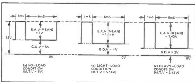
Figure 4: A conventional 'fixed-frame' pulse-controlled DC motor has good low-speed control, but poor regulation.
