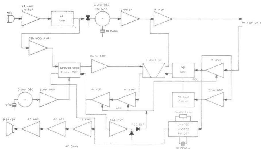
Figure 1: Block Diagram of the IC290.
