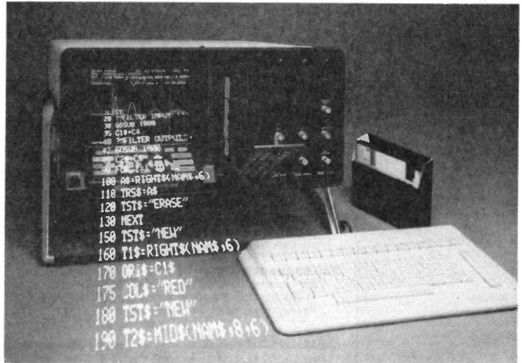
tions have been included in the software to allow better analysis for the frequency domain display; the user may select 'Flat' for no weighting, 'Hanning Window' or self-defined window.
