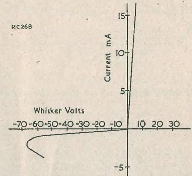
FIG.1. Static characteristics of typical germanium crystal diode
