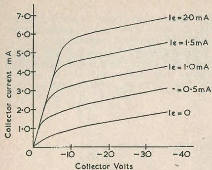
FIG. 3. Static characteristics of typical point contact transistor
