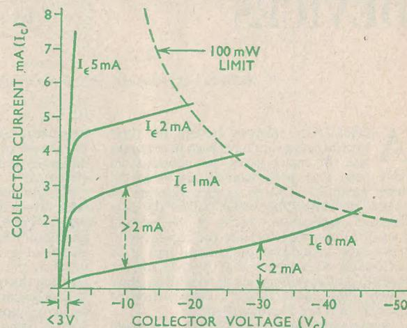
Static characteristics of G.E.C. point-contact germanium triode.
