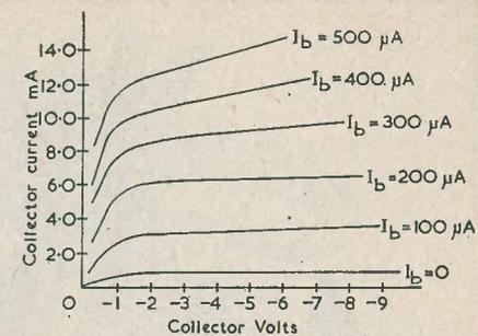
FIG. 5. Collector characteristic of typical p-n-p junction transistor
