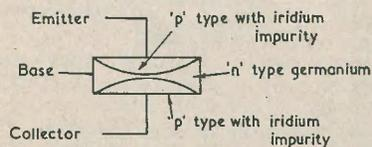
FIG. 4. Diagram of p-n-p junction transistor
