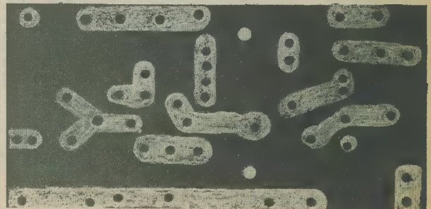
The copper side of a practical printed circuit board made up to the pattern in Fig. 2
