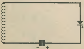
Fig. 6. The first bypass capacitor following an a.m. detector diode charges up with the polarity shown here, whereupon the diode is reverse biased between half-cycle tips
