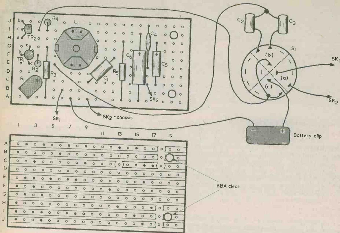
Fig. 4. Illustrating how the components are assembled on the Veroboard panel, together with the wiring to the switch and the battery
