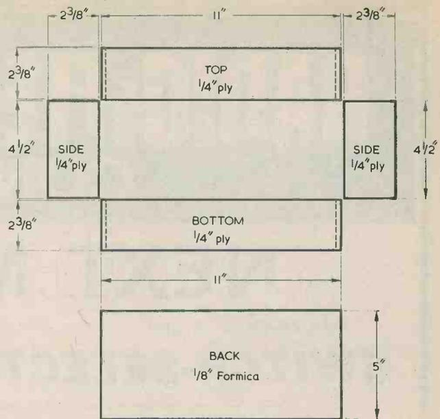
Fig. 4. Details of the items which make up the case. The dimensions may require slight amendment as described in the text
