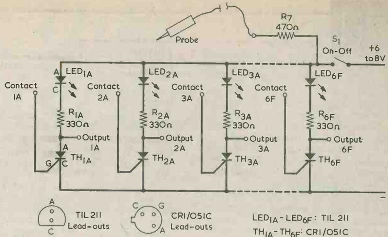
Fig. 2. All the green l.e.d.'s on the front panel have identical circuits, and four of these are shown here
