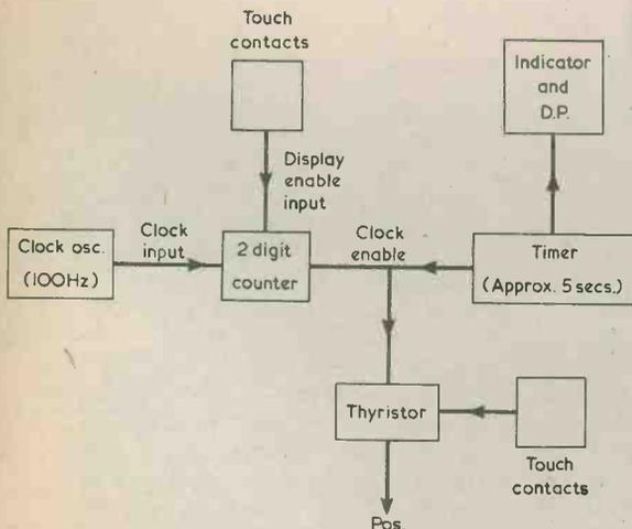
Fig. 1. Block diagram illustrating the operation of the digital reaction timer
