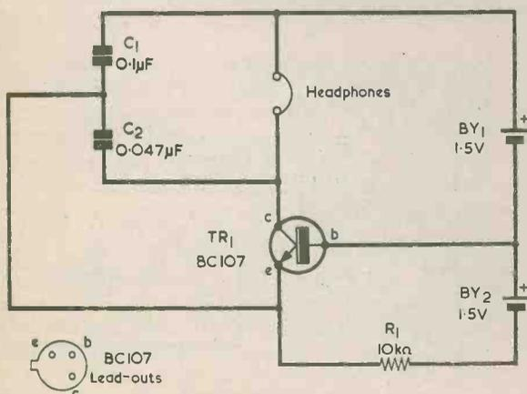
Fig. 1. The basic circuit of the oscillator. Despite its simplicity it functions satisfactorily with headphones of the type specified in the text
