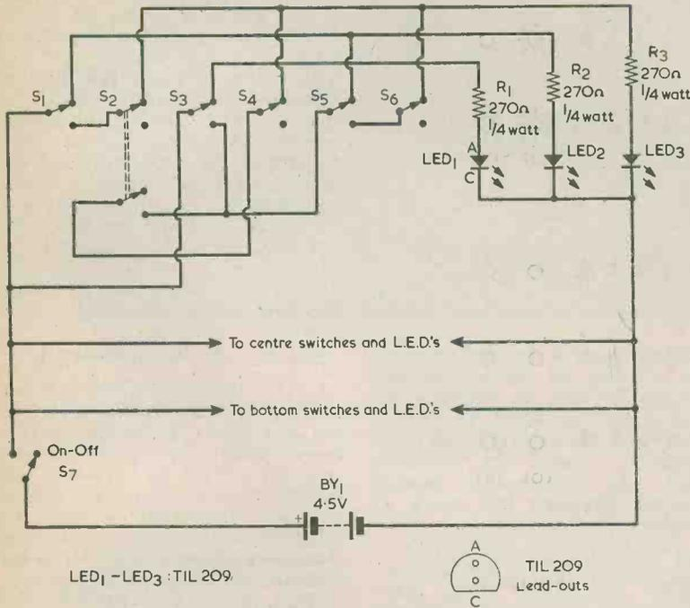
Fig. 7. The switching circuit for the top row of switches and l.e.d.'s. The switch and l.e.d. suffix numbers correspond with those shown in Fig. 4. Identical circuits are used in the centre and bottom rows.
