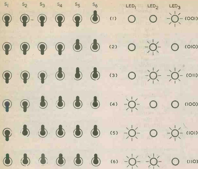
Fig. 4. The l.e.d.'s indicate, in binary notation, the number of switches which are up. The displays, from one to six switches, are shown here.
