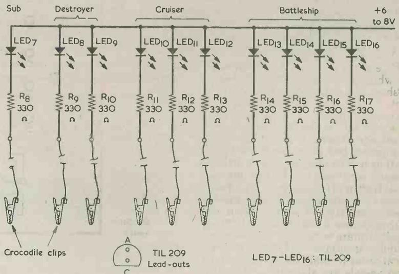
Fig. 3. The circuit for the red l.e.d.'s. It is helpful to distinguish the flying colours by using different colours for each vessel, the lead for the submarine being say, green, those for the destroyer blue, those for the cruiser yellow and those for the battleship red. All resistors have and in Fig. 2 are 1/4 watt 10%
