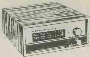
200/240V Mains operated Solid State A/M F/M Stereo Tuner. Covering M.W. A.M. 540-1605 KHZ. VHF/FM 88-108 MHZ. Built-in Ferrite rod aerial for M.W. Full AFC and AGC on AM and FM. Stereo Beacon Lamp Indicator. Built-in Pre-amps with variable output voltage adjustable by pre-set control. Max o/p Voltage 600 mV RMS into 20K. Simulated teak finish cabinet. Will match almost any amplifier. Size 8 1/2" w. 4 1/2" h. x 9 1/2" d. approx. LIMITED NUMBER ONLY at £28 + £1.50 P. & P.
