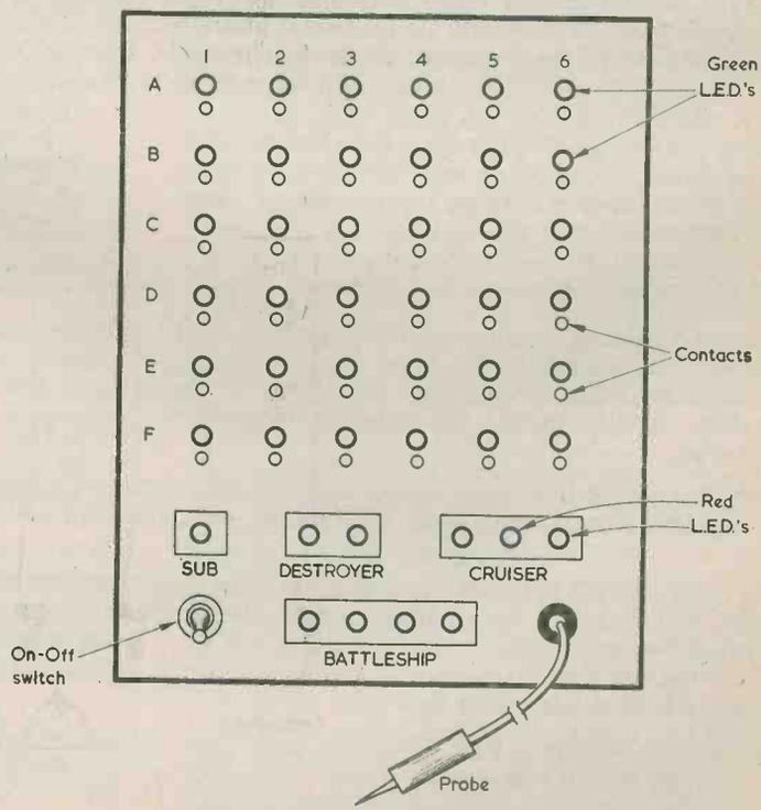
Fig. 1. The front panel of the electronic "Battleships" game has the appearance shown here. The appropriate red l.e.d.'s light up when a vessel is hit
