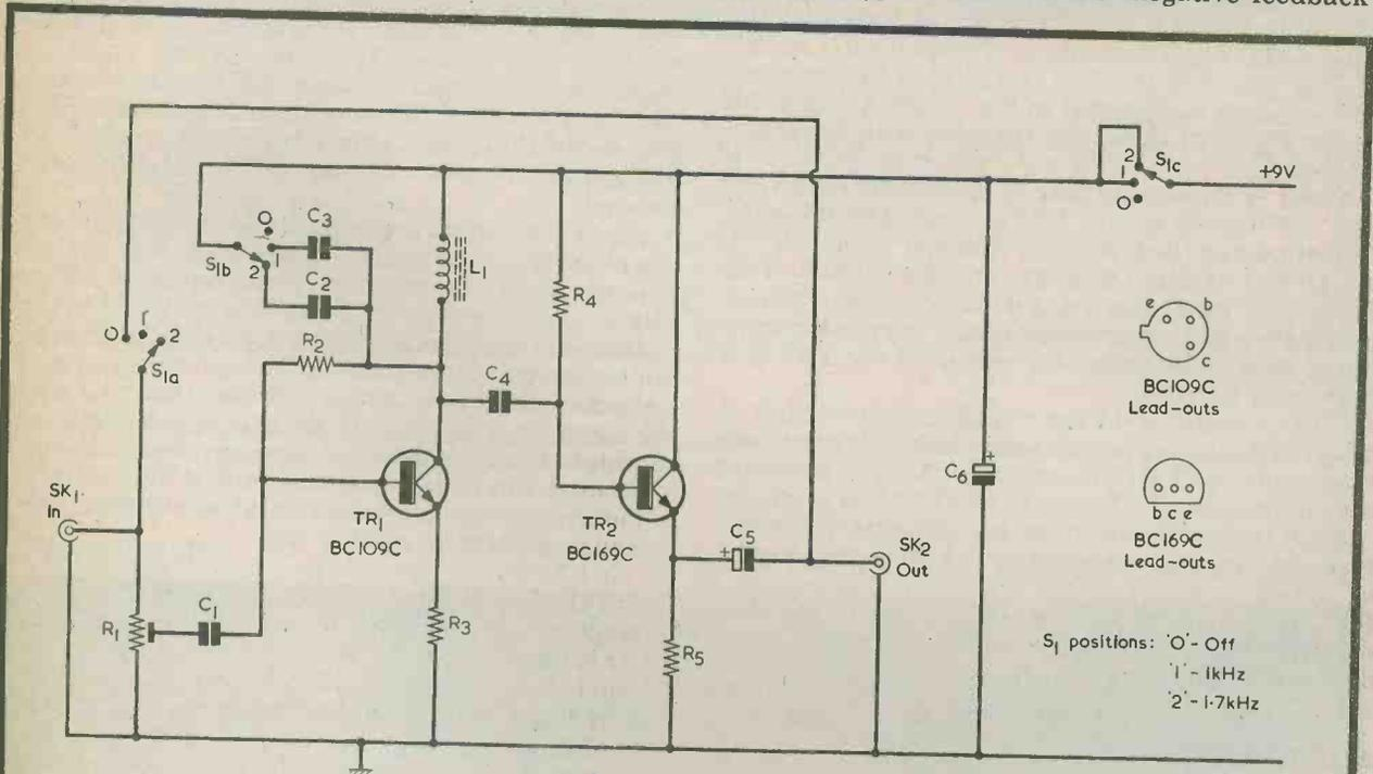
Fig. 2. The circuit of the c.w. filter unit. When the unit is switched off the input at SK1 is coupled directly through to the output at SK2
