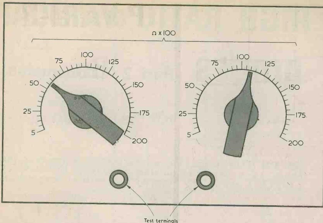
Fig. 2. A front panel layout for the box. The panel can be covered with a sheet of white card on which the scales are marked out. The legend at the top acts as a reminder that units are in hundreds of ohms
