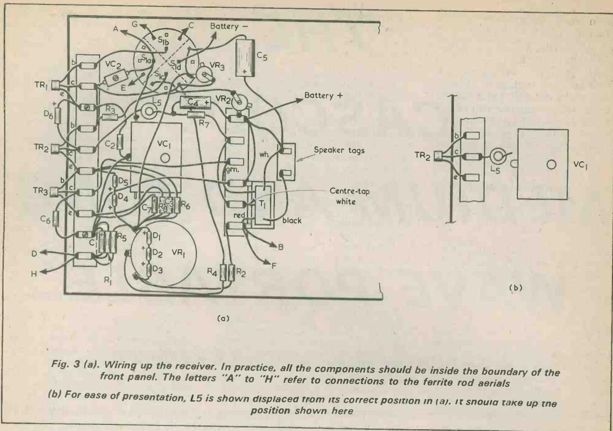
Fig. 3 (a). Wiring up the receiver. In practice, all the components should be inside the boundary of the front panel. The letters "A" to "H" refer to connections to the ferrite rod aerials
