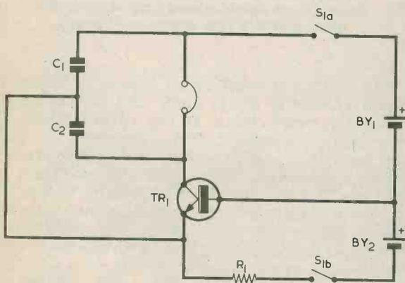
Fig. 4. On-off switching is required if the oscillator is to be assembled in permanent form
