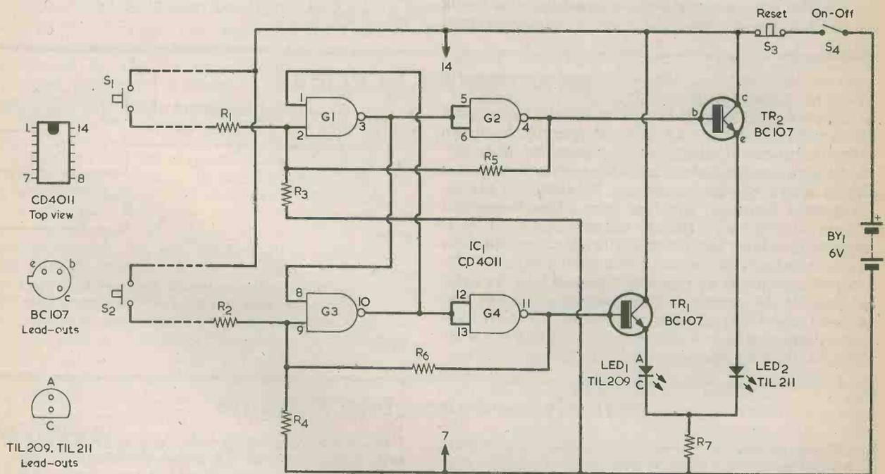
Fig. 1. The circuit of the precedence monitor. The four gates of the CD4011 form two separate latches, each being inhibited when the other latch changes state.
