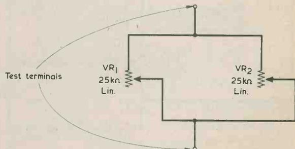
Fig. 1. The circuit of the parallel-R box. A multimeter switched to a suitable ohms range connects to the test terminals
