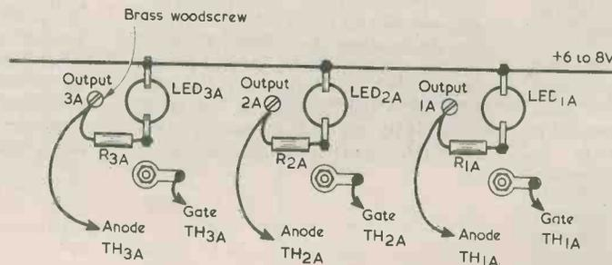
Fig. 4. A suitable layout behind the panel for each green l.e.d., series resistor and Output contact
