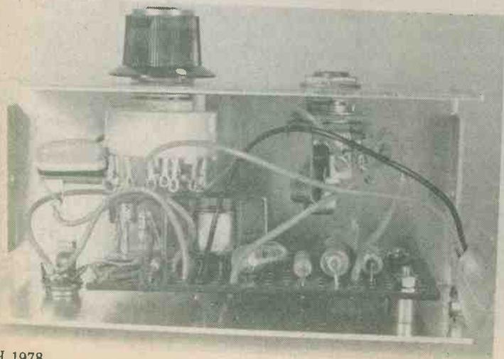
The layout of parts inside the case. C2 and C3 are mounted on the tags of the rotary switch
