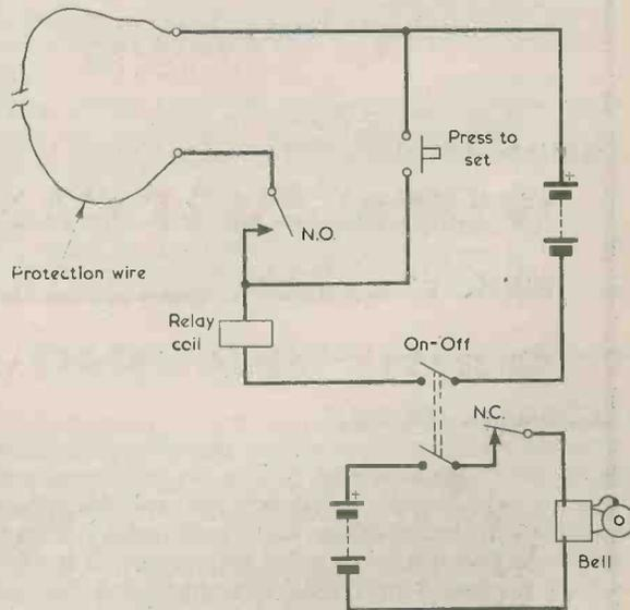
Fig. 1. A very simple protection circuit. It has the disadvantages that the relay coil draws a continuous current and that the protection wire can be easily bridged
