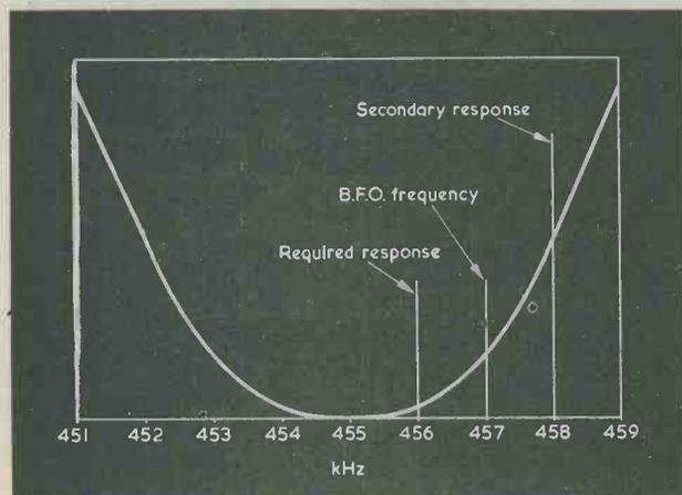
Fig. 1. When using a 1kHz audio filter, there are two peaks of response 1kHz either side of the b.f.o. frequency. The i.f. response of the receiver is used to attenuate one response (that at 458kHz in this case) in relation to the other
