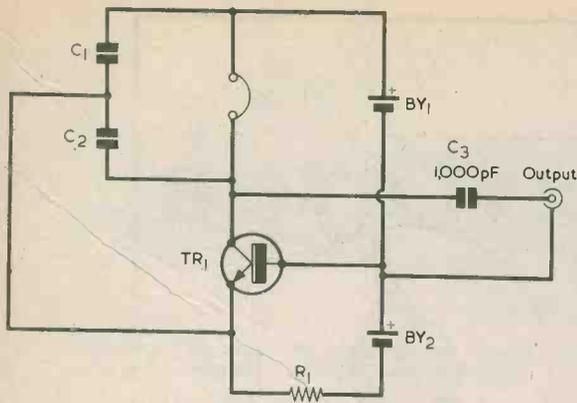
Fig. 3. Adding a series output capacitor enables the oscillator to function as an a.f. signal generator
