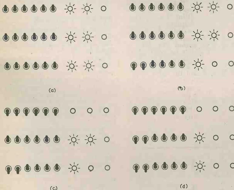
Fig. 2(a). When the game is turned on initially, all the switches are up and the l.e.d.'s are illuminated as shown here.
