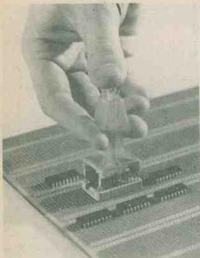
Vero Electronics of Industrial Estate, Chandler's Ford, Eastleigh, Hants, have introduced a new and simple hand tool for the insertion of integrated circuits into boards or sockets.
