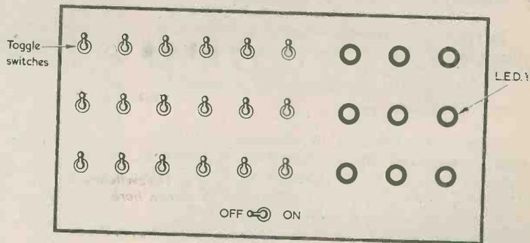
Fig. 1. The front panel layout of the NIM game. There are two players, each of which puts down any number of switches in a single row. The loser is the person who puts down the last switch
