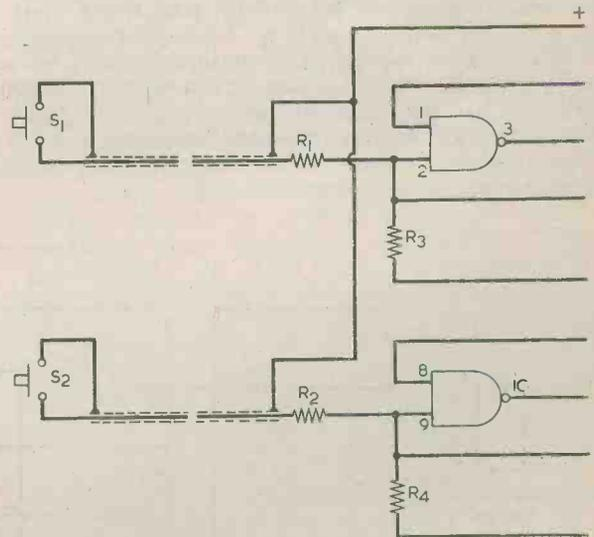
Fig. 2. In instances where the leads to S1 and S2 are very long it is advisable to couple them to the main part of the circuit by way of screened cable.
