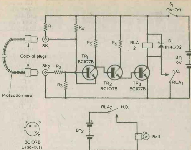
(when 4.5 volts appears across the transistor) is 135mW. The power dissipation is low when TR3 is off or hard on. Naturally, current drain from BY1 when the alarm is sounding reduces as relay coil resistance increases. A suitable relay would be the type listed by Home Radio; this has 2-pole double throw contacts, a coil resistance of 185Ω, and it energises at 6 volts. The relay used by the author was a type P.O. 3000 with a 500Ω coil. A diode across the relay coil prevents the appearance of a
