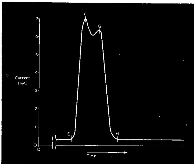
Fig. 6. The circuit of Fig. 5 features low VDD current drain except for a short period at the end of the timing cycle
