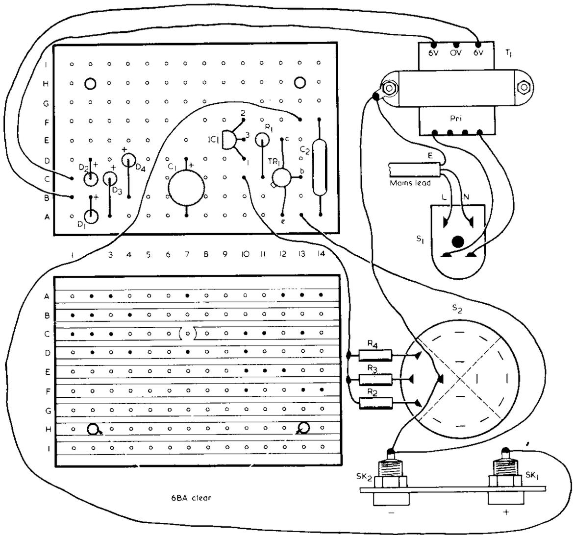
Fig. 4. Layout of components on the Veroboard and the general wiring of the battery eliminator
