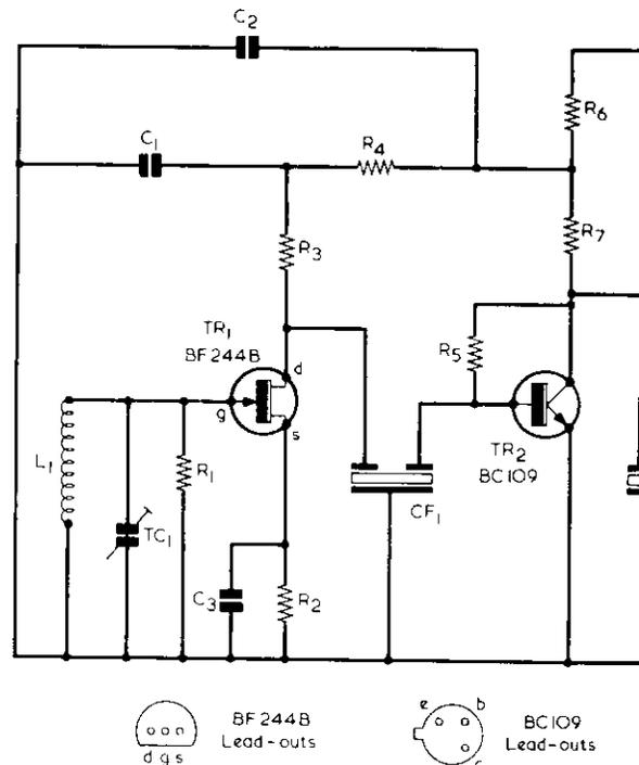
Fig. 1. The circuit of the television sound adaptor which extracts the inter-carrier signal from the TV set. This is amplified and processed to produce an audio output.
