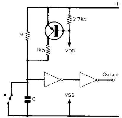
Fig. 4. Adding a silicon transistor to curtail the timing period at a low level of VDD current
