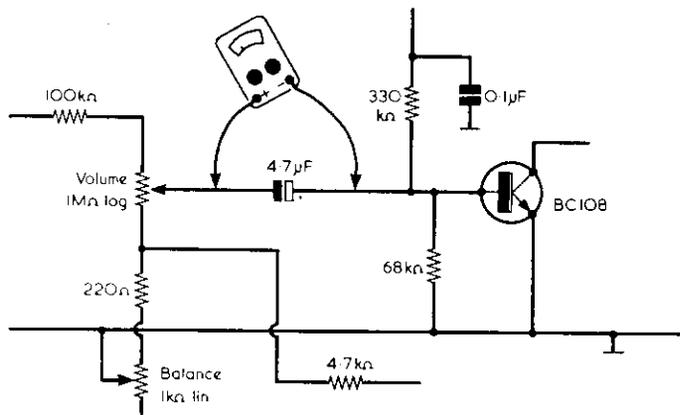
Fig. 3. Checking the electrolytic capacitor coupling the volume control slider to the base of the BC108
