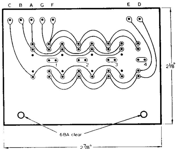
Fig. 6. The copper side of the display board. Connections shown here as lines are, in practice, narrow copper tracks. Like Fig. 5, this is reproduced full size for tracing
