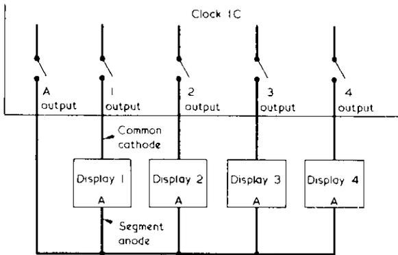
**Fig. 2. Demonstrating the multiplexing technique. The electronic switches to outputs 1, 2, 3 and 4 close in order, driven by an internal oscillator in the i.c.**
