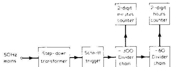
Fig. 1. Simplified block diagram illustrating the stages which allow the 50Hz mains supply to control the minutes and hours display of a digital clock
