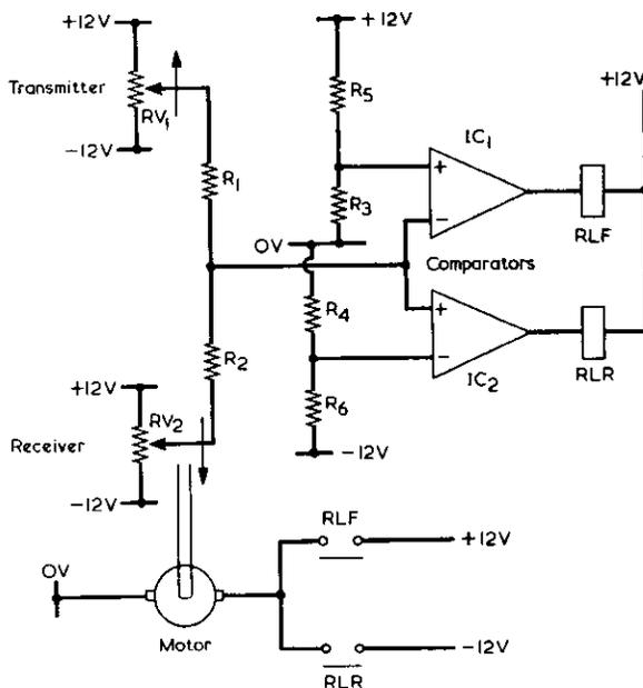
Fig. 2. A "bang bang" servo system. The arrows alongside the potentiometers indicate clockwise rotation
