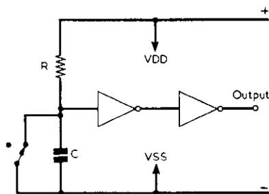
Fig. 1. A simple timing circuit incorporating two CMOS inverters
