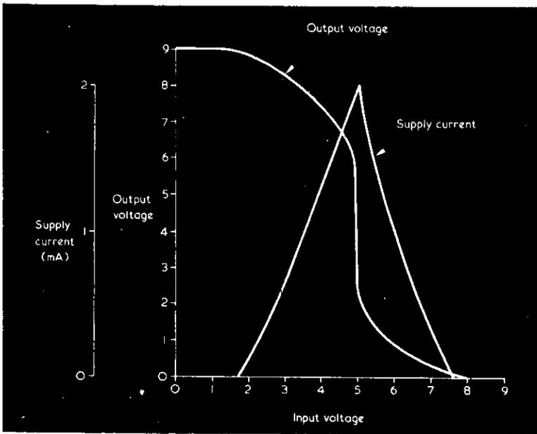
Fig. 2. Typical supply current and voltage transfer characteristics for a CMOS inverter operating from a 9 volt supply
