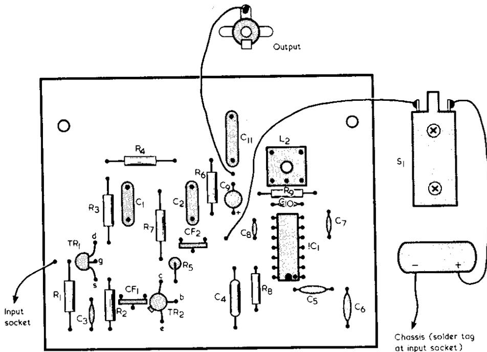
Fig. 2. Details of the printed board assembly. This is reproduced full size for tracing
