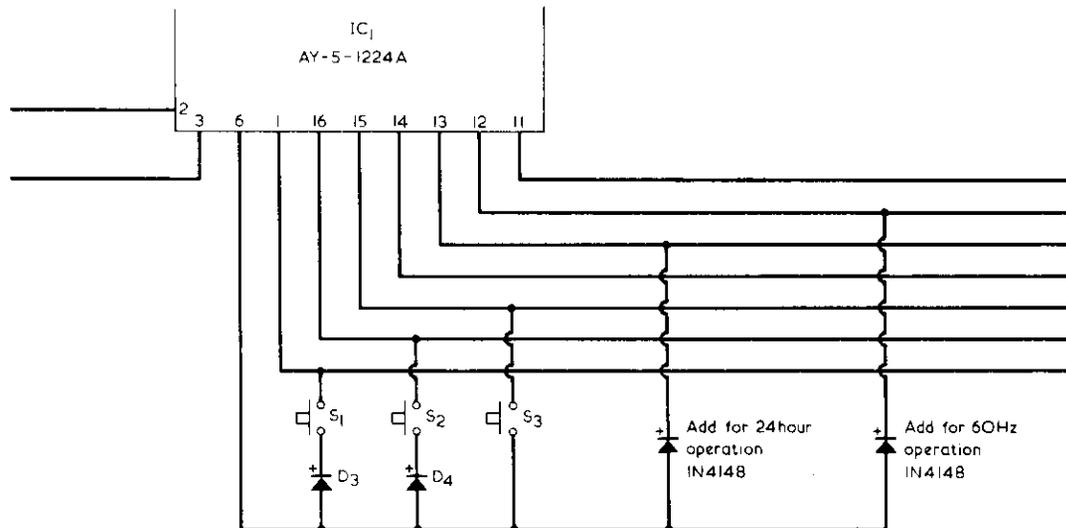
Fig. 7. An additional diode is connected to the circuit if it is desired to have 24 hour operation, or if the clock is to function with a 60Hz mains supply
