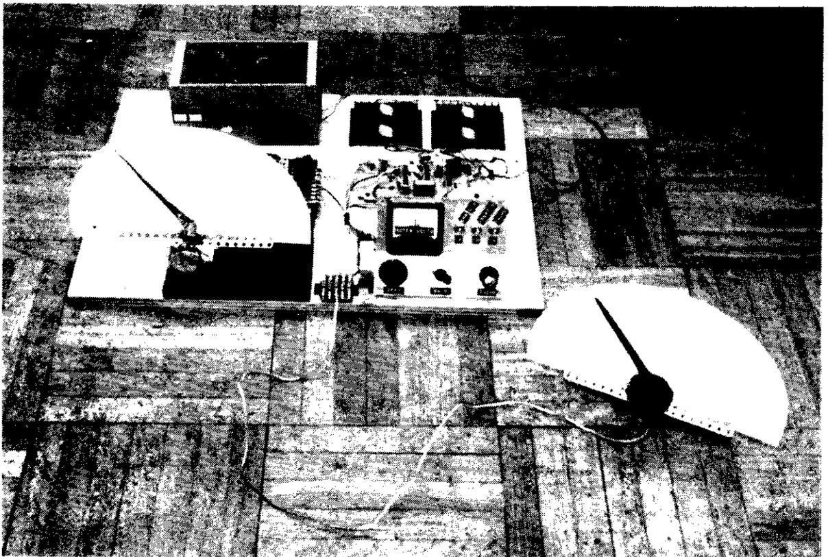
*The complete servo system. The transmitter pointer and dial are in the separate unit coupled by a length of wire to the main receiver section*
