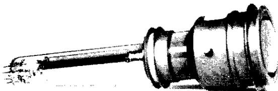
An overall view of the Westinghouse Electric WX-30654 SEC camera tube with electrostatic image section
