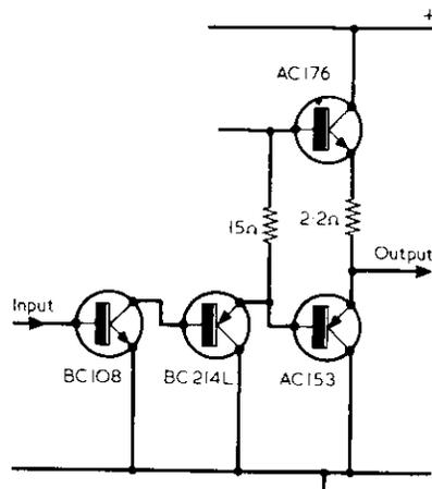
Fig. 4. The only voltage amplification in the amplifier is given by the BC108. The three transistors which follow are all emitter followers
