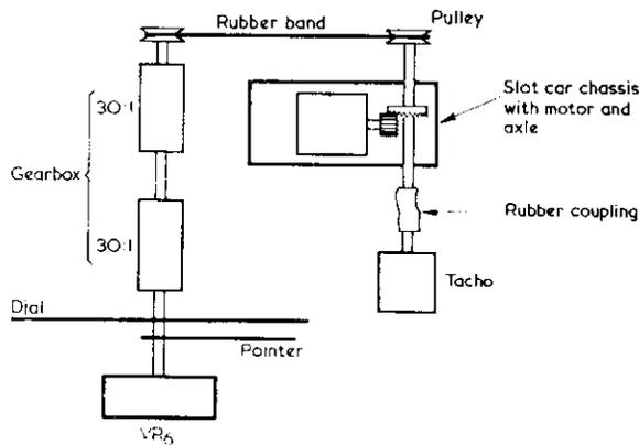
Fig. 6. The mechanical layout of the motor, tacho and drive to the receiver pointer
