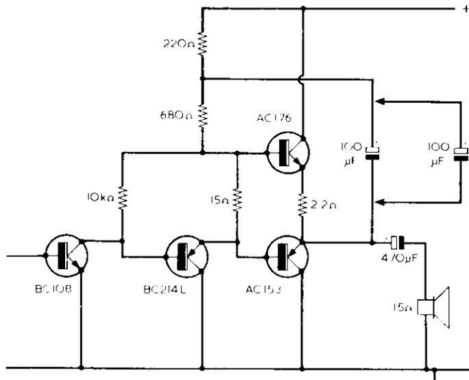
Fig. 7. Smithy experimentally bridged the 100 $\mu$ F capacitor in the amplifier by another of the same value. This capacitor provides the bootstrap coupling to the top of the 680 $\Omega$  resistor, causing this to go positive as the signal output voltage goes positive
