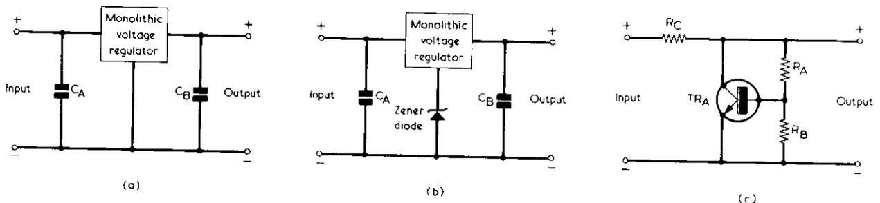
Fig. 1(a). A monolithic voltage regulator can employ the circuit shown here. An unstabilized supply voltage is applied to the input and the regulated voltage appears at the output
