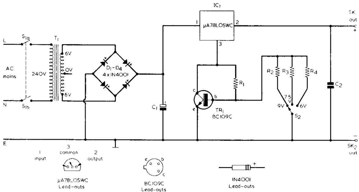
Fig. 3. The circuit of the 3-voltage battery eliminator. No connection is made to the centre-tap of the mains transformer secondary. Output voltages are selected by S2
