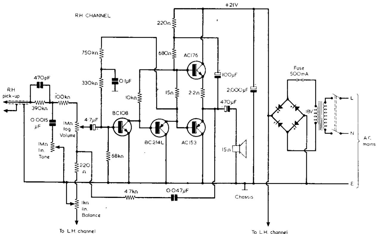
Fig. 1. One channel of an inexpensive stereo record player. The tone and volume controls of the left hand channel are ganged with the similar controls in the right hand channel. Component values are representative of commercial practice
