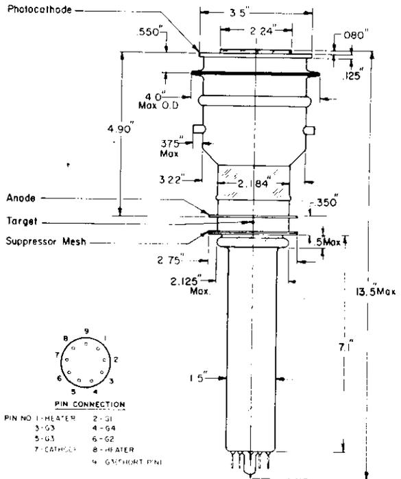
Dimensions of the new camera tube. The pins at the base cater for heater, cathode and four grids. Pin 9 is a short pin for cathode purposes
