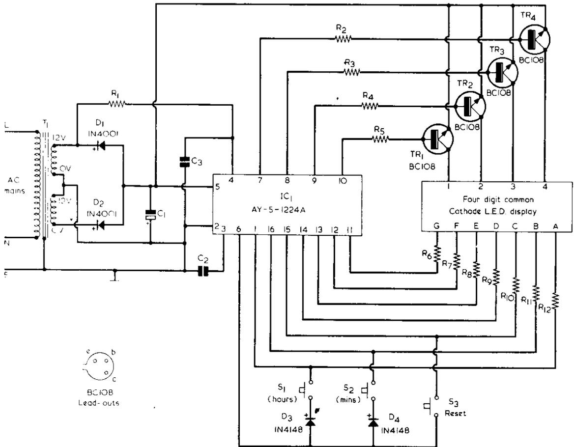
Fig. 3. The circuit of the single i.c. digital clock. For ease of presentation the four DL704 displays are shown as a single display block
