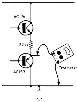
Fig. 2(a). First, Smithy measured the supply voltage applied to the output transistors
