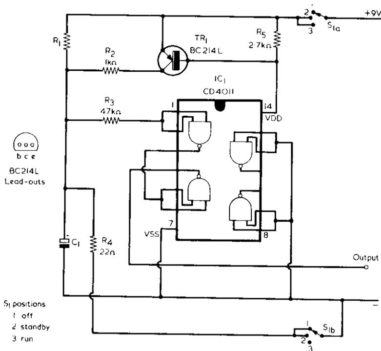
Fig. 5. A practical working version of the timer with two inverters and a transistor. The length of the timing period is controlled by the values of R1 and C1
