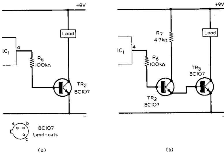
Fig. 7(a). The output of the timer can switch on a load with the aid of an external transistor
