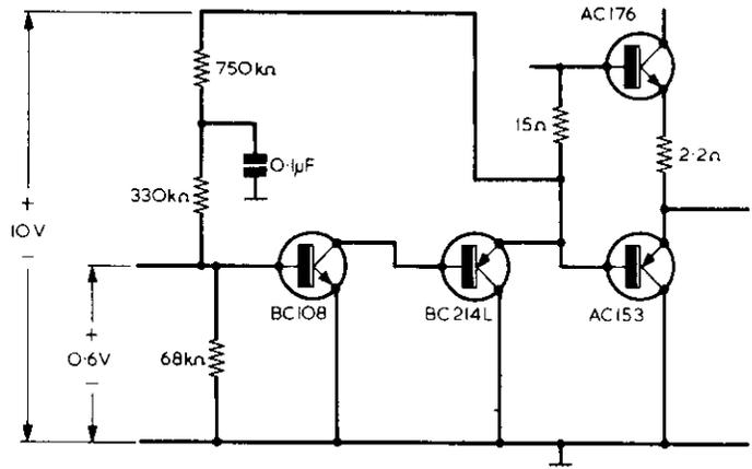
Fig. 5. The d.c. feedback loop consists of a potential divider given by the three resistors from the BC214L emitter to chassis. Their values cause about 0.6 volt to appear at the BC108 base when the BC214L emitter is at 10 volts
