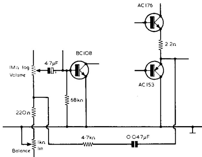
Fig. 6. A.C. negative feedback is provided via the 0.04μF capacitor and the 4.7kΩ resistor
