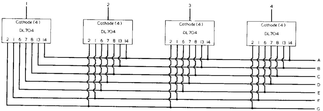
Fig. 4. Detailed circuit illustrating the connections to the DL704 displays. The display pin numbers correspond with the appropriate segments from A to G
