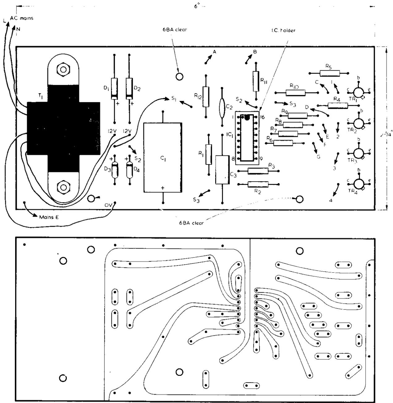
Fig. 5. Component and copper sides of the main printed board. The letter and figure references correspond with the same references in Fig. 6
