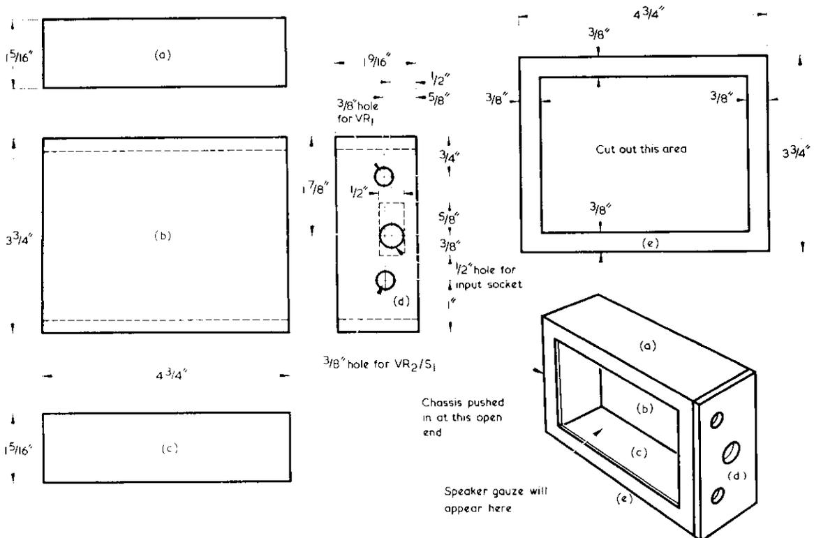
Fig. 6 A case may be made up in the manner shown here with items (a) to (e) inclusive. The finished assembly appears as in (f). Dimensions are for guidance only
