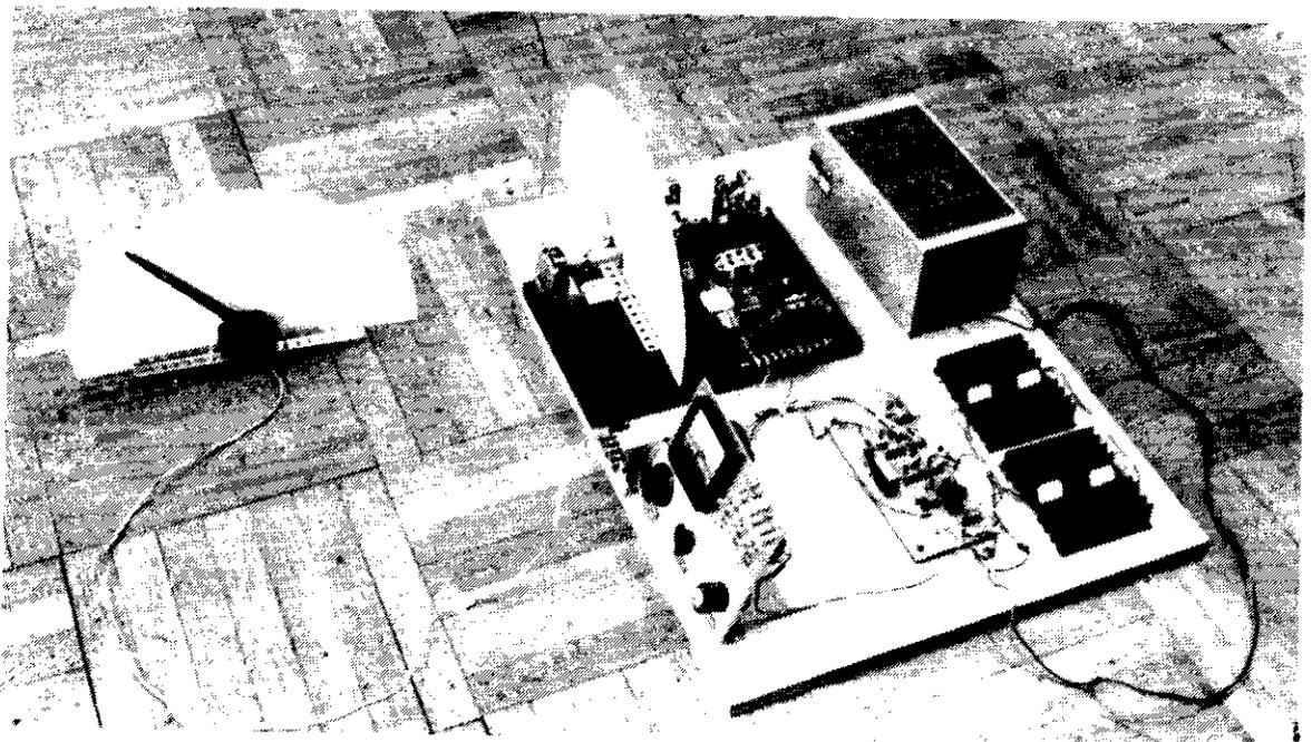
*The receiver potentiometer is mounted in front of the receiver dial. At the rear of the receiver board is the power supply, with the output transistor heat sinks to its right. The positions of other parts of the receiver section are described in the text*
