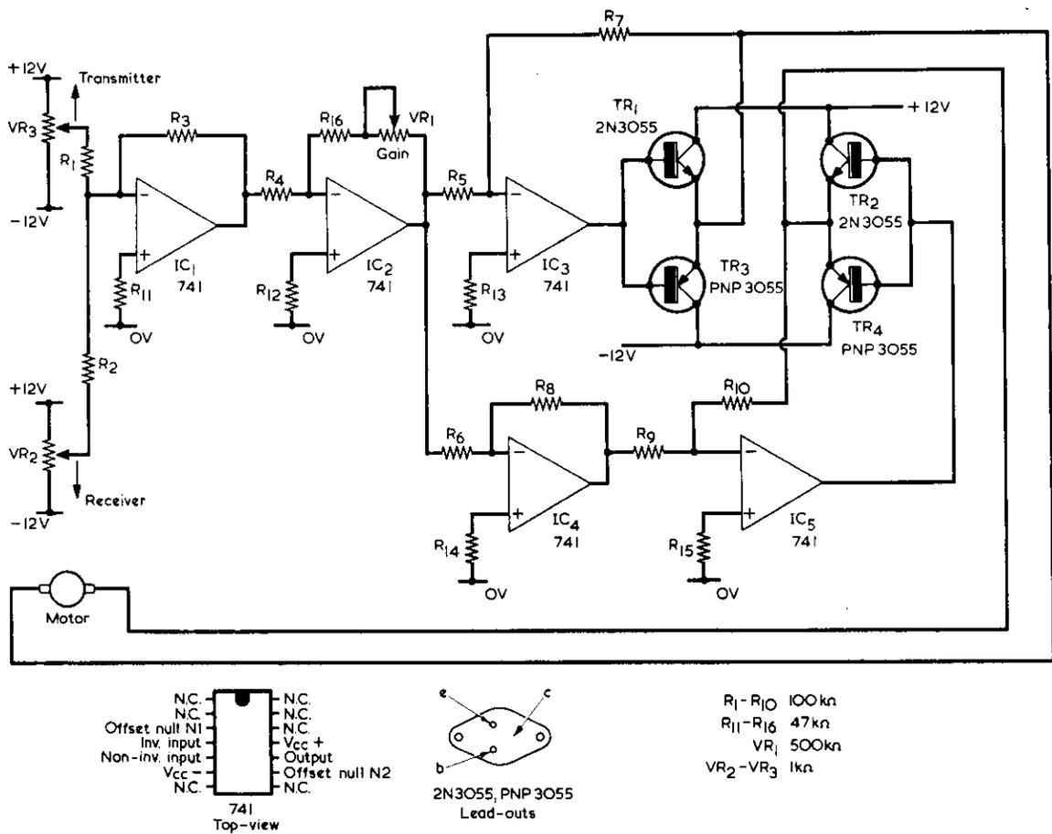
Fig. 3. A proportional servo system. (No connections are made to the offset null pins of the 741's)
