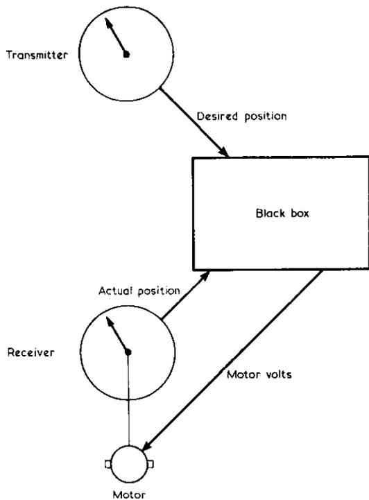
Fig. 1. Block diagram illustrating a simple position control system
