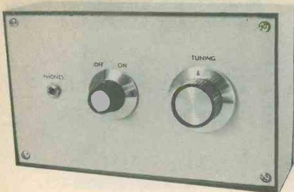
To ensure that the ferrite rod aerial is not screened the receiver is housed in a plastic case.
