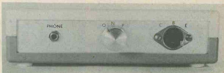
The Go-No Go Transistor Tester. The only control is the 3-way switch in the centre of the front panel, and this selects "Off", "N.P.N." and "P.N.P." The test transistor connects to the DIN socket on the right of the panel.
