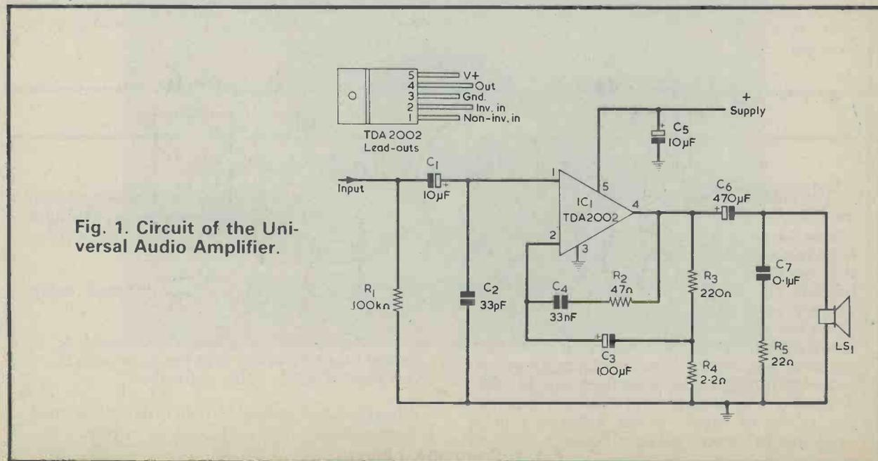
Fig. 1. Circuit of the Universal Audio Amplifier.
