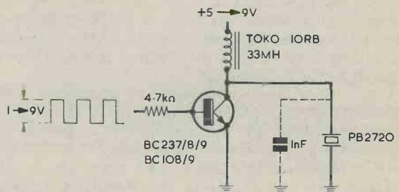
Fig. 6. An inductive voltage multiplier for increased output.
