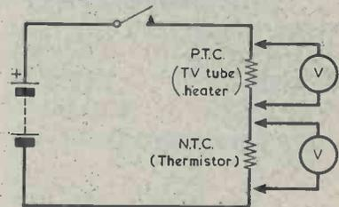
Fig. 5. When first switched on the heater and thermistor are cold. The heater is therefore low resistance, but the thermistor is high resistance and prevents any damaging current surge.
