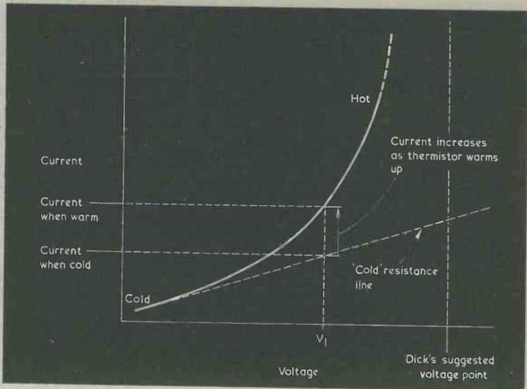
Fig. 4. Graph showing how the current through a Negative Temperature Coefficient thermistor increases as it heats up.
