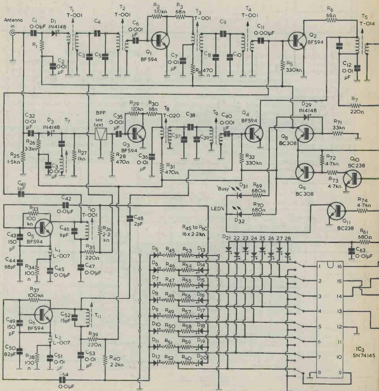
Fig. 3. Circuit of complete receiver. Details
