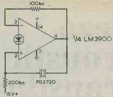
Fig. 5. Using a spare 'Op-amp' section.
