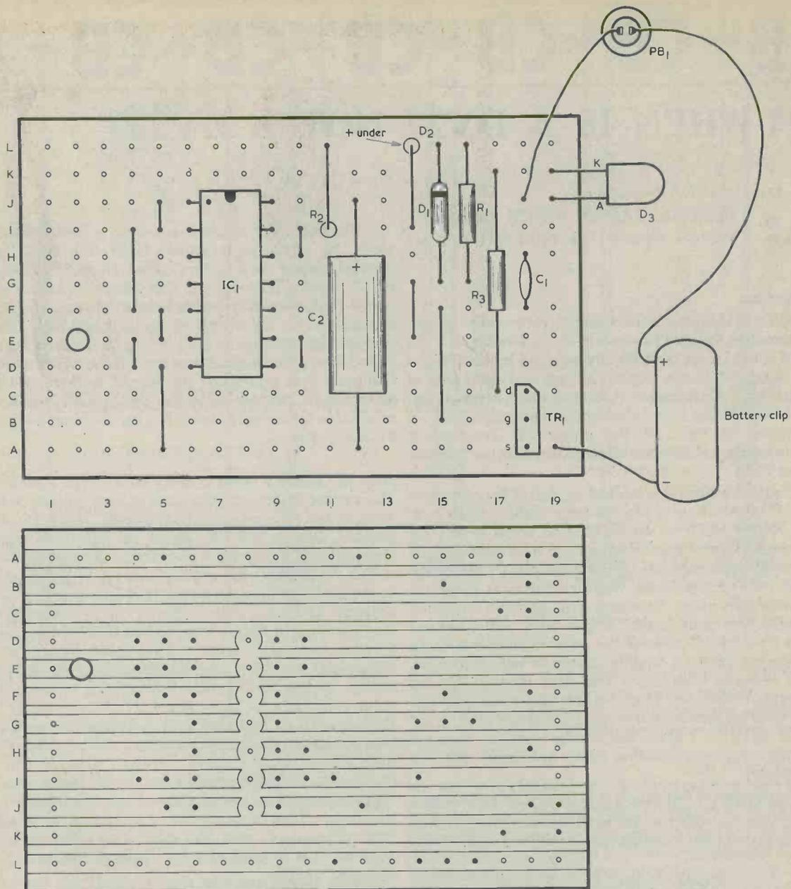
Fig. 3. The 0.1in. matrix stripboard layout for the Infra-Red Transmitter.
