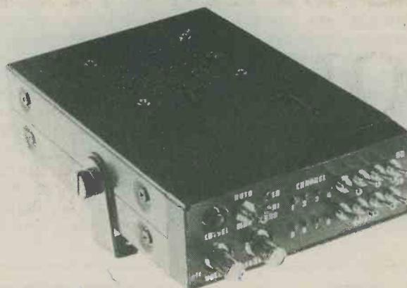
The LED remains lit above the appropriate channel indicator until the transmission ceases – and after a brief pause (determined by presettable values in the circuit) – the scanning is resumed until stopped by a signal once again.
