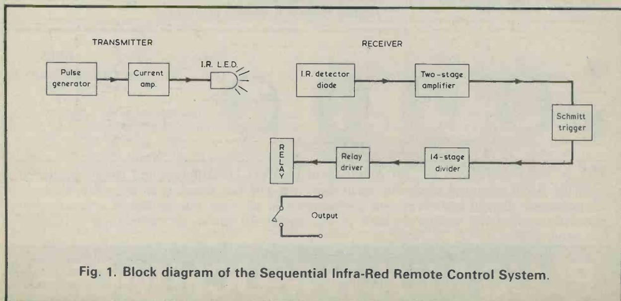
Fig. 1. Block diagram of the Sequential Infra-Red Remote Control System.
