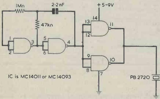
Fig. 4. Simple CMOS drive.
