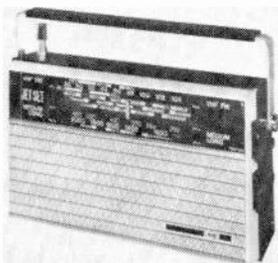
**KB's** new Jet Set model KR 607 ▲ covers l.w., m.w. and f.m. bands and has a 5 x 3in speaker. A two-position tone control is fitted. The cabinet is in black and silver. Power is from four U11 batteries. Price including earphone, 14½gn. **E427**
