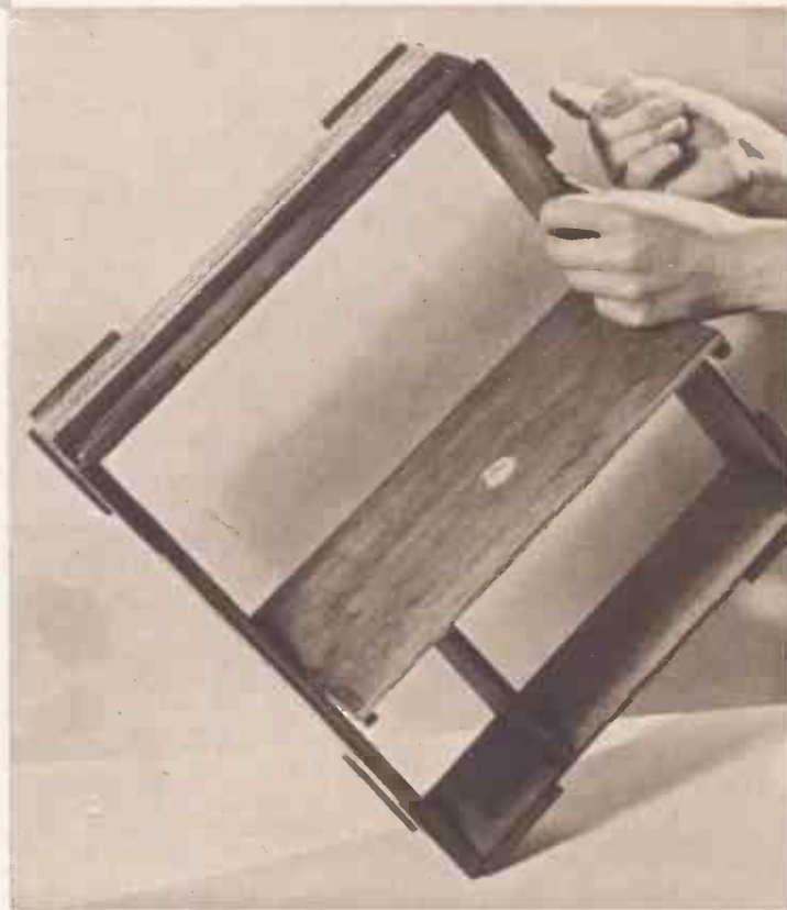
Below shows the wooden frame-work on which the frame aerial for the TWO H.F. PORTABLE is wound.
