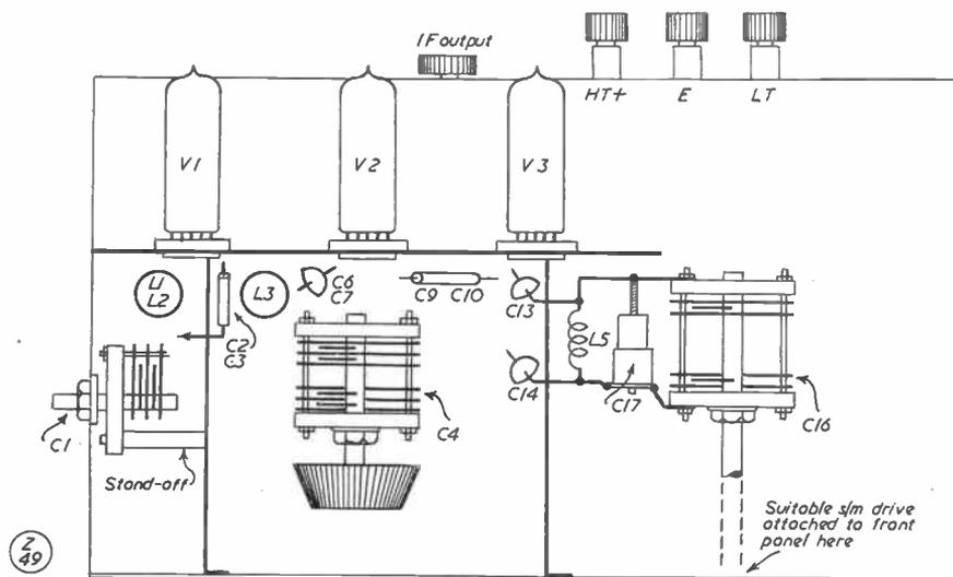
**Fig. 2.** Physical layout for the G2IQ two-metre converter; the oscillator stage is to the right, the mixer in the centre, and the RF stage at left. Some valuable practical advice on construction is given in the article.
