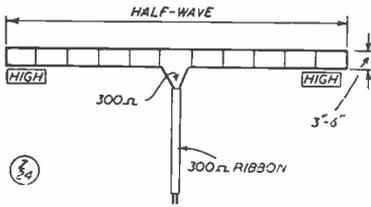
Fig. 6. The Folded Dipole mode of operation, using Telcon 300-ohm ribbon feeder, which is light, strong and very low-loss, and therefore ideally suited to these applications.
