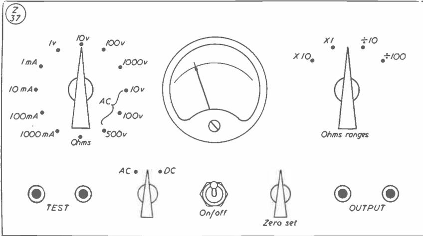
Fig. 11. Suitable panel layout for the instrument for which the full circuit is given at Fig. 10.
