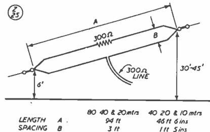
Fig. 7. A recently developed amateur aerial design, suitable for both transmission and reception. It is a multi-band system, and therefore is becoming popular, particularly as space requirements are reasonable. This system is known as the "T2FD."
