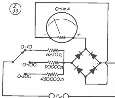
Fig. 7. The basic AC voltmeter.
