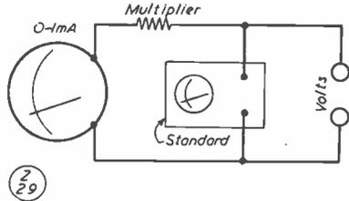
Fig. 2. How to check voltage multiplying resistors using a standard instrument.
