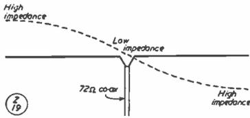
Fig. 1. Illustrating impedance effects on a half-wave dipole, and the principle of matching.
