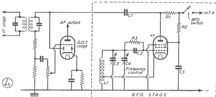
Fig. 3. Using a separate Beat Frequency Oscillator, as described in the text. To the left is the existing receiver output stage, showing the point of connection for the BFO injection. Values are: C1, 2-5  $\mu\text{F}$ ; C2, 100  $\mu\text{F}$ ; C3, 100-500  $\mu\text{F}$  variable, as required; C4, 25  $\mu\text{F}$ , variable; C5, 0.1  $\mu\text{F}$ ; R1, 27,000 ohms; R2, 220,000 ohms; R3, 47,000 ohms.
