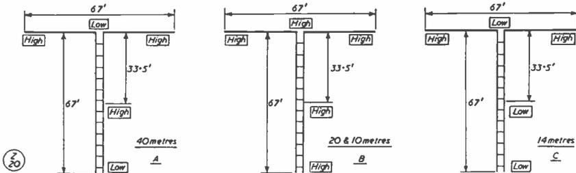
Fig. 2. A 67-foot wire, commonly used because it is one of the useful resonant lengths and within the space available at many amateur locations, with various modes of operation, as explained and discussed in the text.
