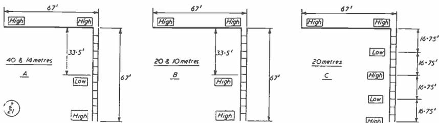
Fig. 3. This should be studied in relation to the system shown in Fig. 2. Here, the feeder arrangement is known as the "Zepp," and is widely used where it is more convenient to connect to one end of the "roof" rather than to the middle.
