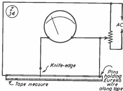
Fig. 8. Set-up used to calibrate the low AC voltage range.
