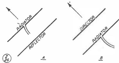
Fig. 8. Reflector and director systems, to give high gain in a particular direction. The principles are explained in the text.
