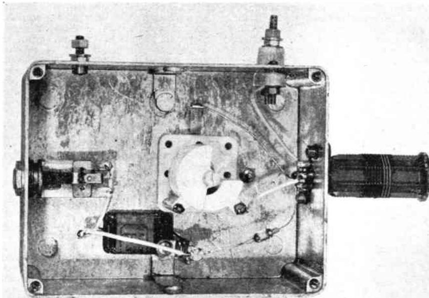
Interior construction of the Crystal Unit, showing layout and wiring — what could be simpler !
