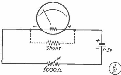
Fig. 5. Set-up for adjusting current-range shunts.
