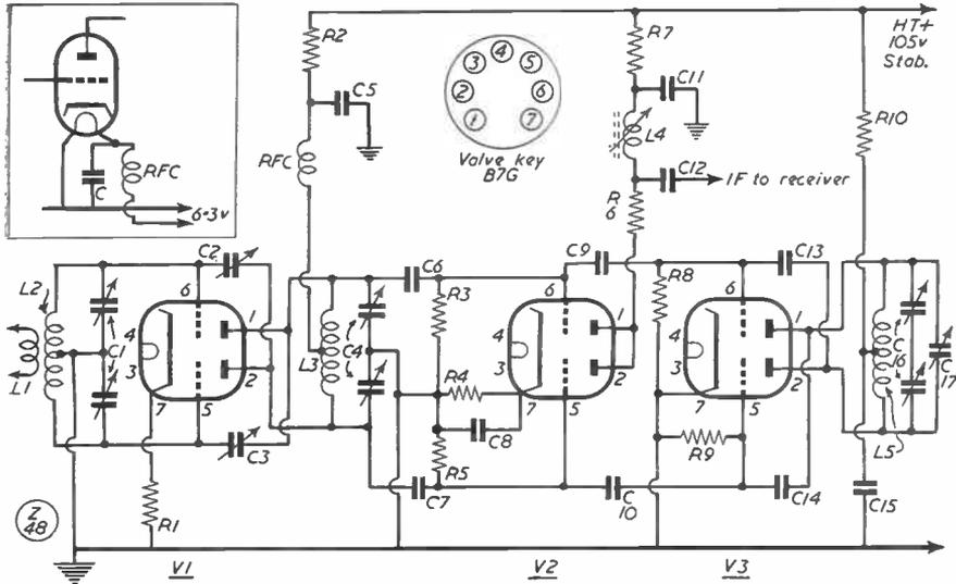
**Fig. 1.** Circuit of the two-metre converter using 6J6's, as described in detail in the article. The symmetry of the electrical layout should be noted — this should be translated into practice in the actual construction, of which one possible form appears at Fig. 2.
