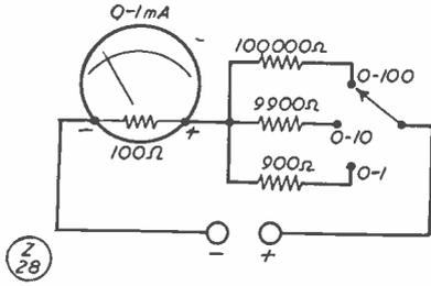
Fig. 1. Basic multi-range DC voltmeter.
