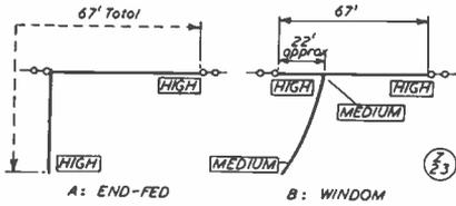
Fig. 5. Single-wire arrangements showing the distribution of impedance in two well-known types. In (A), the 67-foot wire as a whole is the aerial, and there is no feeder connection in the accepted sense; in (B), the feeder line is supposed not to radiate (or pick up) but nearly always does!
