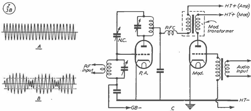
This sketch illustrates the answer to Question 1, sections A, B, C, being Figs. 1, 2 and 3 respectively. "A" is the unmodulated carrier, "B" a carrier wave with modulation on it, and "C" a suitable modulating circuit.
