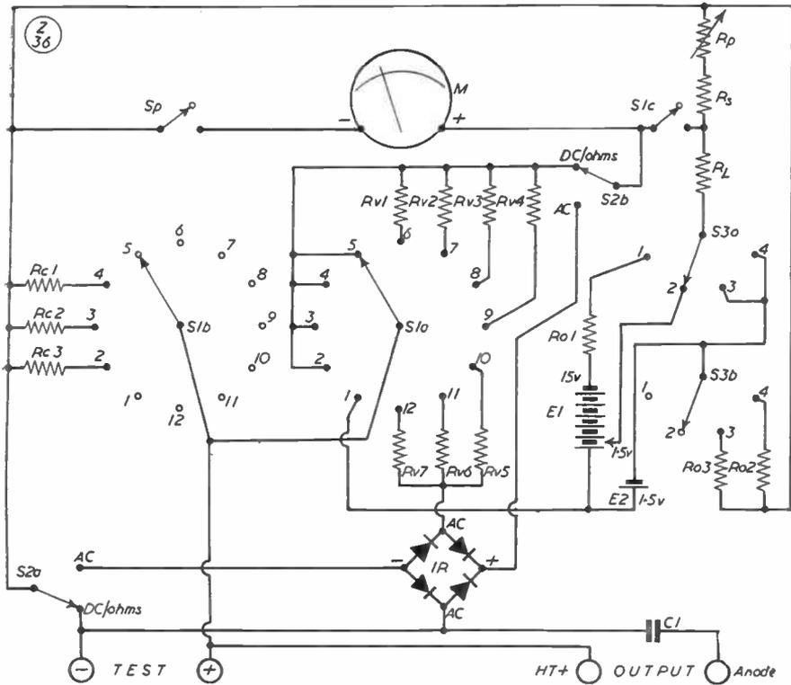
Fig. 10. Circuit covering all the possibilities discussed in the text, resulting in a very versatile instrument giving both AC and DC readings over a wide range, as well as resistance values.
