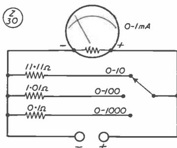
Fig. 3. Basic multi-range DC milliammeter.
