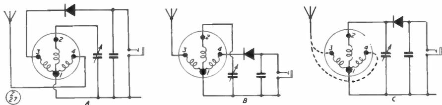
As explained in the text, results will vary according to which of the connections shown here is made. It is recommended that each be tried in turn to ascertain which works best with the particular aerial in use.
