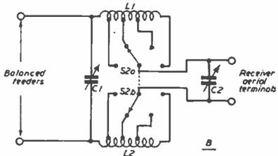
Circuits for the front-end tuner discussed in the text. An aerial coupler of this sort will nearly always give much improved results and is very desirable for serious DX work on the S/W bands.
