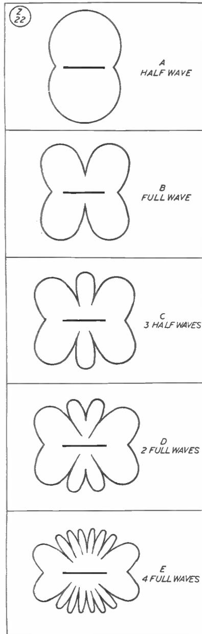
Fig. 4. Polar diagrams, or representations of the way in which energy is radiated by different types of aerials, giving rise to directional effects, as explained in the article.
