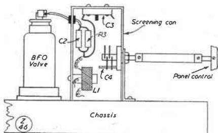
Fig. 4. In Fig. 3 is shown the circuitry for a useful BFO unit, external to the receiver, but for which space could usually be found on the average chassis. This sketch shows a suitable constructional layout.
