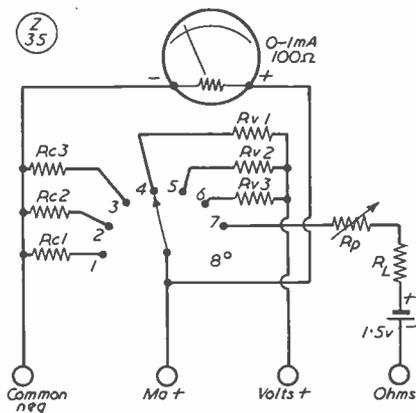
Fig. 9. Suitable Multi-Meter designed for many receiver tests. A more elaborate instrument is shown in Fig. 10.
