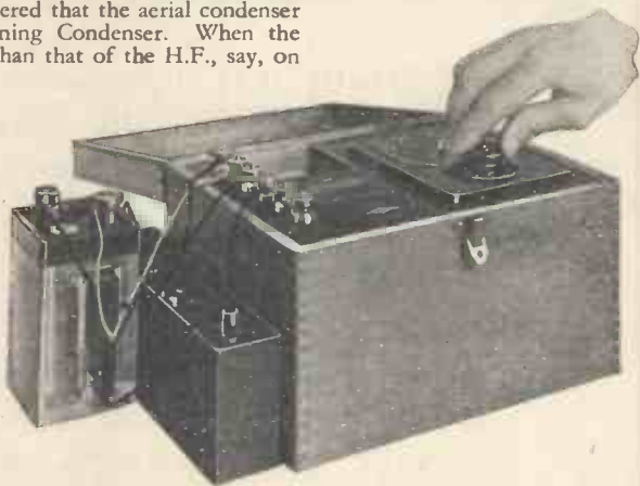
This illustration shows the Emerald Wavemeter, by the aid of which the identity of received stations was confirmed.
