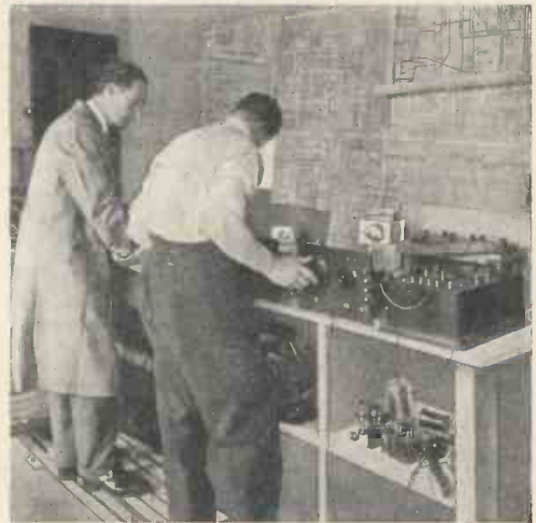
Checking up, stage by stage, the amplification of the experimental model of the Raleigh P.M. Receiver.
