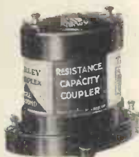
Showing the R.I. Varley R.C.C. Unit, the L.F. coupling referred to in this page.
