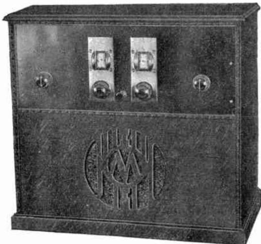
**A**n illustration of the new cabinet, designed especially for the new Mullard screened-grid receiver. The upper compartment contains the receiver, while the lower section houses the speaker, low-tension and high-tension batteries.
