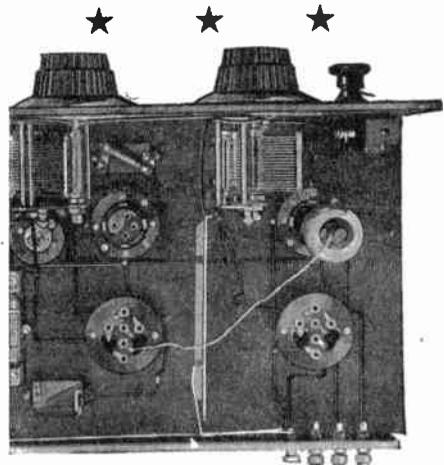
**A**N illustration of a reader's Mullard Nelson P.M. de Luxe converted to use a Mullard Screened-grid Valve.
