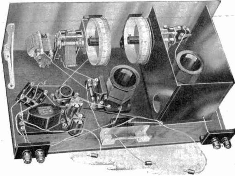
**A**S was the case with the previous Mullard Master Three Receivers, all battery leads are taken direct from the terminals of the components. Needless to suggest the method eliminates a number of rigid wires.
