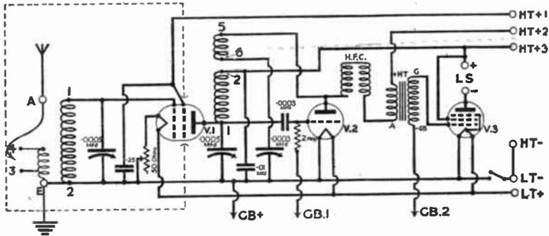
**A**BOVE is a circuit diagram of the Mullard S.G.P. Master Three. One of the main points in the design is the fact that selectivity may be adjusted for every individual case. This is effected by the suitable use of the alternative aerial taps, and in extreme cases, by a suitable modification of the aerial turn numbers.
