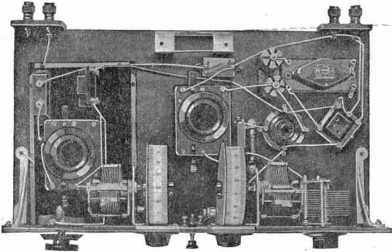
**A**n illustration of the combined-wave model, which, in conjunction with the "Wiring Step by Step," makes the assembly of the receiver an easy undertaking, even for those without any technical experience whatever. The disposition of the coils is clearly shown. They should be fixed to the baseboard in the manner described in the text.
