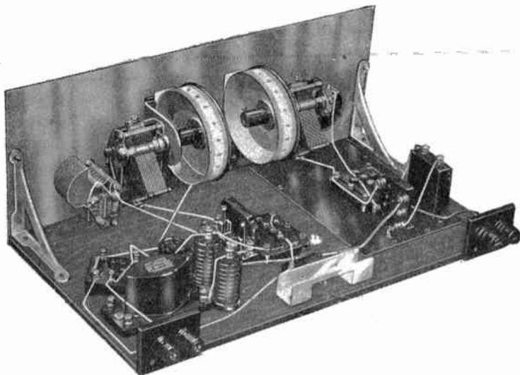
**A**NOTHER view of the receiver which provides a number of useful points to note during the construction. Connecting Links were actually used for the wiring-up of original receiver.
