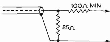
Fig. 4. Simple input pad for coaxial feeder. Attenuation through the circuit can be increased by using a larger value for the series resistor. This should never be less than 100 ohms, which is a fair average value.
