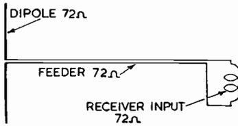
Fig. 1. Showing the elements of a television aerial system which must all be of the same impedance. Where twin balanced feeder is used, its impedance is somewhat higher (80 ohms).
