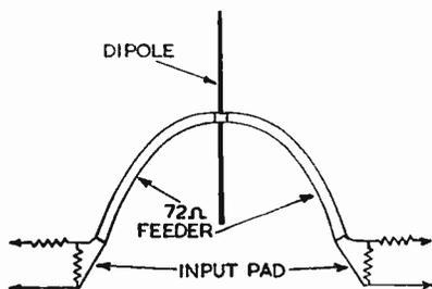
Fig. 5. Illustrating how the input pad of Fig. 4 can be used to terminate the feeders where two receivers are using the same dipole aerial.
