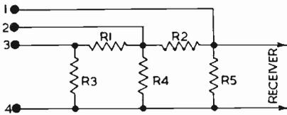
Fig. 3. A ladder attenuator made up of  $\pi$ -section networks. Good average values are 330 ohms (R1), 150 ohms (R2), 70 ohms (R3), 150 ohms (R4) and 100 ohms (R5). The common (outer) conductor is taken to position 4, the inner coaxial conductor being used at either of the other positions according to the ratio of attenuation required. Similar systems may be devised for twin feeder by using the appropriate basic networks.
