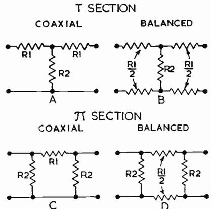
Fig. 2. Four basic types of attenuator networks as used for television purposes. These are fully discussed in the text. In examples A and C the outer conductor is taken to the lower leg of the network.
