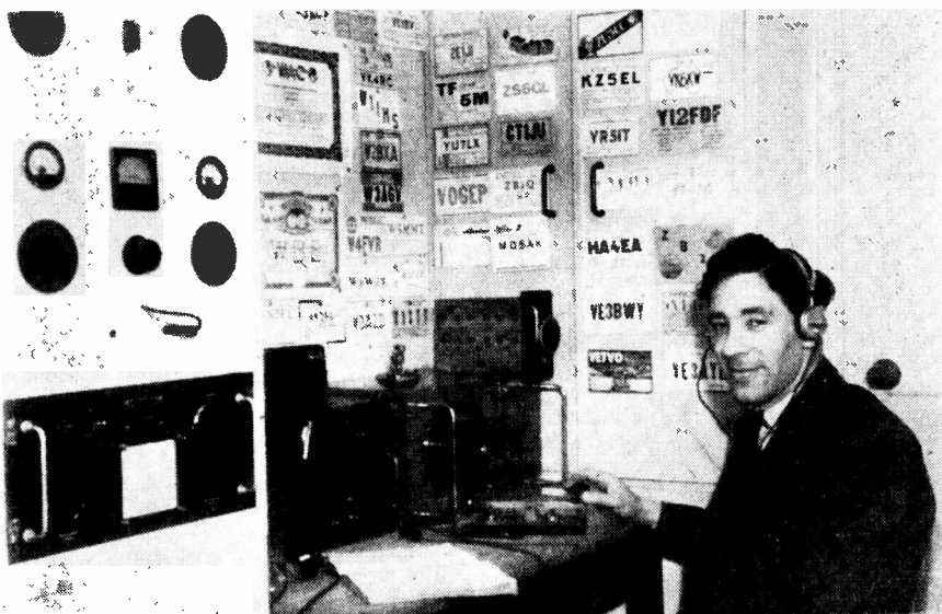
G5PQ, Hull, has the outfit in the kitchenette of his aluminium prefab, the gear occupying only 5-ft. by 2-ft. 6ins. of precious space. Of particular interest is the fact that he uses a ground plane aerial, as no poles are allowed. The score is 90 countries worked, using the full 150 watts into an 808 in the output stage.
