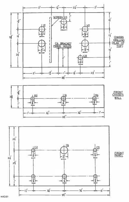
Fig. 2. DRILLING DIMENSIONS OF THE PANEL AND CHASSIS
