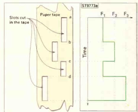
**Fig. 2: The solution, as subject to patent 2292387. This example allows the use of three discrete frequencies. The execution of the scheme was beyond the technologies of the day.**
