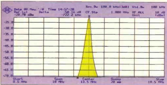
Fig. 2: AR88 pre-selector response 13.5MHz, -50dB bandwidth <1.5MHz.
