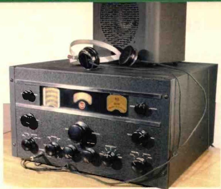
Selectivity in the AR88D is provided by having three i.f. amplifier stages embracing a total of twelve tuned circuits at 455kHz (735kHz in the AR88LF) and a single crystal filter. The crystal filter is not tunable from the front panel as in the case of receivers like the HRO, so keen c.w. operators would miss the 'single signal' razor sharp peaks and notches, but the design and alignment of the crystal filter is such that the resultant bandwidth is more or less symmetrical.
