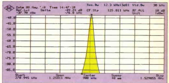
Fig. 4: AR88 pre-selector response 900kHz, 50dB bandwidth 150kHz.
