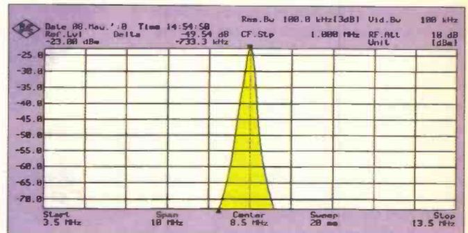
Fig. 3: AR88 pre-selector response 8.5MHz, -50dB bandwidth <1.5MHz.
