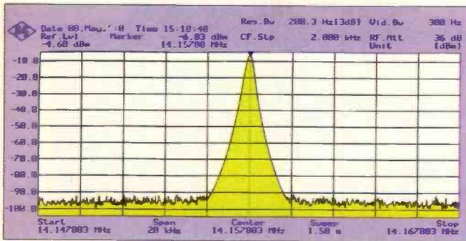
Fig. 1: AR88 local oscillator spectral purity.
