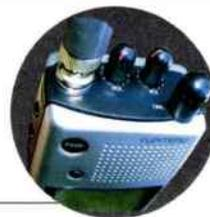
the click-step rotary knob on the top panel and a side mounted 'function' bar, these controls let you do all the usual things like select a frequency, program memory channels, adjust the channel step rate and so on. A further recessed green push button is used as the power switch, holding this down for a second or so acts as an on/off toggle switch.
