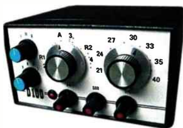
The D-100 DX-TV converter. An optional alarm is available to warn of a Sporadic-E opening.
