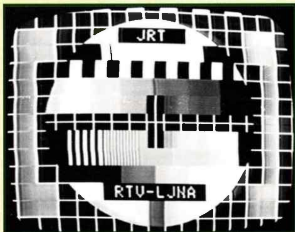
A Slovenian PM5544 test card on Channel E3 during a bout of stable reception. The PM5544 is currently used by Denmark, the Netherlands, Belgium, Latvia, Estonia, Slovenia, Hungary and Slovakia. A version of the test card featuring a digital clock insert is known as the PM5534; this is currently broadcast by Iceland, Norway, Sweden and Denmark.
