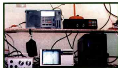
A DXer's shack with f.m. receiver, scanner, D-100 converter and two TV receivers.
