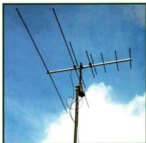
Mounted at only 5m, this compact antenna has received signals in Band I from the Middle East and Australia and Band III from Algeria, Tunisia and Libya.
