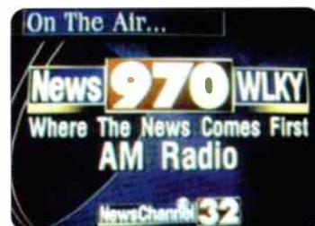
Fig. 2: WLKY Louisville, Kentucky, received on Channel A32 at around 330km by William Mitchell during tropospheric enhancement.
