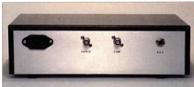
Interconnections to radio, computer, key and mains.
