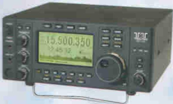
**RX-350:** The Ten-Tec RX-350 is a full featured, mid-price range HF DSP receiver. on-screen band activity display adds a new dimension to locating transmissions and tuning the receiver, 34 DSP bandwidths provided, noise reduction etc. Extensively reviewed by John Wilson, *SWM September 2002.* **£1,099 inc VAT\***
