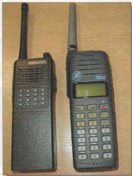
Two popular MPT1327 trunked radios. The radio on the left is a Kenwood TK-255 while the one on the right is a Tait T3000. The Tait's large display lets its users receive text messages just like a mobile phone.
