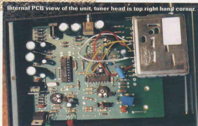
Internal PCB view of the unit, tuner head is top right hand corner.
