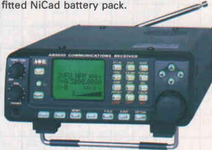
The upper **frequency range has been extended to 3000MHz (3.0GHz)**, lower band sensitivity has been increased (now officially covering to 100kHz) with an **enhancement to short wave performance** by the addition of further bandpass filters and revision to I.F. filters. **Mini-Circuits RMS1 / RMS2 mixers** have been employed with **active SPM aerial switching devices** (not diode-switching) abundantly employed throughout the signal path.
