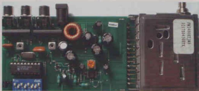
**Fig. 2: A 2.4GHz receiver card.**
