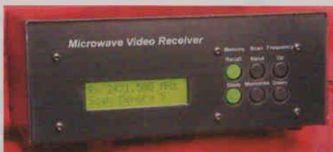
frequency ranges. The 13cm version reviewed here covers 2.2-2.7GHz (2200-2700MHz) and offers 10 memories, scanning functions, and superb frequency control. The 23cm version, which covers 800-1800MHz, offers similar facilities. I've only used the 13cm version so all my comments relate to that version.
