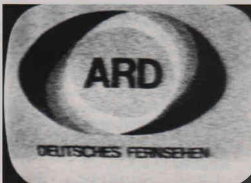
**Fig. 7: The German studio caption from ARD photographed on June 12th 1970 during a tropospheric opening. The signal was received on an indoor dipole from the WDR Langenburg transmitter which operates on Channel E9.**
