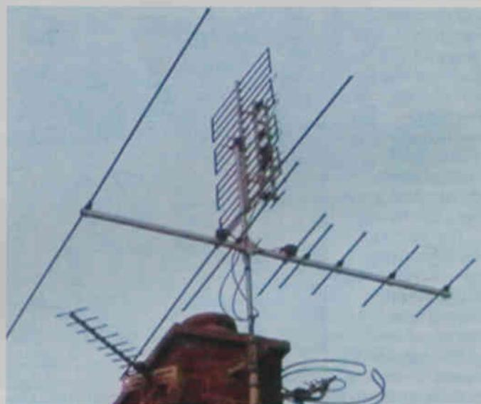
**Fig. 3: A chimney-mounted system featuring a wideband grid for u.h.f. DX-ing and an eight-element v.h.f. array for Bands I, II and III.**
