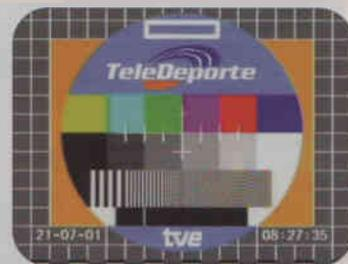
**Fig. 1: The Spanish GTE test card, which may still be used by TVGE in Equatorial Guinea, but bearing the appropriate identification.**
