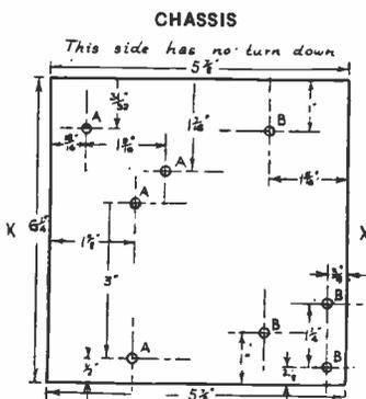
Tube Bracket and Chassis, 16 S.W.G. Aluminium.
