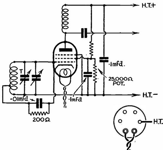
The cathode dial resistance and shunting condenser are fastened direct to the cathode pin and the wire from the other side passes through the hole (which is left vacant when fastening the coil base) to the cathode tap soldering tag on the base.
