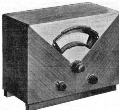
By the use of a carefully developed circuit arrangement, the two self-contained aerials and a powerful valve combination, having six separate functions, this receiver measuring only 11 in. x 12 in. x 8½ in. provides performance which is equal in sensitivity and quality of reproduction to instruments of standard size of similar type. The set weighs but a few pounds, is neat and compact, and with carrying handle, may be taken from room to room as required.
