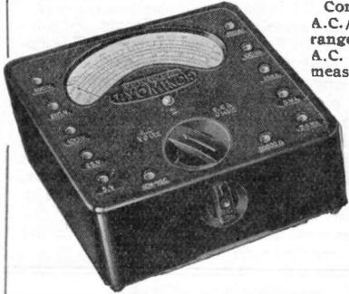
Compact multi-range A.C./D.C. meter, 22 ranges. Provides for A.C. and D.C. voltage measurements up to 500 volts; Current measurements up to 500 milliamps; Resistance measurements from 0-10 megohms; Highly accurate. Total resistance 800,000 ohms. Complete with leads, testing prods, crocodile clips, and instruction booklet.
