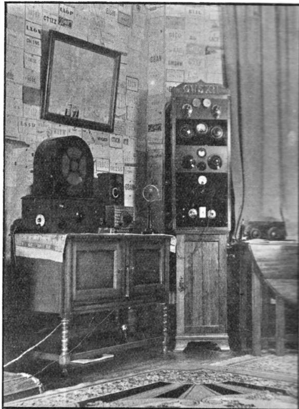
GW5XN has carried out a great deal of experimental work with aeriels, the most successful up to date being a 67-foot Windom link coupled to the PA. The aerial tuning network can be seen at the top of the rack, with the PA, doubler-CO, and modulator speech-amplifier stages in order underneath. The receiver is a straight 1-V-2, and a monitor and test set are also visible to the right on the operating table.
