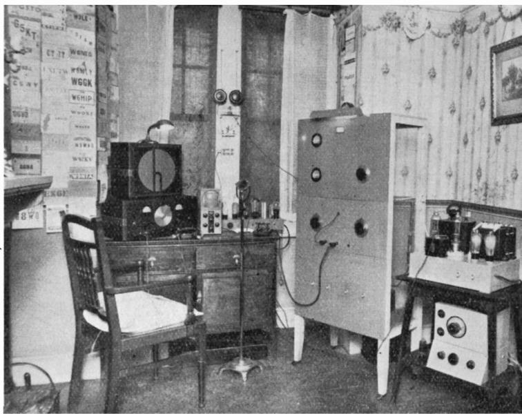
tioned pushes a pair of zero-bias 203Z's in a Class-B unit, giving about 300 watts of audio.
