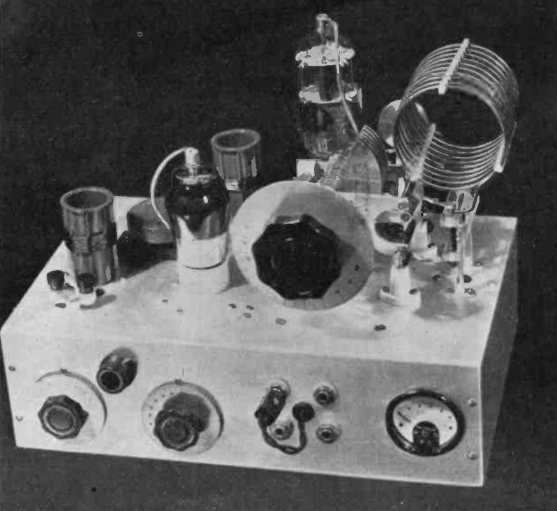
DESCRIBED AND ILLUSTRATED here is a two-stage transmitter which, called the "Two-Band-Two," can be operated on any frequency, including those used by the R.N.W.A.R. and C.W.R. Though 7 and 14 Mc working is discussed in detail, it is only a matter of selecting crystals and winding appropriate coils to get output on any band from 1.7 to 56 Mc.
