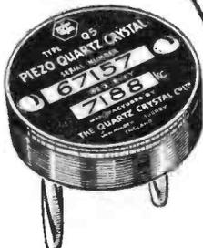
All units are ready mounted in the type U holder illustrated, and are supplied to within 5 kc. of your specified figure in the 1.7, 3.5 and 7 Mc. bands. The actual frequency is given on the Frequency Certificate to an accuracy of 0.025 per cent.
