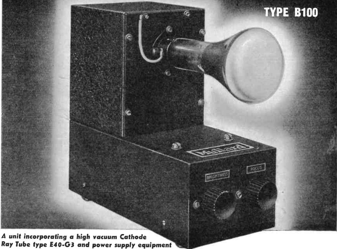
A unit incorporating a high vacuum Cathode Ray Tube type E40-G3 and power supply equipment
