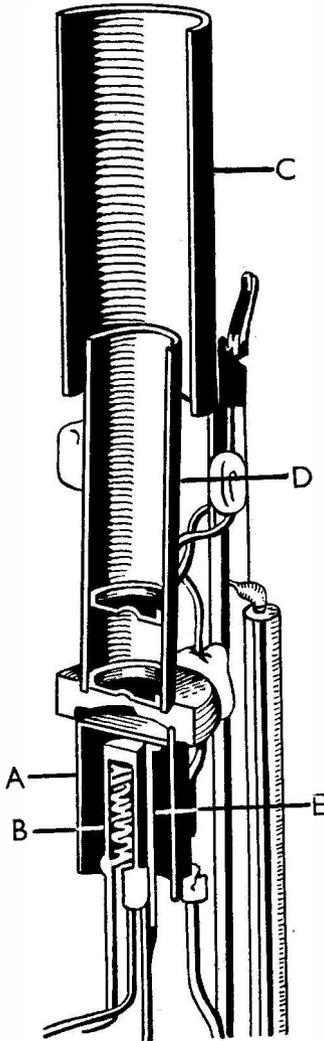
A—Grid. B—Heater. C—Anode 2.
