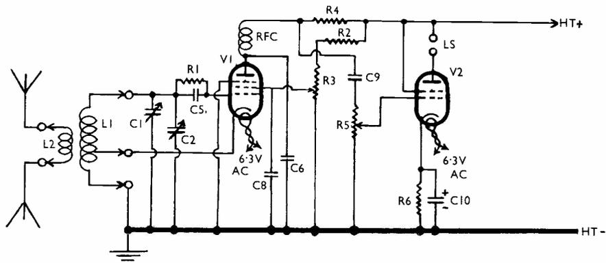
Fig. 4. A two-valve mains-operated receiver, with electron-coupled reaction circuit and band-spread tuning. The circuit of a mains power unit for this receiver is given in Fig. 5.
