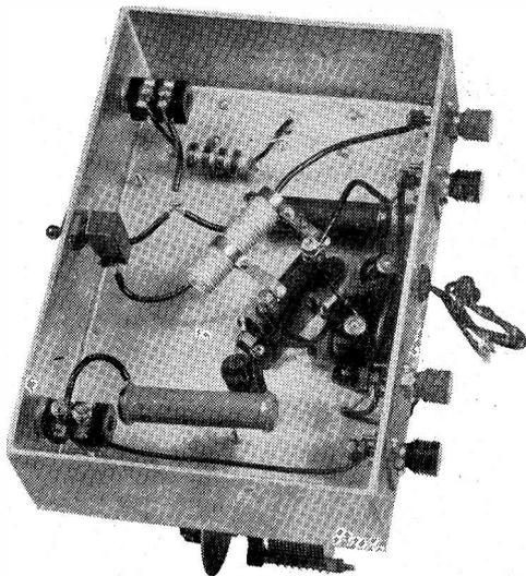
The FD sub-space. An additional terminal strip is provided to bring in the bias, and the cathode resistor is soldered across its by-pass condenser.
