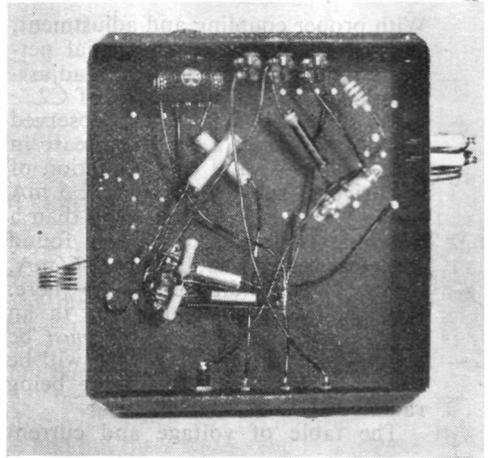
Underneath the PA chassis. Note how the return leads that matter are bunched to one point for soldering. R1, R2 and R5 are supported in the wiring; R3 is represented by the mounted resistor which has an additional 10,000 ohms in series to make up the full value required.
