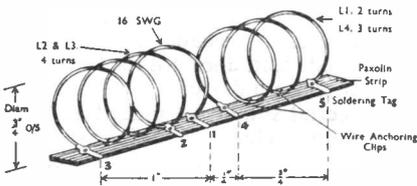
Fig. 4. Coil details for 58 mc receiver of type shown in Fig. 3.
