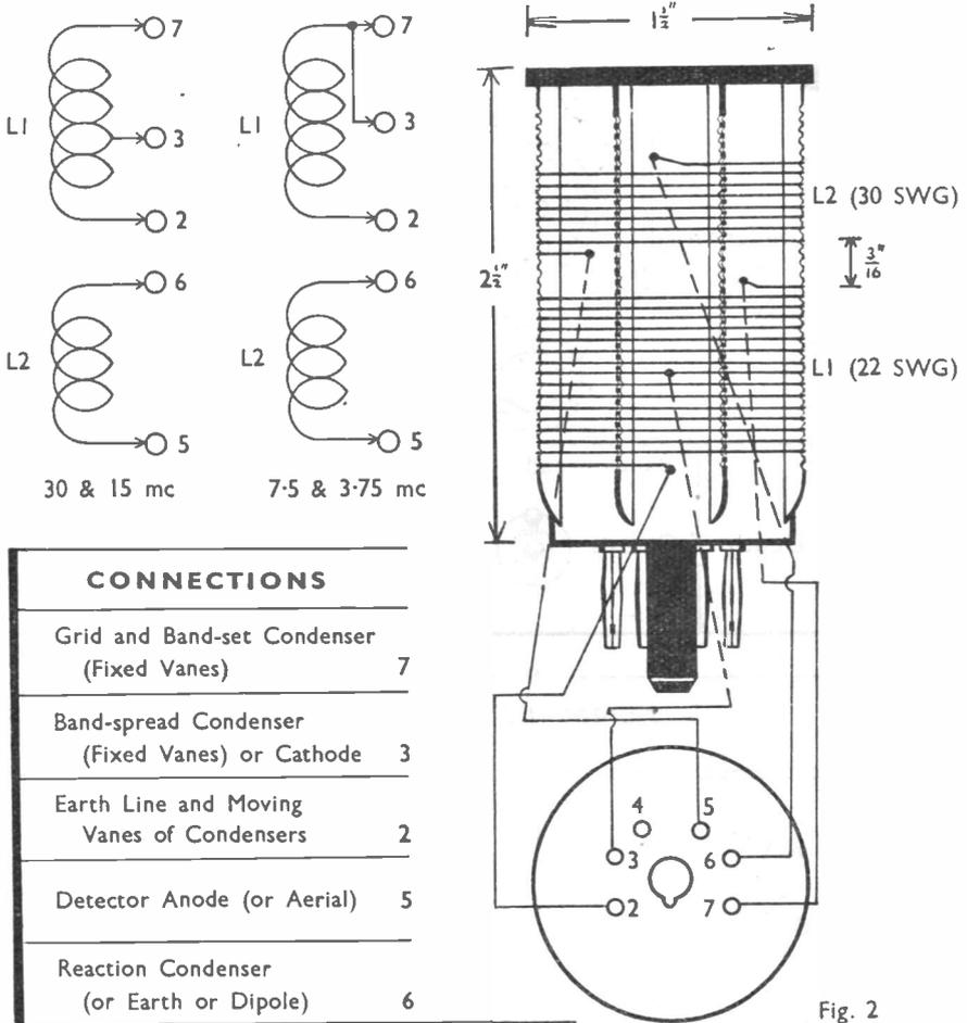
Fig. 2. Constructional details of octal-base six-pin coils suitable for short wave bands between 3 and 30 mc. Base connections shown are as seen when looking at the coil base or under side of the holder. Note that turns of L1 on all except 3.75 mc coil are spaced to fill a length of 1 1/2 in. on the former. For the 3.75 mc coil, L1 is close-wound, as they are for L2 on all ranges.
