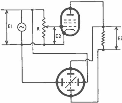
Fig. 12. Circuit arrangement for measuring the amplification of a valve.
