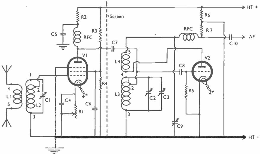
Fig. 3. A good circuit for the RF and detector stages of a simple 58 mc receiver.
