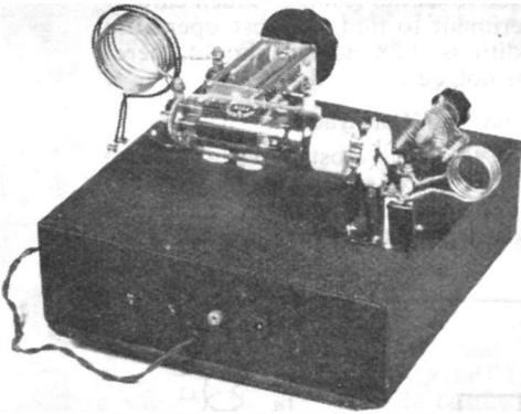
A view of the amplifier showing the construction at the grid end of the PT15. Note the grid coil mounting; fixed condenser C3 is to the right and one side of C6 goes directly to the screen terminal of the valveholder.
