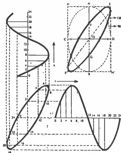
Fig. 9. Diagram showing the formation of an ellipse from two sine waves out of phase and of different amplitude.
