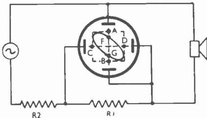
Fig. 10. Diagram of circuit used for measuring the impedance of loudspeakers or output transformers.
