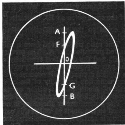
Fig. 11. Diagram of image on cathode-ray tube from which impedance and phase angle measurements may be taken.
