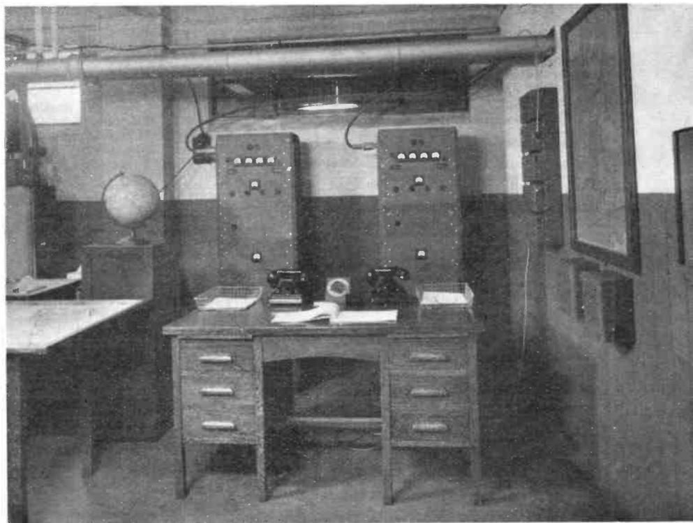
Layout of the Headquarters Station for the Radiophone Mobile Control System developed by Eddystone. This enables constant two-way contact to be maintained with police patrol cars, fire tenders and floats, and in other services where speedy mobile point-to-point communication is essential. The transmitter, with an aerial power of 100 watts, is VFO switched, and the frequency can be set anywhere within the limits 40-150 mc.
