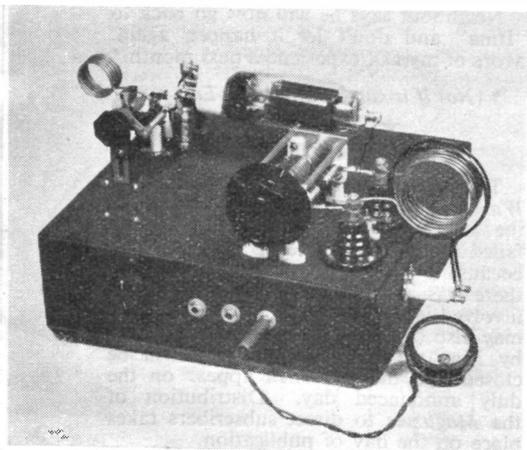
HT, and it is in any case most undesirable to allow the possibility of any stray external coupling between suppressor grid and plate, the suppressor HT should be separately supplied. In the model it was convenient to do this from a source which happens to give 360 volts. As the suppressor voltage should be set at +40 volts, the potentiometer-resistor combination R4, R5, was provided for the purpose. It
