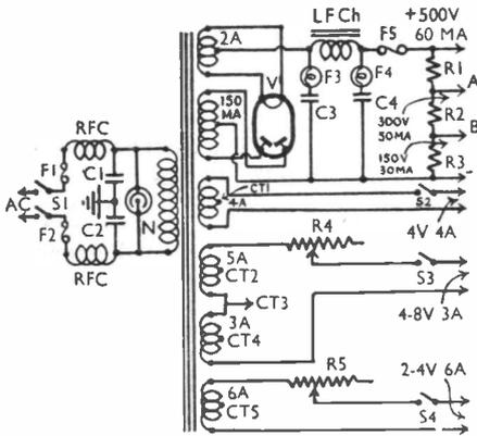
A complete wiring diagram of a suitable unit is shown in Fig. 2. Note that, as in Fig. 1, an RF filter is incorporated, as with certain transmitter arrangements and types of aerial coupling, there is a tendency for RF to get back to the power supply and so into the mains, causing unnecessary and avoidable BCL interference. The
