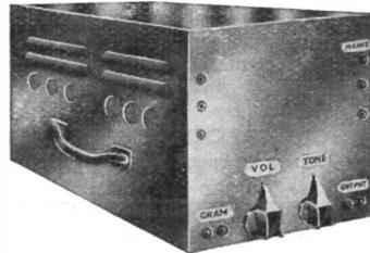
A small compact amplifier, using 6F6's in push-pull,
