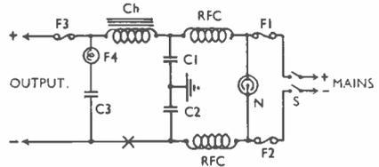
Fig. 1 shows the arrangement of a DC mains filter, delivering a hum- and ripple-free PDC supply and preventing RF feedback from the transmitter into the mains.
