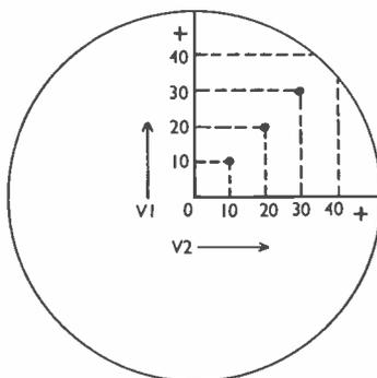
Fig. 7. Showing spot displacement due to equal values of DC voltages between horizontal and vertical plates.
