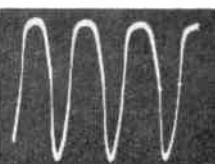
Fig. 33. Oscillogram obtained from a receiver operating under incorrect conditions.
