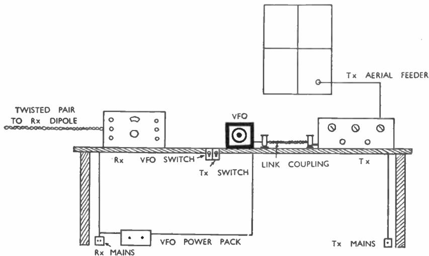
Fig. 4. Suggested internal station layout for using the VFO. Obviously, many variants of this arrangement are possible.
