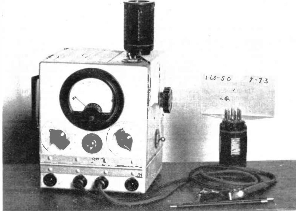
**GSBY's V.O.M.-Frequency Meter.** General view of an instrument covering 1-35 mc, and giving readings up to 5,000 volts, with current scales to 1,000 mA and resistance readings to 500,000 ohms.
