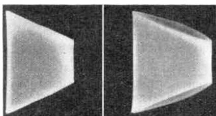
Fig. 28. Oscillogram of Fig. 29. This figure is a signal with 38 per cent. modulation recorded without a time base.
