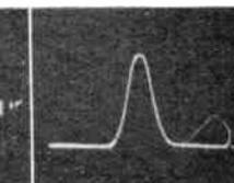
Fig. 41. A resonance curve with somewhat wider band width than Fig. 40.
