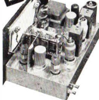
A high performance 6-valve A.C. Superhet covering 880 Kcs to 34 Mcs (9 to 345 metres) in 5 bands, having an EF 50 high-mu low noise RF stage.
