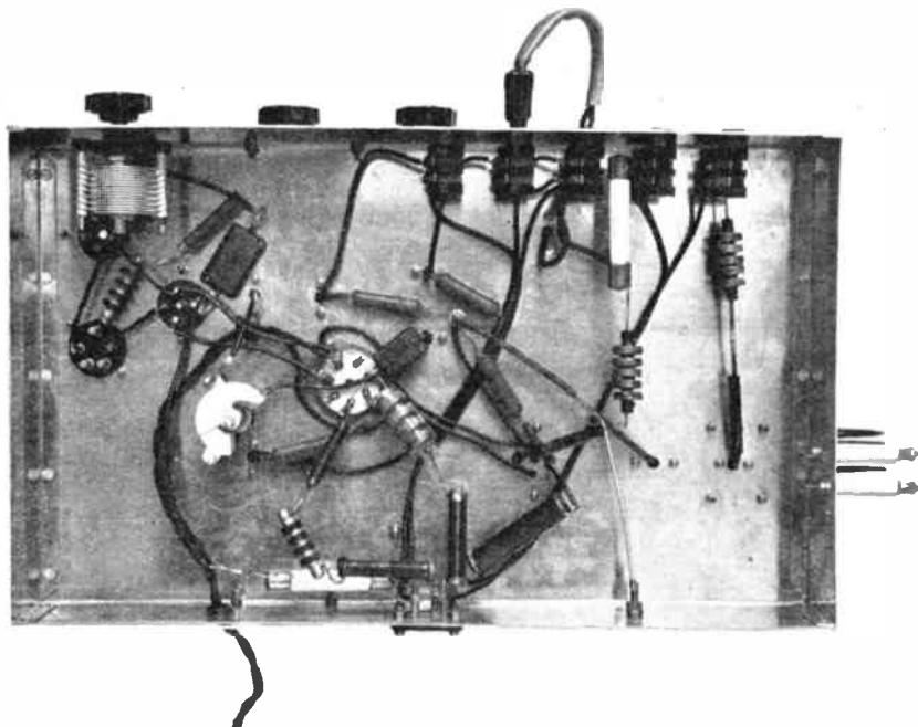
The chassis sub-space. All components, and practically every connection, can be seen. Note the small 58 mc RF chokes in series with the larger chokes at the 58 mc end of the transmitter. The large ceramic valve-holder is for V2, across the heater pins of which LT is fed for all three valves. Connections made through holes in the chassis are sleeved. The sub-space is 3 in. deep, and the chassis is 17 in. long by 10 in. wide
