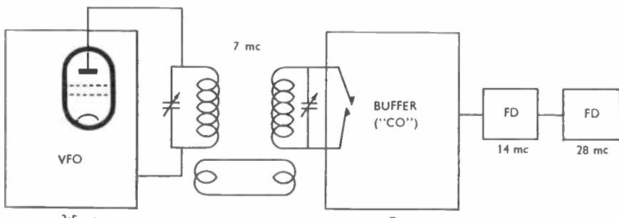
Fig. 2. Block diagram showing tuning sequence with VFO on 3.5 mc. The 7 mc CO becomes a buffer-doubler when, with the crystal removed, it is driven from the VFO. If the original CO was operated on the fundamental of the crystal, the buffer will have to be neutralised unless it is a tetrode or pentode in a stable, well laid out circuit.
