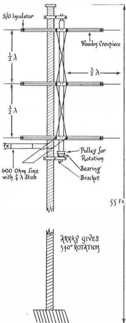
Diagram gives main details of the six- $\frac{1}{2}$ -wave-in-phase vertically stacked 58 mc aerial at G6CW (Nottingham). All elements are  $\frac{1}{2}$ wave long, with  $\frac{1}{2}$ wave separation, and fed through a 600-ohm line across a  $\frac{1}{2}$ -wave matching stub at the base of the array. G6CW credits this aerial with his recent successes on 5 metres.
