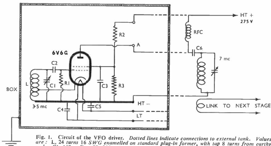
Fig. 1. Circuit of the VFO driver. Dotted lines indicate connections to external tank. Values are : L, 24 turns 16 SWG enamelled on standard plug-in former, with tap 8 turns from earthy end ; C1, 160  $\mu\text{F}$ ; C2, 200 $\mu\text{F}$ ; C3, C4, C5, .01  $\mu\text{F}$ ; C6, .001  $\mu\text{F}$ ; R1, 100,000 ohms, 1 watt ; R2, 50,000 ohms, 1 watt ; R3, 20,000 ohms, 1 watt.
