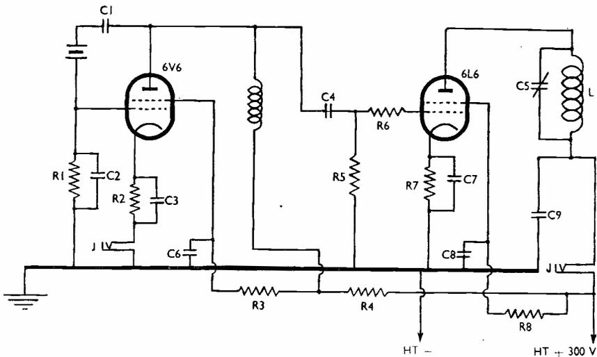
Fig. 2. The same circuit adapted for the use of the commoner 6V6 and 6L6 types in the CO and PA positions. All values for both circuits are given in the table.
