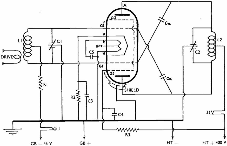
Fig. 1. Circuit around the QVO4-20, connected in push-pull. The neutralising wires in the photograph are represented by  $C_n$ . The electrodes are marked for reference to the valve base connection diagram, given at Fig. 2. Suitable RF chokes in series with the grid and plate coil centre-taps might improve balance. Heaters can be connected either in series (12.6 volts) or parallel (6.3 volts).
