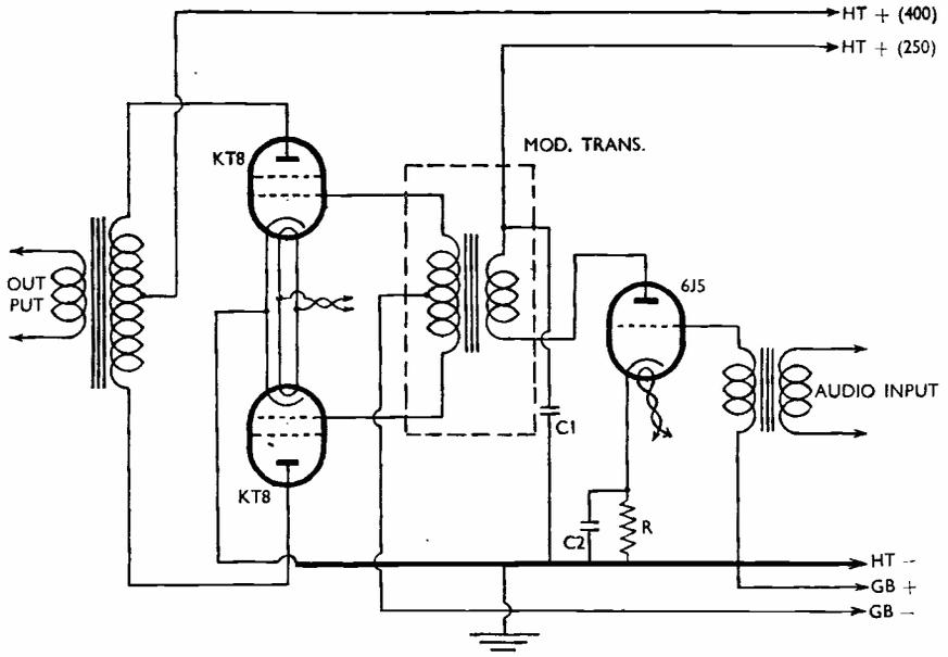
Fig. 1. A Class-B modulator. It will give sufficient output to control a 100-watt carrier. In this circuit, C1 can be  $4 \mu\text{F}$ , C2  $8 \mu\text{F}$ , and R 1,000 ohms. The screen connection should be made by strapping them together, by-passing to earth with a  $8 \mu\text{F}$  400-volt DC working condenser, and feeding through a 2000-ohm 10-watt resistor connected to the HT positive line.
