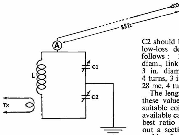
**The Matched End-On aerial coupler.** C1, C2, should be  $\cdot 0005 \mu\text{F}$  for all-band operation 1.8-28 mc, or  $\cdot 0002 \mu\text{F}$  for 7 mc upwards. The system will also take power very effectively on 58 mc with smaller condensers and careful adjustment. Coil details are given in the text. A is an aerial ammeter, either hot-wire or thermo-couple; a 5- or 6-volt bulb taking about 1 amp. will do it a meter is not available.
