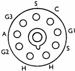
Fig. 1. Base connections of the EF-50. H, H, heater, C cathode, G1 control grid, G2 screen grid, G3 suppressor grid, A anode, S valve screen.
