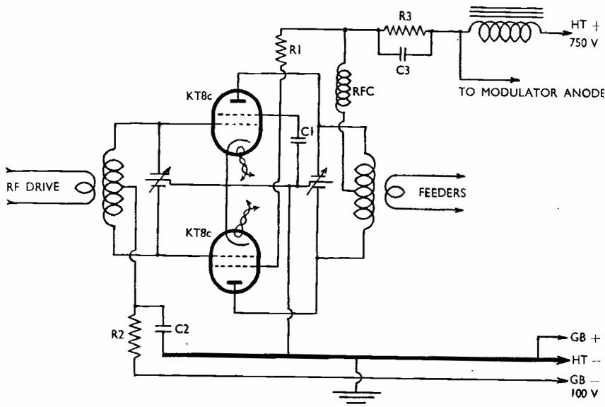
Fig. 2. Plate-and-screen modulation of a pair of tetrodes (KT8c's or 807's) in Class-C push-pull. Under the circuit conditions given, they will require about 10 mA drive. Values are: R1, 30,000 ohms, 3 watt; R2, 25,000 ohms, 2 watt; R3, 1,000 ohms, 40 watt; C1, .001  $\mu$ F, 600-volt DC working; C2, .002  $\mu$ F, 250-volt DC working; C3, 8  $\mu$ F, 250-volt DC working.
