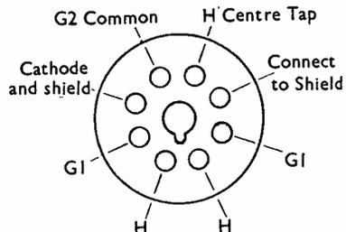
Fig. 2. Base connections for the QVO4-20.
