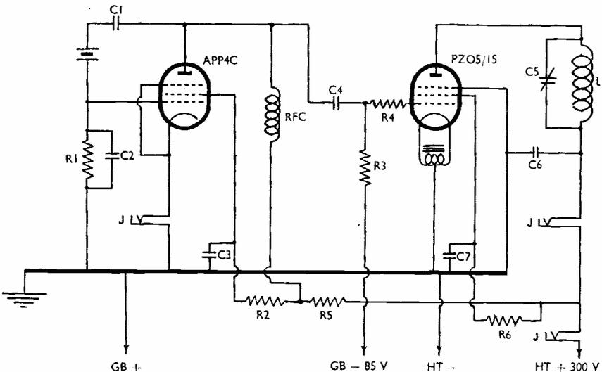
Fig. 1. Circuit of G6KR's 1.8 mc CO-PA. A simple arrangement, capable of giving excellent results. The CO is a Pierce oscillator. The PZO5/15 PA is a filament-type valve; its cathode return can be made at the heater winding centre-tap.
