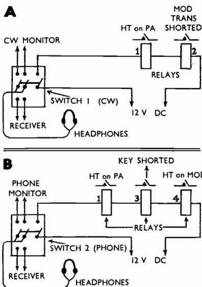
(A) is the wiring of the CW switch, (B) is for the Telephony change-over. Though four relays are shown, the operations in (A) and (B) could be performed by two relays only: One having three pairs of contacts (1, 3, 4, in B) and the other two pairs (1, 2, in A).
