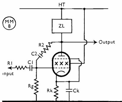
Fig. 3. Anode follower using cathode bias.
