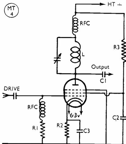
Fig. 3. A suitable frequency-multiplier circuit using the EF50.
