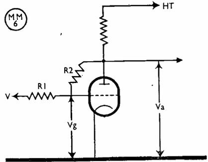
Fig. 1. The basic circuit.
