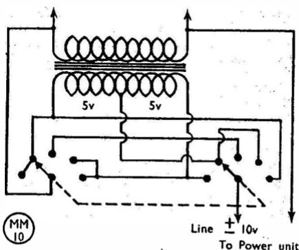
Fig. 2. The same idea adapted to give a plus or minus variation of line voltage.
