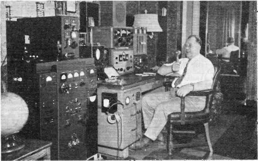
Clearly, VE3BKL of Merriton, Ontario, has practically 'everything'! The transmitter is a BC-610 running just the half-kilowatt input, and receivers are a Super Pro and SX-28A.
