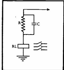
Fig. 6. Idea by P. H. Alderson. The 150,000-ohm resistor R limits the operating current for the relay RL.
