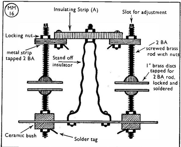
Fig. 2. Idea by G8TT for the construction of a push-pull neutralising condenser. The sketch is self-explanatory, the parts are mainly junk-box, and the important point to watch is the use of good insulating material for the bridging strip (A).
