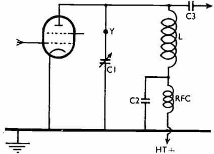
Fig. 3. Series-parallel feed, the modification suggested by G5UM. C1/L are electrically in parallel via C2, and the circuit tunes quite normally. One side of C1 can be earthed and the DC voltage across it removed by inserting an additional series condenser at Y. It is necessary to provide a good RF path from C1 through C2 to L, since the RF circulating current flows in this part of the circuit.
