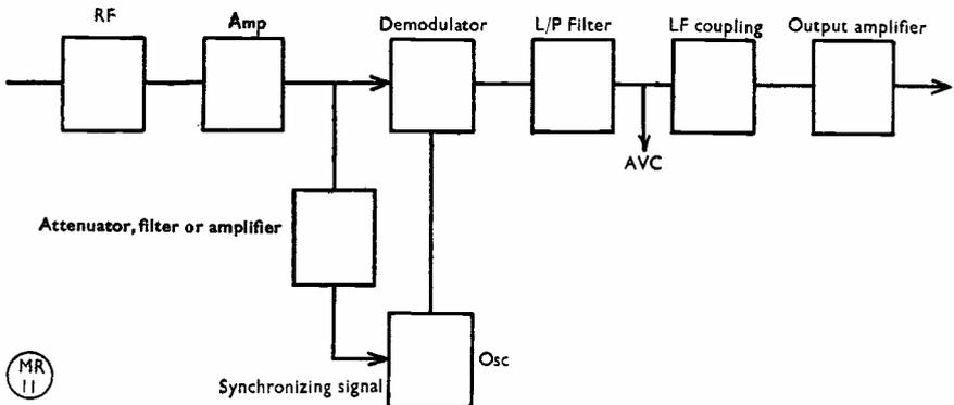
Fig. 1. Block schematic of the circuit arrangement. The attenuator-filter-amplifier element in the synchronising circuit may not be required in certain cases.
