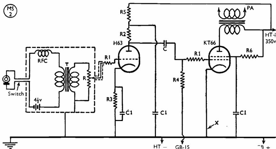
Fig. 2. Circuit of the modulator. A carbon microphone is shown, for which one stage of speech amplification (H63) is sufficient. This would not give enough gain with a crystal microphone, for which an additional stage (and some re-design) would be necessary. If self-bias is desired, a 3-watt resistor of 170 ohms, by-passed with  $25 \mu\text{F}$ , can be inserted at the point "X" in the cathode lead of the KT66.
