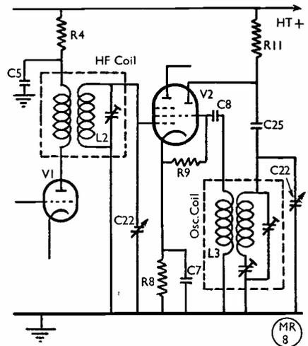
Fig. 2. Alterations to the circuitry around V1 and V2. Note the  $100 \mu\text{F}$  condenser C25, inserted in the oscillator plate lead as a precaution against trimmer or padder condenser shorting on L3.
