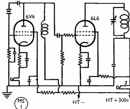
Fig. 1. The circuit of the original CO/PA, as described in the August issue. For anode-and-screen modulation of the 6L6, it is essential that jack J be wired as shown. The modulator circuit is given in Fig. 2. Cathode control can be applied by breaking the cathode of the 6L6 and connecting the modulator output across the break.
