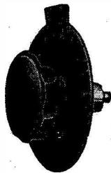
Slow-motion Dial, with Vernier reading device, 3½ in. scale and large fluted instrument knob. Reduction ratio 10-1. Matt Black with White fillings.
