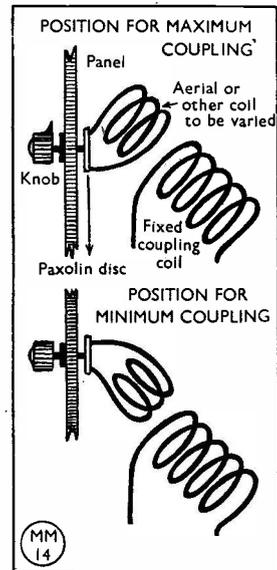
Fig. 5. R. A. Bernard's method of obtaining panel-controlled variable coupling. With extension rods, it could be applied to transmitter links.
