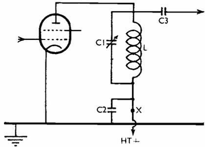
Fig. 1. Standard series-feed circuit. An RF choke is sometimes inserted at X, but is not essential. In this circuit, both sides of C1 must be well insulated.
