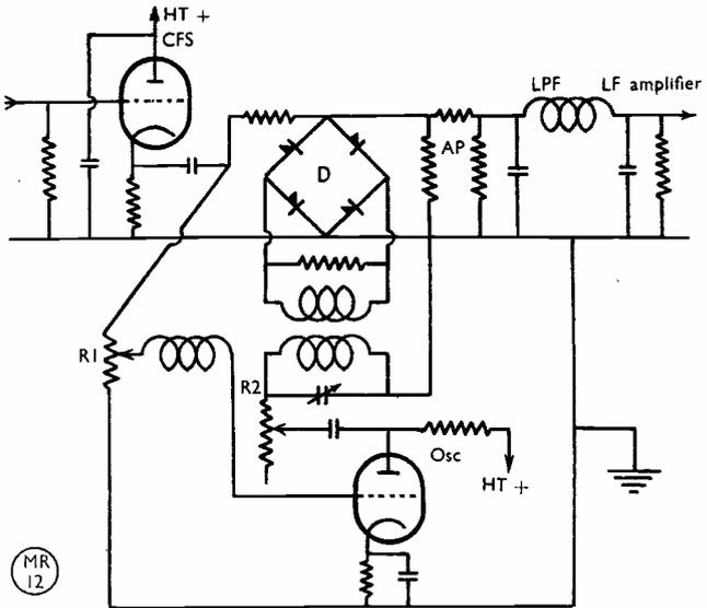
Fig. 2. A practical circuit, which gave the results described in the text. CFS is a cathode-follower stage, D the demodulator, AP a small attenuator pad, LPF the low-pass filter, and Osc the oscillator. R1/R2 are pre-set and adjustment for volume is on the oscillator tuning condenser.
