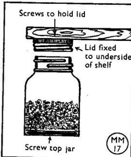
Fig. 4. G5WC has a series of screw-top jars for holding small parts. The lids are fixed by screws to the underside of a shelf and the jars screwed into the lids.
