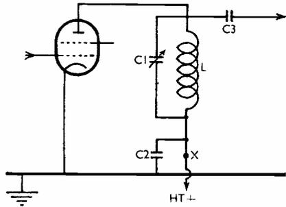
Fig. 1. Standard series-feed circuit. An RF choke is sometimes inserted at X, but is not essential. In this circuit, both sides of C1 must be well insulated.
