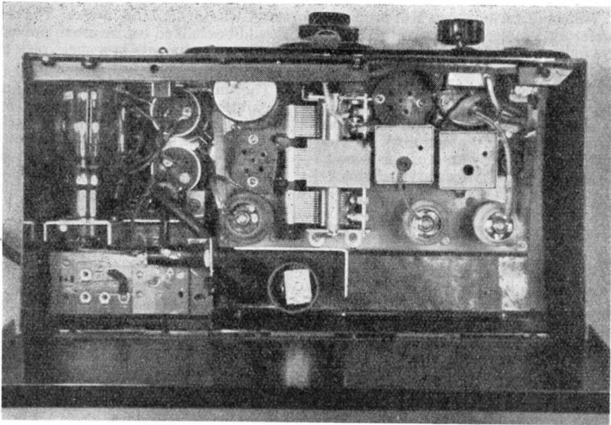
Looking into the receiver as modified. Rectifier valve on left, V1 in the first can at top with V2 in line below and the RF coil socket between them, aerial coil socket to the top right, and oscillator coil behind the screen along the lower edge. The space to the right of this screen could be used for an additional output stage.
