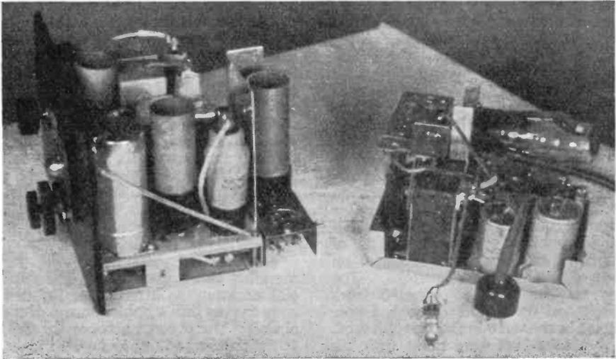
The receiver chassis and, on right, the power unit. The small extension to the chassis, as described in the text, can be seen with the meta screening for the oscillator.
