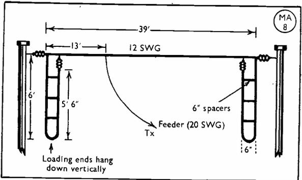
Fig. 1. Due to space considerations, G3SN uses a folded  $\frac{1}{2}$ -wave aerial for 7 mc. The system loads up well and can be made to resonate correctly; there is no radiation off the folded end sections.
