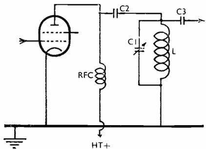
Fig. 2. The normal parallel-feed arrangement. The RF choke becomes a vital factor and C2 must withstand the HT. But one side of C1 is earthed, easing the constructional problem where a metal chassis is used.
