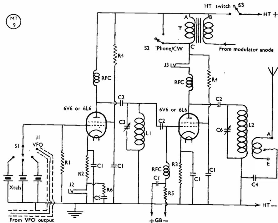
Fig. 1. Circuit of the RF portion of a simple CO/PA., with provision for modulation.
