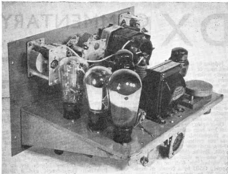
RF and audio sections can be accommodated together on the chassis-panel assembly. The three valves in line in the foreground are AC/HL-41MP-DO24 for the speech amplifier/modulator, with the PA just behind and the CO to the right rear.
