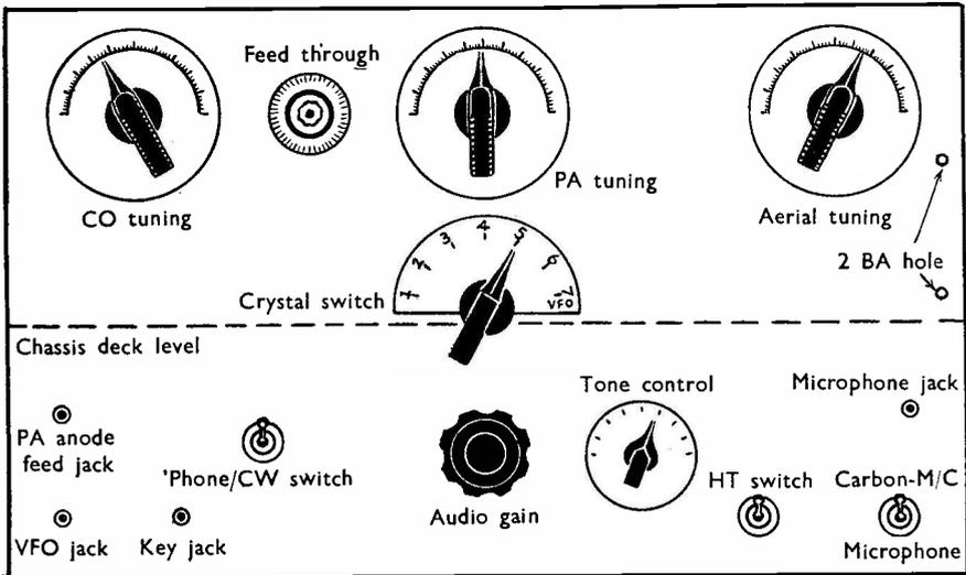
Fig. 4. Suggested panel layout for the CO/PA transmitter and modulator.
