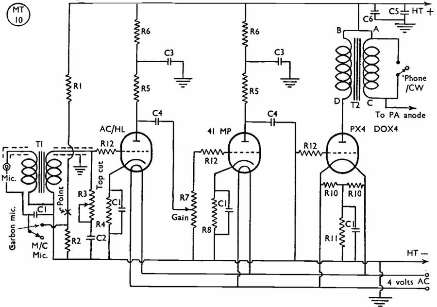
Fig. 2. A three-stage modulator for the CO/PA. The input circuit is arranged for either a carbon or a moving-coil microphone; the input leads should be shielded. For "DOX4" above read DO24.
