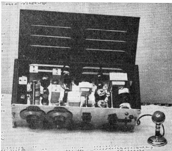
HB9CD has a nice driver unit for his P/P T55 RF amplifier. This end of the job is what he uses on 58 mc.
