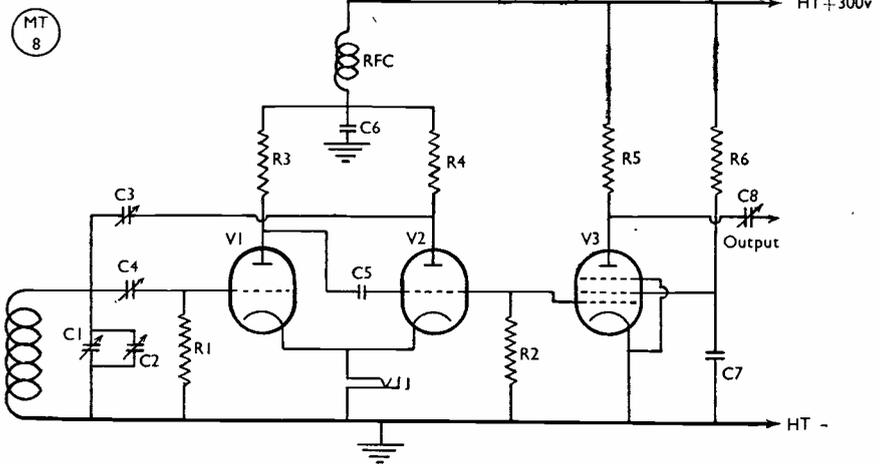
Circuit of the "T9x" Franklin Oscillator and Buffer.
