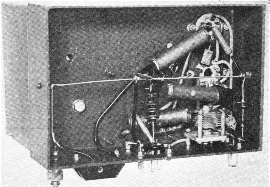
Under-chassis view of the Oscillator Buffer unit, showing wiring detail.
