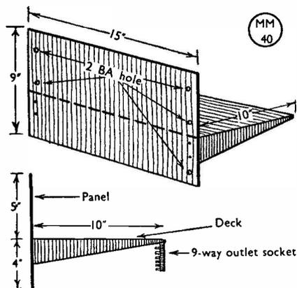
Fig. 3. Chassis-panel dimensions as used by GSUM for this transmitter.
