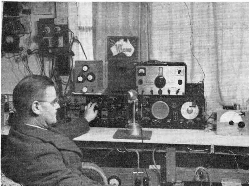
Operating position at VK2NO, Sydney, N.S.W., with OM Don Knock himself in the chair. To the right is the 28/50 mc converter, used with the Philips R163 to its left. The Rx on tune is an Australian Army No. 4 set, and above is a hand-switched pre-selector for 3.5, 7, 14 and 28 mc. VK2NO will be remembered in this country as G6XG of the early days.
