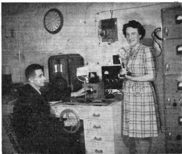
Here is an impression of ZL3AW, H. O. Hills, Kaiapoi, New Zealand, an amateur station conforming to modern standards of design and construction. In the rack-panel transmitter, units are so arranged as to draw out without having to fiddle with wiring at the rear of the assembly, as plugs are fitted behind all trays for making connections.
