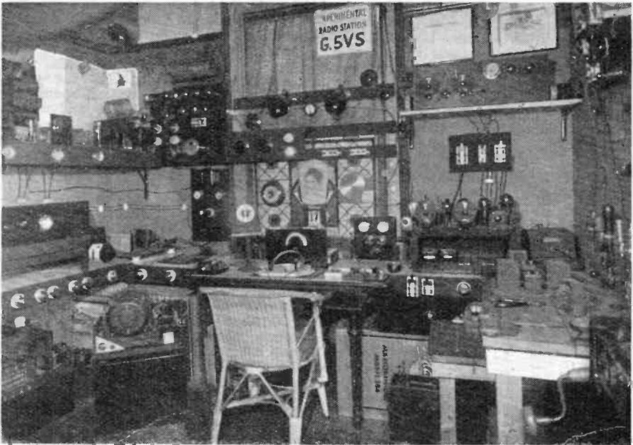
Another old-timer rig—G5VS, of Southend-on-Sea, Essex. The *Wireless World* of April, 1931, described this as the photograph of an "unusually ambitious amateur radio installation." The CC Tx ran DESB-LSSB-LSSB-P650 and the Rx was an 0-V-1.
