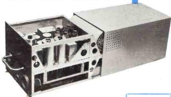
A pre-set frequency I.F. unit complete with 10 valves and power unit in wooden transit case, new and unused. Chock-full of components. Part of the transmitter receiver TRI366.
