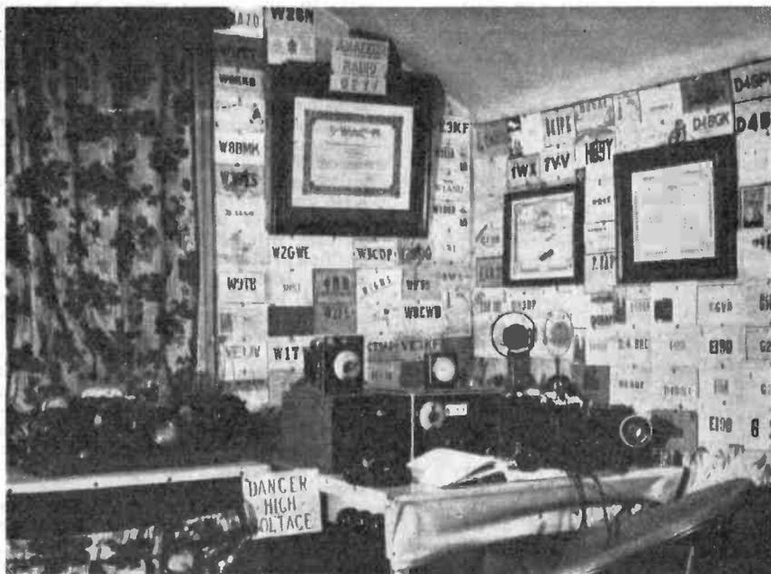
G2VV, Hampton-on-Thames, in 1934. The Tx was TPTG, with a 68-ft. end-fed aerial, and 25 watts into a Mullard TZO5-20. The Rx was 0-V-1.
