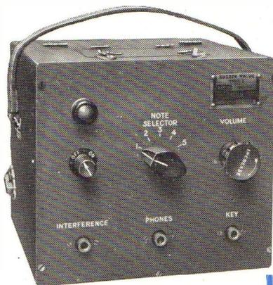
Incorporates note selector control, volume control, phone, key and interference jacks. Size 9" x 8" x 8½". Power supply required HT 60v. GB 4½v. LT 2v. Provision for these inside cabinet. Unit as illustrated, 15/-. Complete with 2 valves, types PMILF and LP2, 27/-. Pair of HR or LR phones (only if supplied with unit), 5/-. Heavy duty morse key, 2/6. Transit case, 2/6. A complete kit as described above, 32/-. **AS USED FOR R.A.F. TRAINING.**
