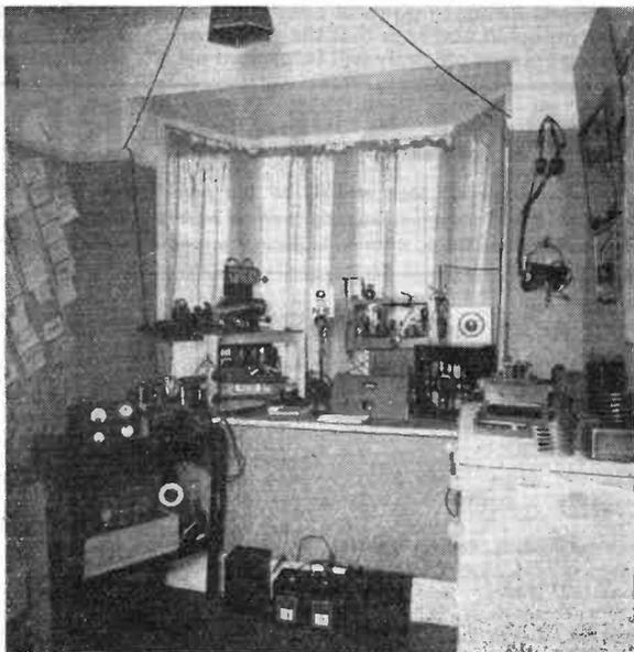
Another old timer outfit—G2NS in 1933. He ran a crystal-controlled SP55R-SP55R-LSSB transmitter, with an AR4100-PT25 modulator; the receiver was the ubiquitous 1-V-1, using PM12-HL210-PM22.
