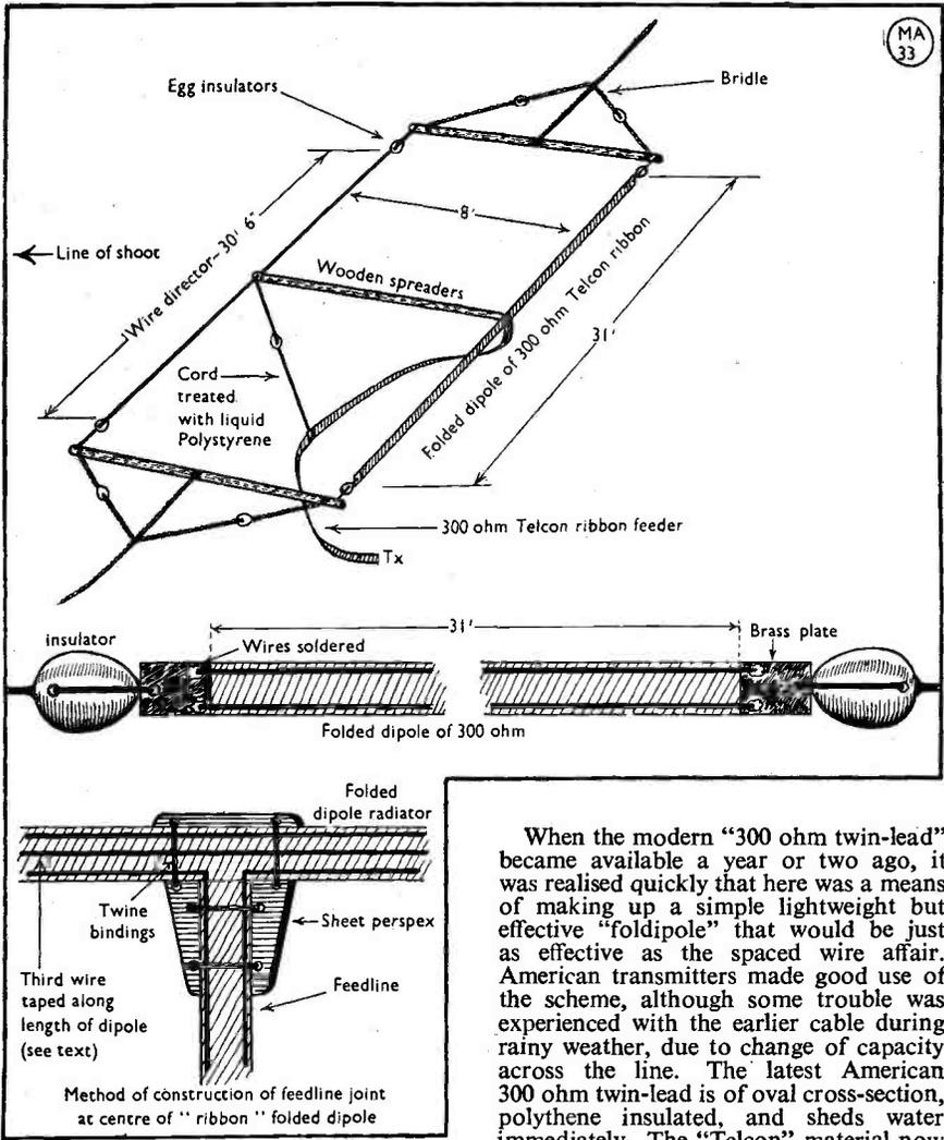
feedline tied-in at the centre of one side. The centre impedance of the two-half-wave folded dipole may be considered to be around 300 ohms. This can be raised by adding half-wave sections, but whatever the impedance characteristic, it will be obvious that an aerial made up from 14-gauge copper wire is likely to be rather heavy. If supported between poles with halyards, there may be a large degree of sag in the middle, unless poles and halyards are designed accordingly.
