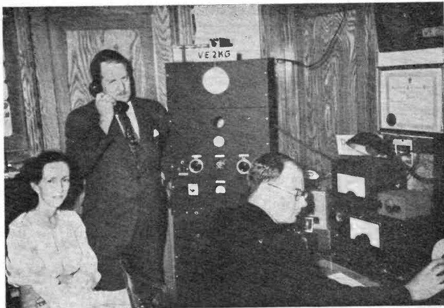
General view of VE2KG, Quebec, with ex-G2CIN at the operating position. The Tx runs 50 watts, using a 6L6-RK39 combination, into a 4-clement beam.
