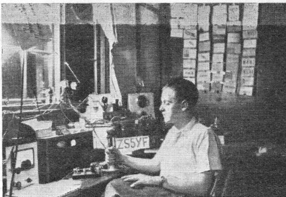
ZS5YF, Durban, is ex-G3BYF and uses a VFO 6L6-807-809 transmitter, with 50 watts input and a 138-ft. single wire aerial. The receiver is an SX-24 with two-stage preselector. He has worked 66C in 29Z; though he is always on the look-out for G's, difficulties at ZS5YF are a high local noise-level and BC receivers within a few feet of the transmitter.
