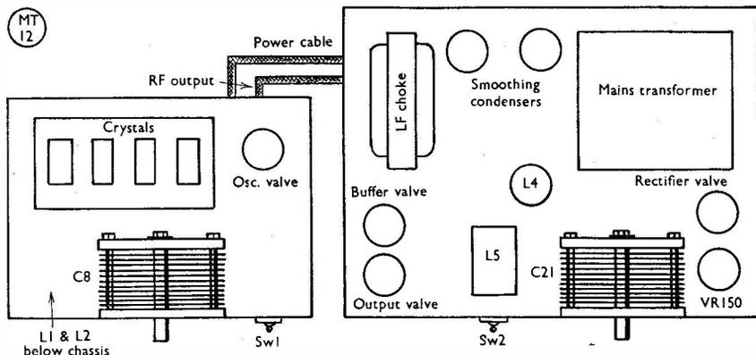
Fig. 3. Block diagram of the general chassis layout. That part of the circuit enclosed within dotted lines in Fig. 1 is in the section on the left in this drawing.
