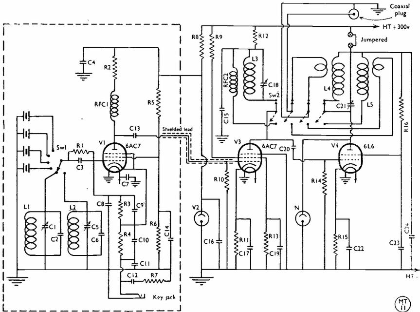
Fig. 1. Circuit of the unit complete. VFO or crystal operation can be obtained at will (SW1) and the output side is also switched (SW2). Stabilised HT supply is provided.
