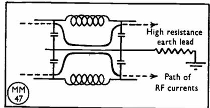
Fig. 2. Conventional mains RF choke circuit, not always effective for reasons discussed in the text.
