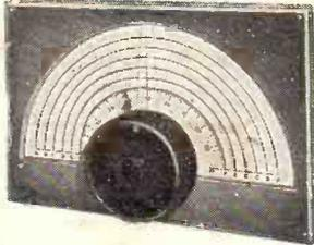
Type SMDB. A very high class Precision Slow Motion Unit for communication type equipment, frequency meters, V.F.O. units, converters, signal generators, etc., embodying a geared drive actuated by a combined direct and slow motion drive (50-1).
