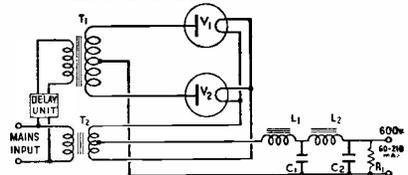
V<sub>1</sub>, V<sub>2</sub>, RG1-240A. T<sub>1</sub>, 750-0-750V/250mA.
