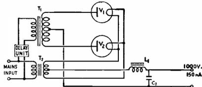
V<sub>1</sub>, V<sub>2</sub>, RG1-240A. T<sub>1</sub>, 1200-0-1200V/150mA.
