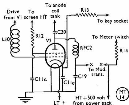
Fig. 1. Circuit of the PA side, showing how modulation can be applied. R12, 500 ohms ; R13, 200 ohms, bias ; R14, 1.2 megohms ; C11a, C11e, C19, C20, all .002  $\mu$ F ; V2, 6L6. Key sockets must be shorted on "transmit" and open on "receive."
