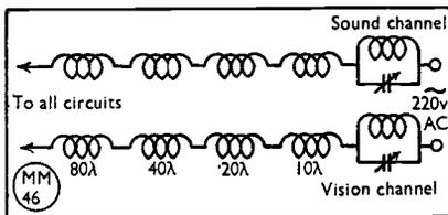
Fig. 1. Multi-band mains choke arrangement for blocking-off piped interference through the domestic supply lines.
