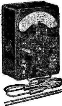
A conveniently compact 2 1/2-inch moving coil precision meter for making D.C. measurements of milliamps, volts and ohms. The total resistance of the meter is 100,000 ohms, and full scale deflection of 300 v. or 600 v. is obtained for a current consumption of 3mA. or 6mA. respectively.
