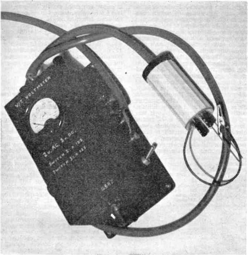
The instrument complete, with the diode probe on a wandering lead.
