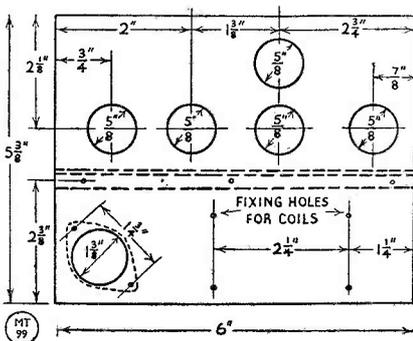
Fig. 2. Dimensioned sketch of the general chassis layout.
