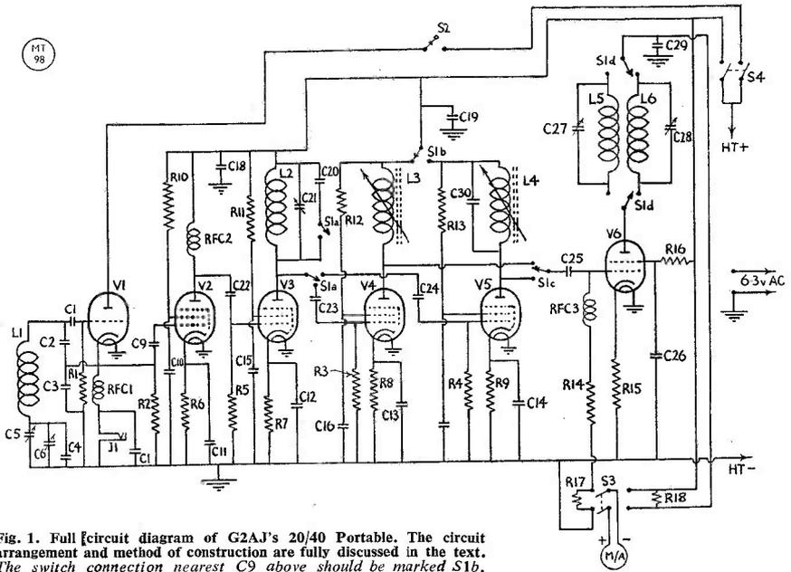
Fig. 1. Full circuit diagram of G2AJ's 20/40 Portable. The circuit arrangement and method of construction are fully discussed in the text. The switch connection nearest C9 above should be marked S1b.
