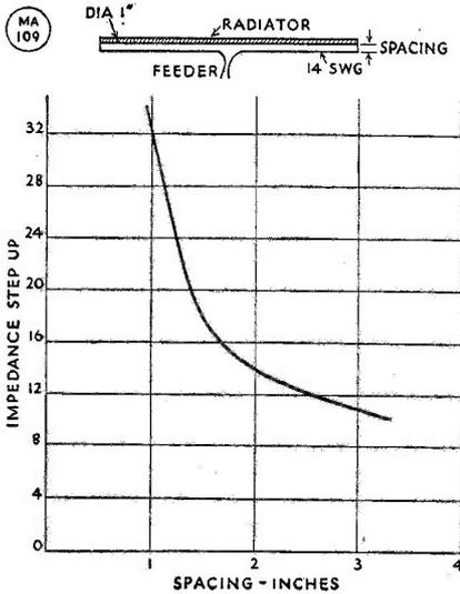
Fig. 3. Design data for folded dipole used as a radiator. As an example, for 1½-in. spacing between tube and wire the feeder impedance divided by the radiator impedance is 18, representing an impedance step-up of 18 times over a plain dipole in the same position.
