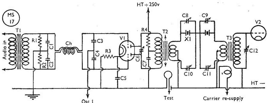
Fig. 17. Circuit of the balanced modulator—see text for discussion.
