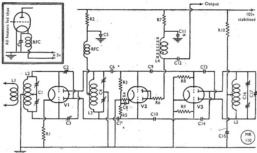
The circuit complete of G2IQ's two-metre converter, using 6J6's and with a neutralised RF section. It is a low-noise high-gain job, easy to build, and should give exceptional results on Two. The by-pass condenser C in the sketch inset can be 500  $\mu$ F.
