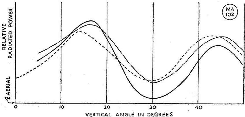
Fig. 2. Showing power distribution pattern (vertical plane in forward direction) for beam arrays adjusted as follows: 3-ele. close-spaced, maximum front-to-back ratio, dotted line; 3-ele. close-spaced, maximum forward gain, chain dotted; 4-ele. close-spaced, adjusted for maximum forward gain, solid line. In each case the height above ground is one wavelength and the element spacing 0.1 wavelength.
