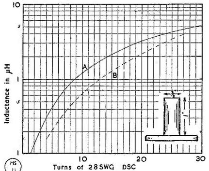
Fig. 11. Inductance wound on ex-Service type formers: A, close wound; B, turns spaced to maintain coil length 1.5 centimetres.
