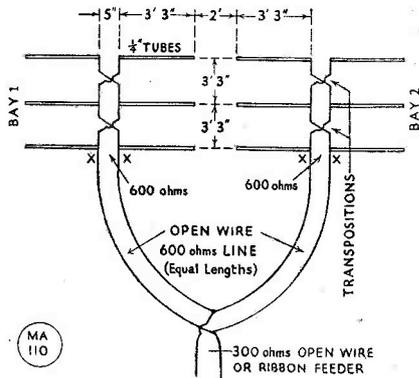
GW3ZV suggests this "Three-by-Three" for 145 mc. All elements are 39-in. of 1-in. tubing, stacked 39-in. A single bay could be used separately and fed by 600-ohm open line. Note the transposition points, also using open wire line and with connections between elements kept as short as possible. The array as dimensioned is two-way looking, giving a clover-leaf pattern broadside to the plan of the elements, and the lobes are approximately 60 deg. wide at half-power points.
