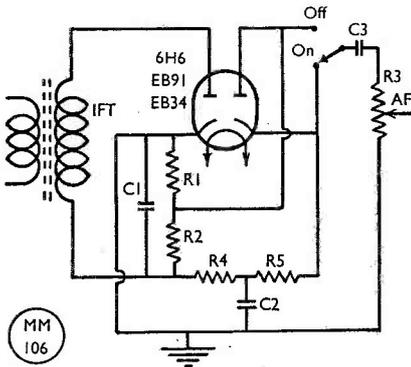
Circuit incorporating G2AKY's ideas for an effective noise limiter; details are given in the text.
