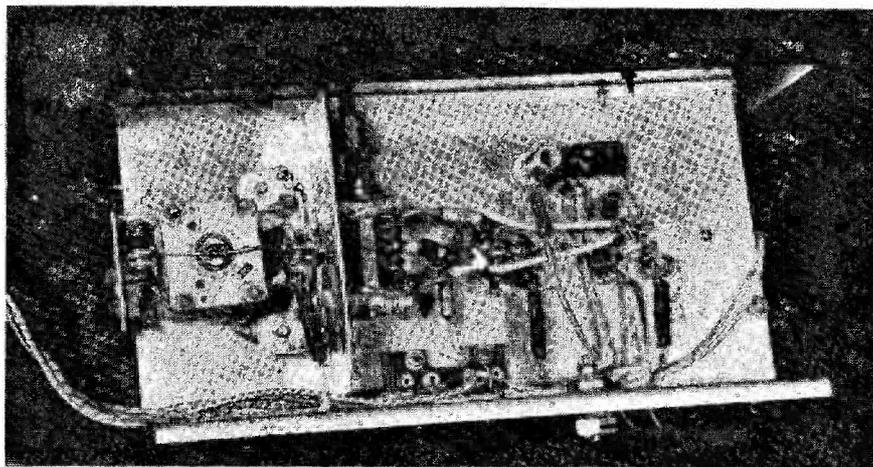
Underneath the converter constructed from surplus components. The grid coil is across the butterfly condenser, and the screen divides the grid and plate sections of the push-pull RF stage. The mixer injection condensers are the two parallel wires in the centre (white sleeving).
