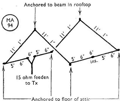
Physical layout of the indoor aerial system for 7 mc, devised by G3BQJ.
