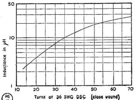
Fig. 12. Inductance on ex-Service type formers.
