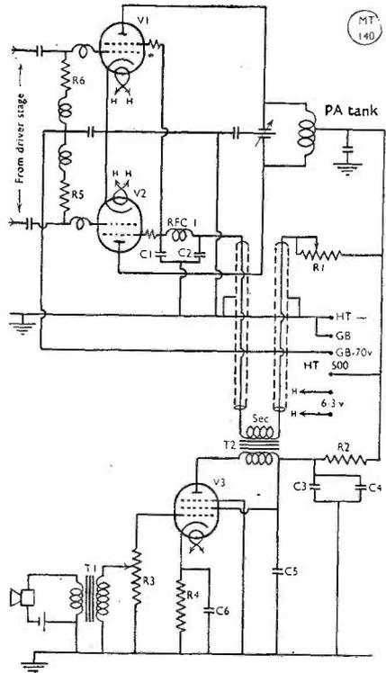
Circuit of the screen-modulated PA complete. The values given above are those affecting only the modulating system discussed by GM8BO—otherwise, the circuit follows normal practice.
