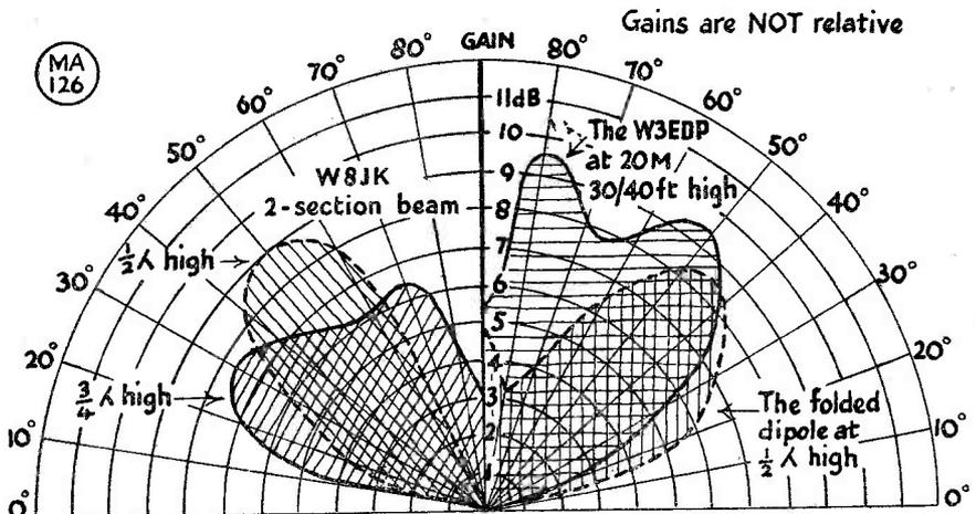
Fig. 6. Vertical radiation patterns given by some other model aerials at different heights.
