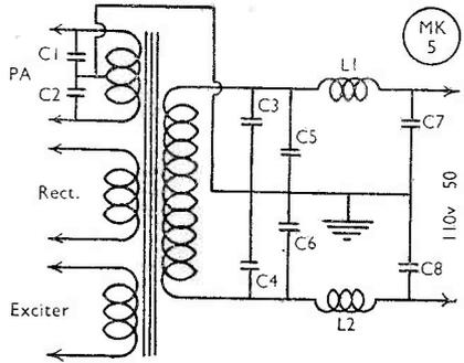
Fig. 5. TVI filter circuit for the transformer supplying LT to RF stages.
