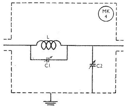
Fig. 4. Circuit of the low-pass filter, values for which are discussed in the text. (See photograph).
