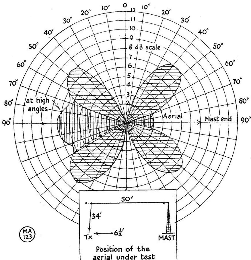
Fig. 3. An analysis of the horizontal radiation pattern of the W3EDP cut for Twenty, and at a height of 40-ft. with the counterpoise at right angles to aerial. (Layout inset).
