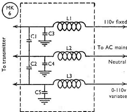
Fig. 6. Suitable mains filter for the HT4E transmitter, but applicable to the supply unit for any other type of transmitter.
