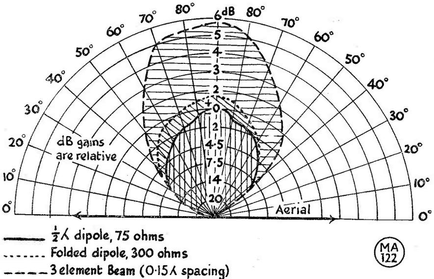
Fig. 2. Some horizontal polar diagrams with aerials at half-wave height. The reference frequency is 144 mc, but the argument is that by the Theory of Similar Structures, the same sort of pattern would be obtained for a similar aerial on the lower communication frequencies.
