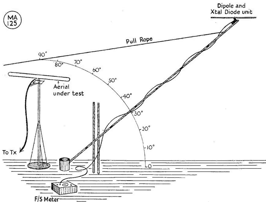
Fig. 5. Arrangement devised by G2BCX to plot vertical patterns. The reference aerial is on the tripod and fed with power from the transmitter on 144 mc. The test aerial connected back to the field-strength meter is swung on the counter-weighted rod. Comparative readings can thus be obtained through all vertical angles.
