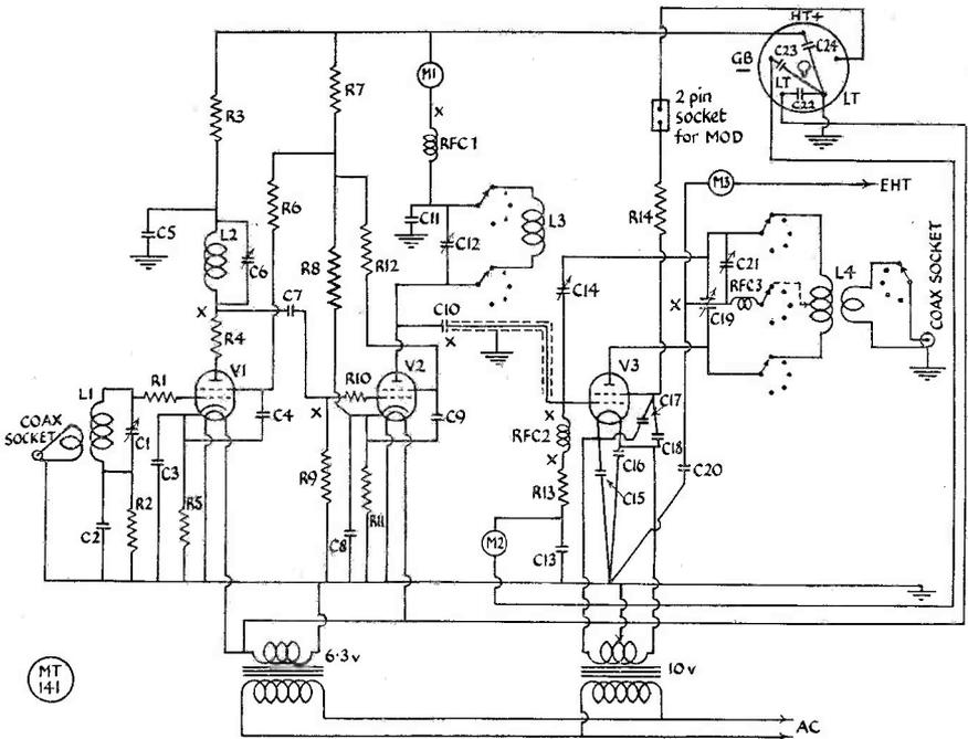
Fig. 1. Circuit of the Band-Switch QRO Transmitter, discussed in detail in the text. For simplicity, one set of coils only is shown across the band-change switches. The switching is integral with the recommended coil assemblies, designed to cover all bands 3.5 to 28 mc inclusive.
