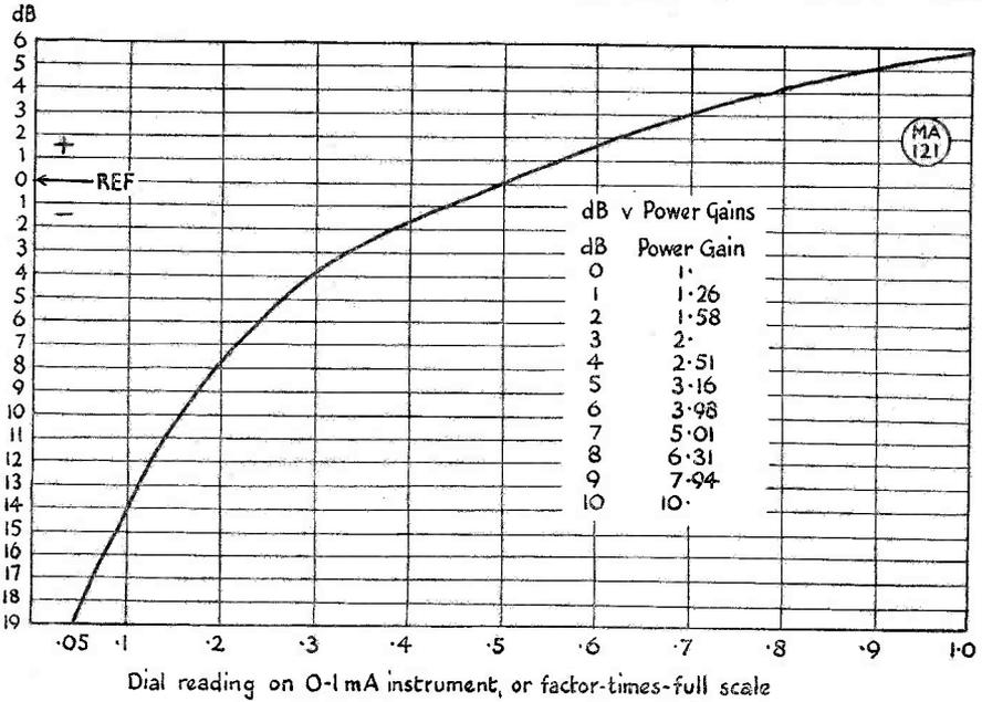
Fig. 1. Curve showing relationship between power and meter readings, as used in the experiments described
