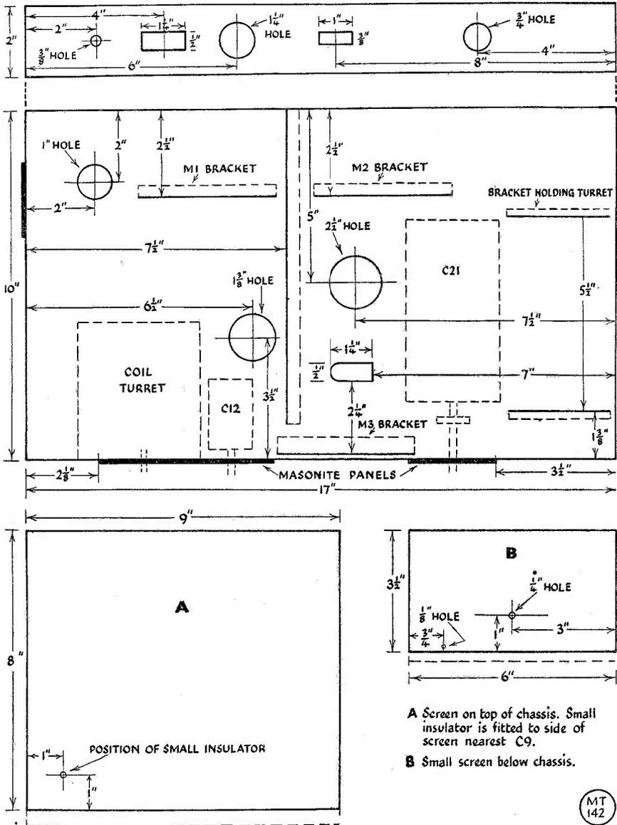
Fig. 2. Chassis and screen constructional detail. Piece "A" is the screen above the chassis, with a small insulator fitted on the side nearest C12. Piece "B" is the under-chassis screen. These details should be compared with the accompanying photographs of the finished job.
