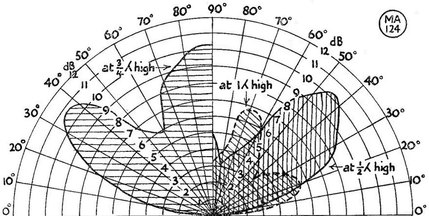
Fig. 4. Some vertical polar diagrams for aerials at half-wave, three-quarter-wave and full-wave in height. The aerials are actually dipoles on 144 mc, and in this diagram the gains are not relative except in the case of those at half-wave and three-quarter-wave in height.
