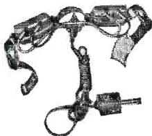
Pair of electro-magnetic throat pieces (coil resistance 7.5 ohms), with lead and jack plug.
